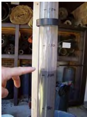
c) Incremental slurry position within column
