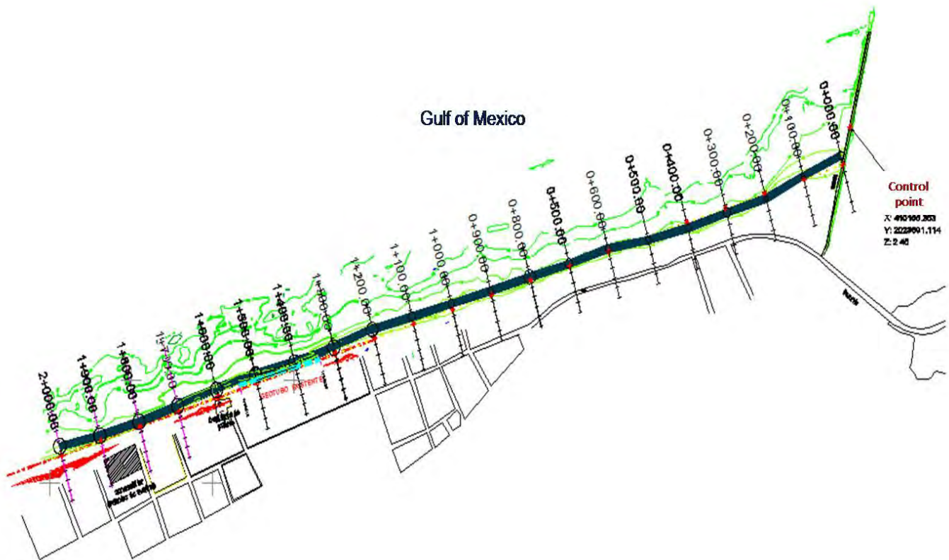
Figure 6. There were installed 77 Geotextile tubes to attain the total longitude of 2,303.85 linear meters from the existing breakwater to the local cemetery along all the coastal line.
