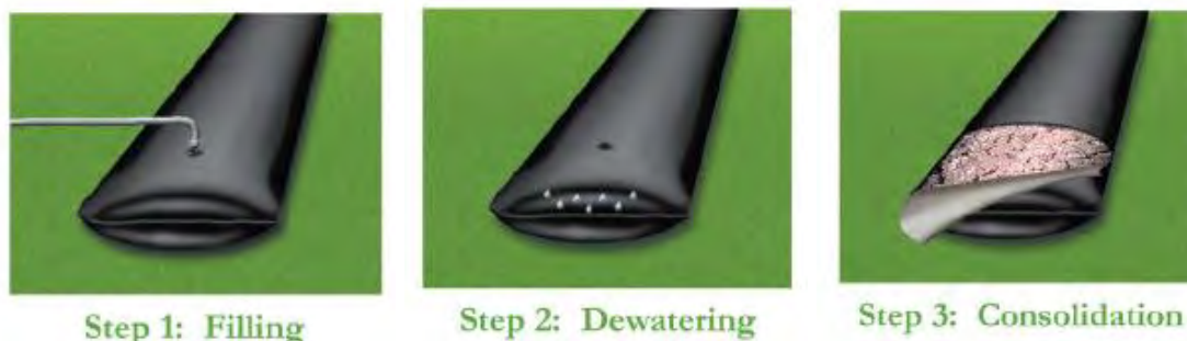
Figure 1. Three basic stages of geotextile container dewatering.
