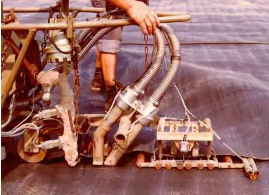
Figure 6. Schlegel Lap welding machine (courtesy Catrin Tarnowski).
