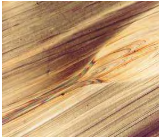
Figure 12. Thin slice cross section at root of squeeze-out bead in a fusion weld viewed with crossed polarizing filters.
