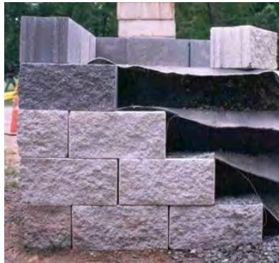
Figure 1. Cross-section of fully frictional connection.
