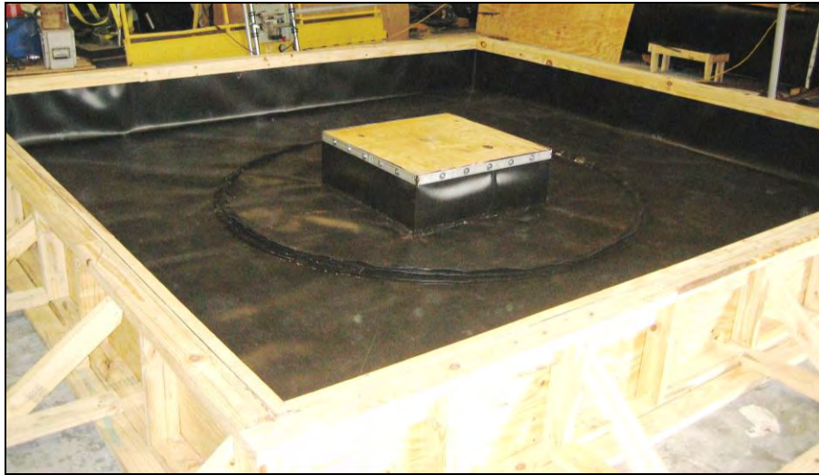
Figure 3 – Prototype boot in test box without gravel layer
