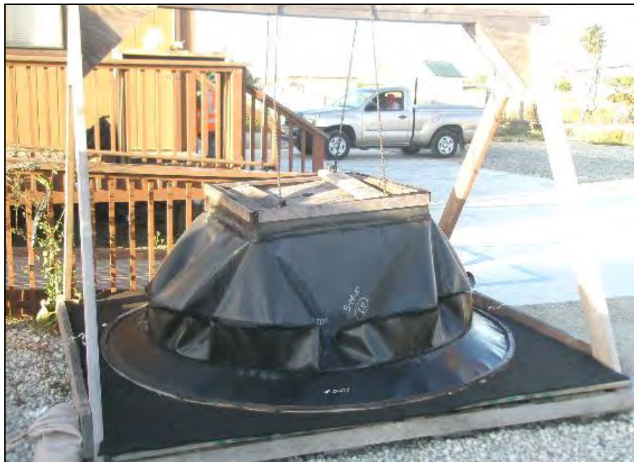
Figure 9: Single flap boot on display at the site since April 2010; extended to compensate for 76 cm of settlement.
