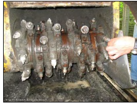
Figure 9. Virtually no fibers on the milling drum
