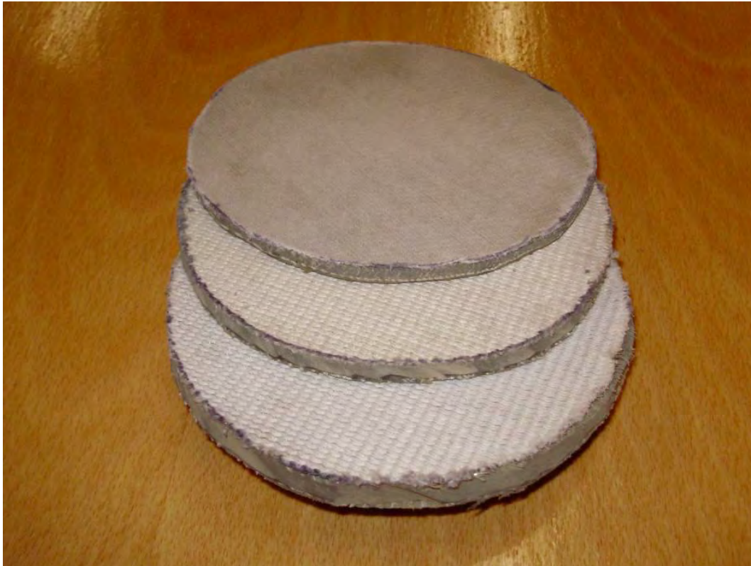
Figure 2 - Samples of Hardened 5mm, 8mm and 13mm thick GCCM, with fabric side showing (side with PVC attached is down).
