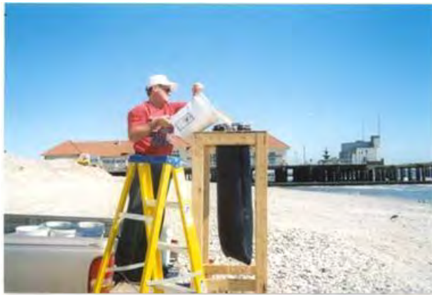
a) Sand slurry being placed in a hanging bag
