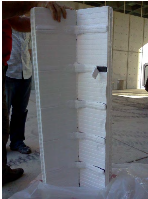
Figure 9. Exhumed ICF after full scale ICF-pipe test
