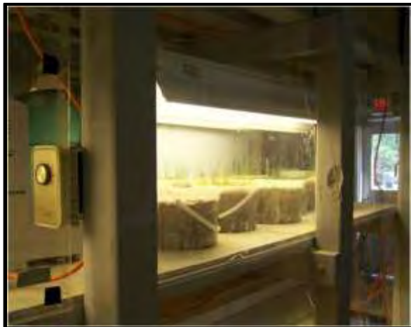
Figure 21 - ASTM D 7322 Germination Testing
