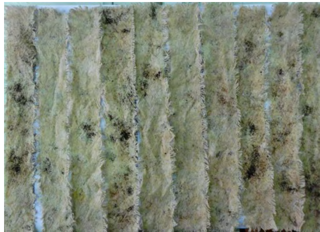
Figure 2. Picture of 7-day incubated cotton strip samples (significant rot was observed).
