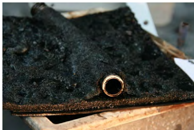
Figure 11. Side view of the geocomposite in cell 7 (type A).
