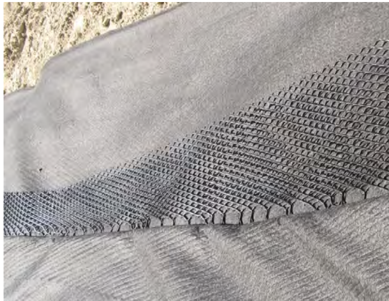
Figure 6. Melted geonet at the edge of a geonet composite roll.
