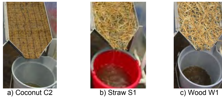
Figure 4. Photographs of the ECBs (C2, S1, W1) during a rainsplash test.
