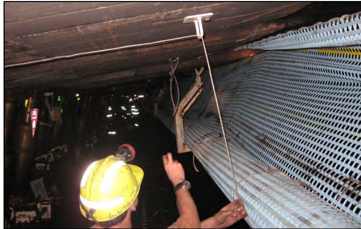
Figure 13: USA and Australian Coal Mines working with Longwall method mining are using geogrid how surface control in underground mines .
