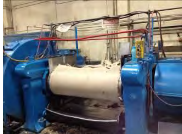
Figure 6 and 7: Feeding CSPE into the two-roll mills. Mill #1 on left, Mill #2 on right. Tan CSPE shown.
