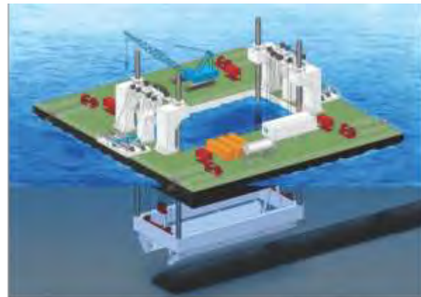
c) Geotextile container installation barge
