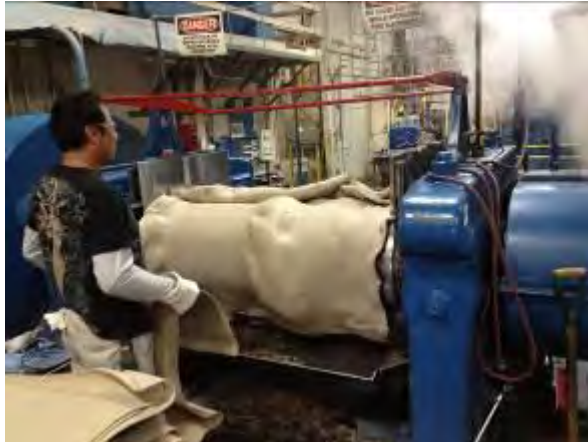
Figure 6 and 7: Feeding CSPE into the two-roll mills. Mill #1 on left, Mill #2 on right. Tan CSPE shown.
