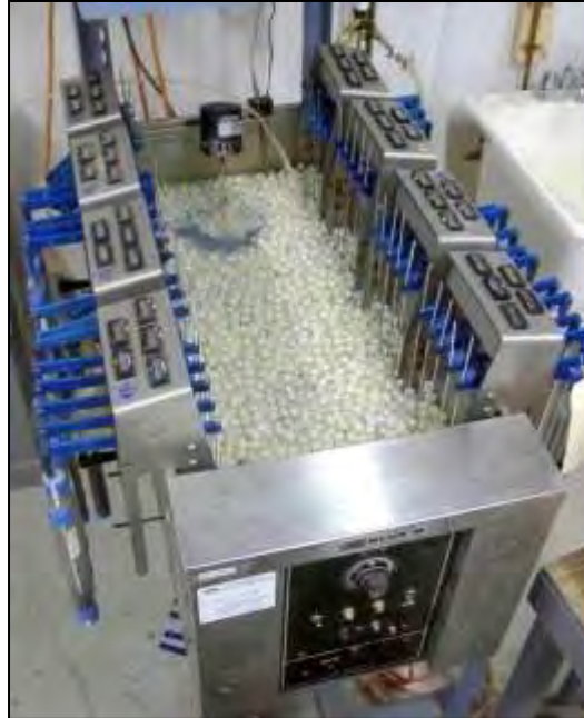
Figure 2: ASTM D 5397, Appendix – Notched Constant Load Stress Crack Testing
