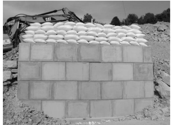
Figure 8. Wall with 1.5m overburden load (~30kPa)
