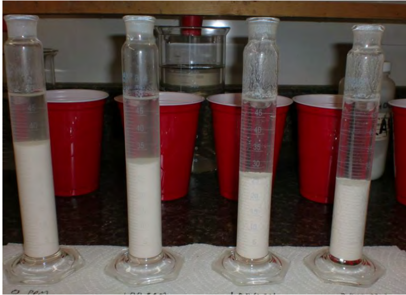
Figure 2. The Flocculation Method, presence of polymer increases settling rates
