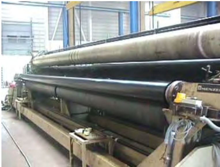
(d) winder is part of a flat die production facility although it could just as well be used for round die production.
