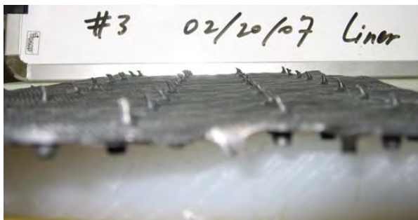
c Spikes Bent in the Downslope Direction
