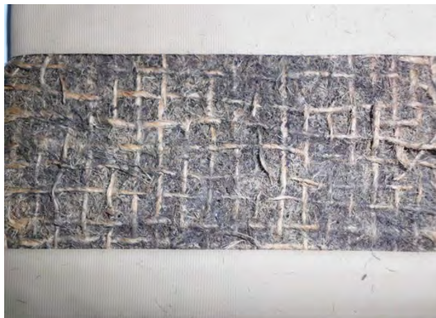
Figure 4. Picture of 14-day incubated jute fabric samples (sample woven structure was damaged).
