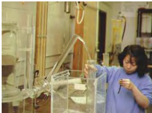
(d) Colleague Grace Hsuan performing a permittivity test
