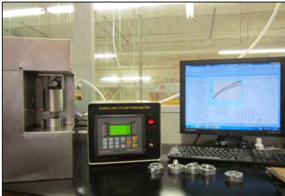
Figure 6: ASTM D 6767 PSD Test Apparatus
