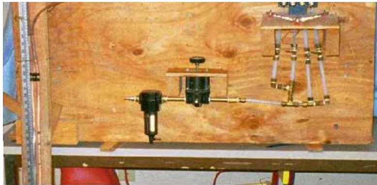
Figure 2. (a) Schematic diagram, and (b) photograph of the bubble point test equipment (from D'Hondt, 2005).
