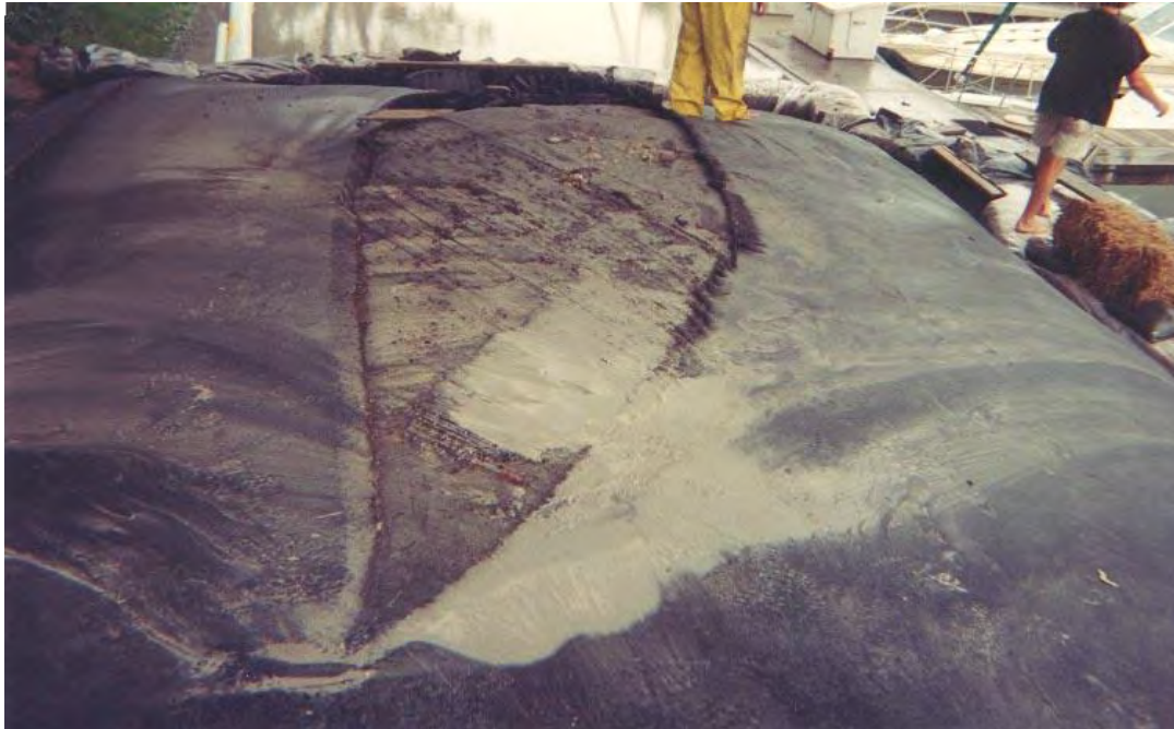
Figure 5. Controlled failure of tube.
