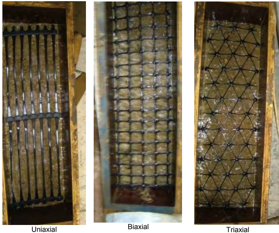
Figure 3. Placing of the geogrid layer after pouring and compacting of the 5 cm concrete layer
