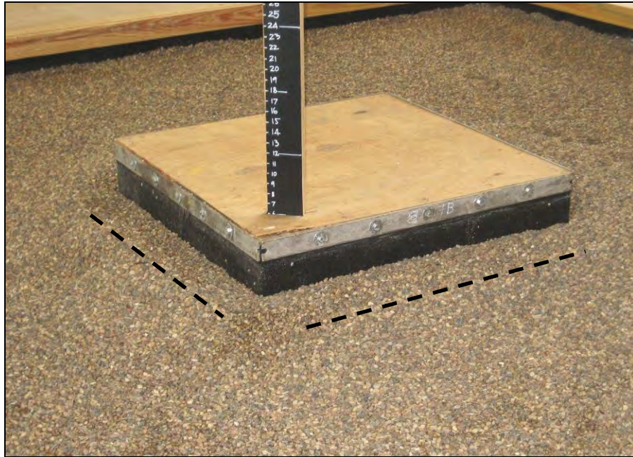
Figure 5 – Typical behavior of boot displacing 30 cm gravel layer upon differential settlement of 15 cm (approximately the maximum estimated remaining settlement of 17 cm). Dashed line added to show approximate location of base of cone of displaced gravel.
