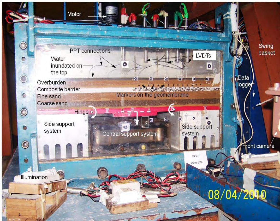
Figure 1. Model test package for centrifuge tests
