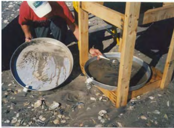
c) Fine sediment ( \leq #200 sieve) carried in the escaped effluent
