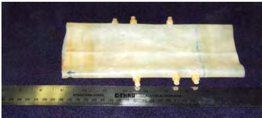
Figure 8. FWGR 71 mm diameter latex membrane with pressure ports.
