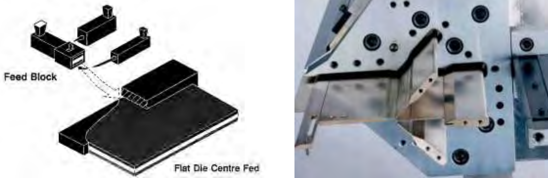
Figure 3. Die configuration for a three layer flat die web.
