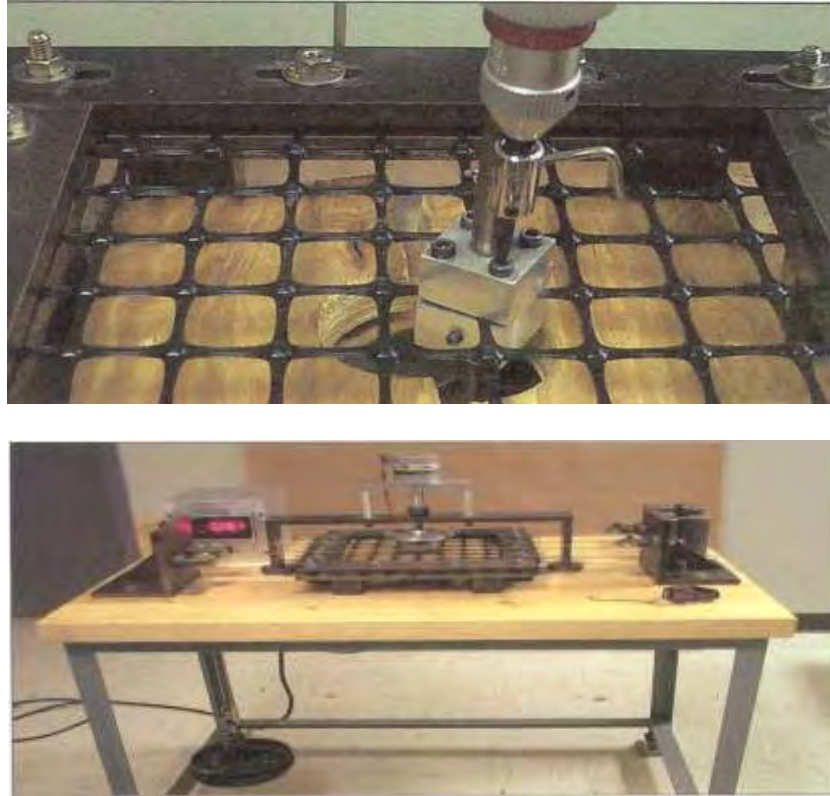
Figure 15. Plan and elevation view of the test apparatus for in-plane torsional rigidity determination of bidirectional geogrid stiffness per Kinney (1998) and GRI-GG9 test method (2004).
