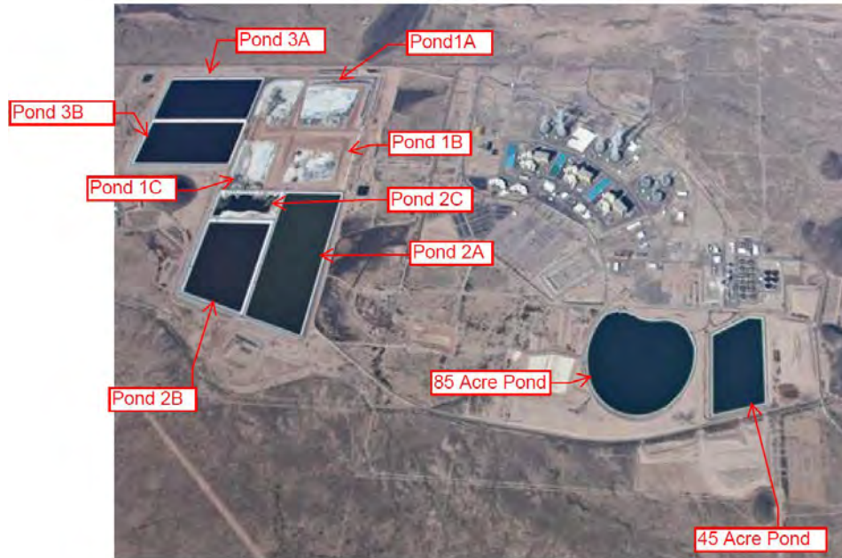
Figure 2. Aerial view of the lined containment reservoirs for municipality wastewater and Evaporation Ponds. The 85-acre and the 45-acre reservoirs are shown above.
