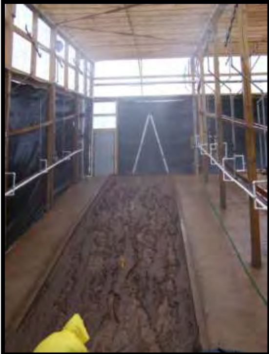
Figure 24 - ASTM D 6459 Slope Testing
