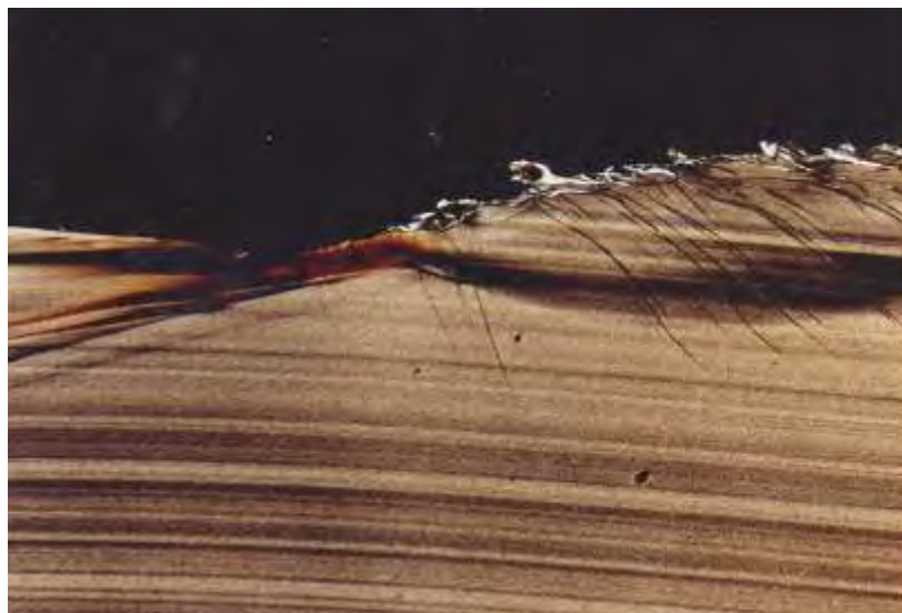
Figure 13. Crazes initiated in peel separated surface (arrowed). Squeeze-out bead to left.
