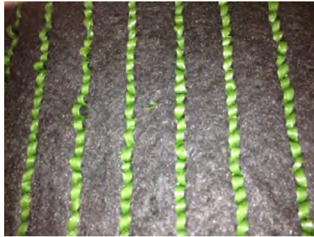
Figure 5. Back of synthetic grass tufts in nonwoven geotextile.
