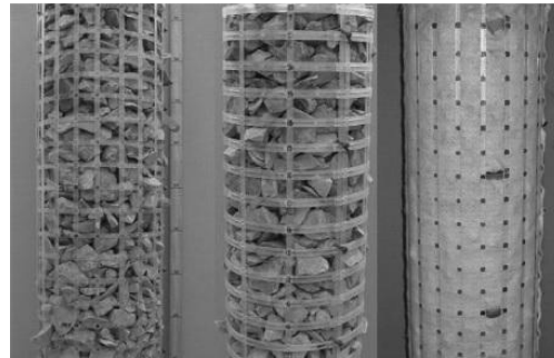
FIGURE 3 – Medium-scale testing with columns encased by two types of geogrid and one geocomposite performed by Gniel & Bouazza (2010). Extracted from Gniel & Bouazza (2010)
