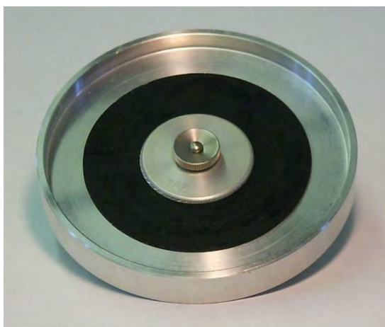
Figure 3. Reconfigured specimen holder so as to provide for saturated conditions.
