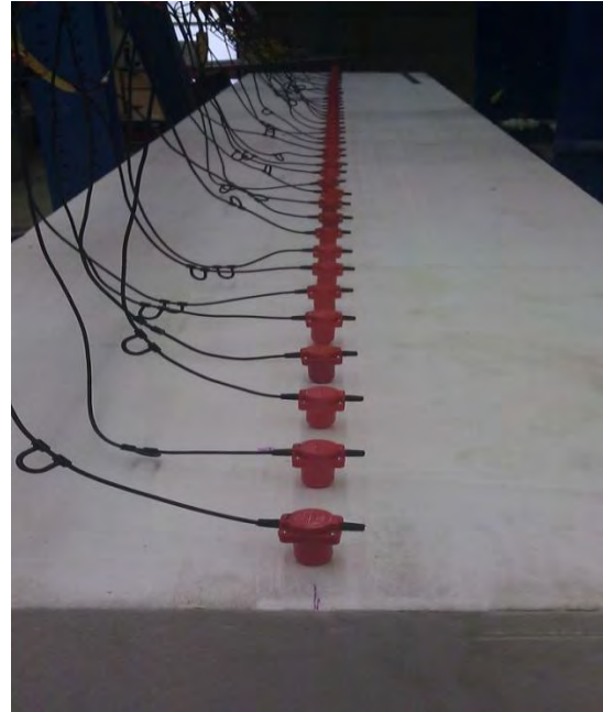
Figure 4. Large scale EPS block under MASW test at the University of Memphis Geotechnical Lab.
