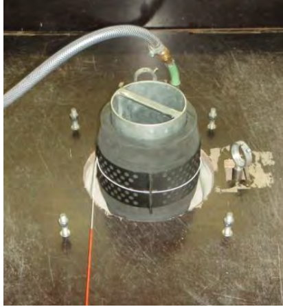
Figure 7. Installed geocell on air pressure bag and connected strain measurement system
