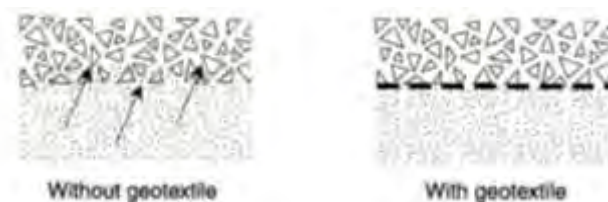
(a) Mechanism of fine soils pumping into stone base voids and prevention using geotextiles
