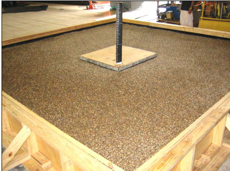
Figure 4 – Prototype boot in test box with 30 cm gravel layer
