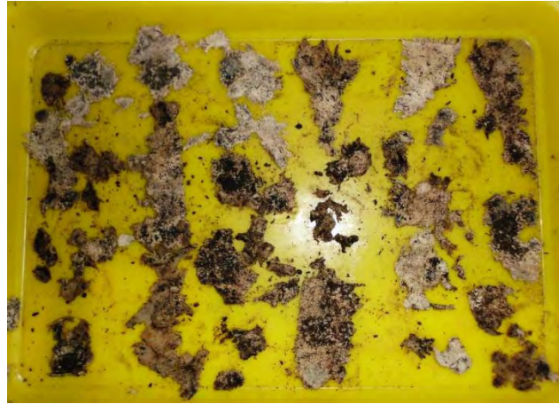
Figure 3. Picture of 14-day incubated cotton strip samples (samples were completely destroyed by rot).
