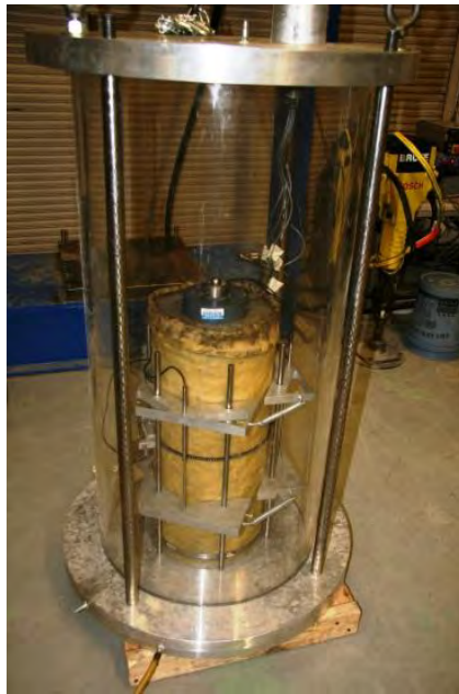
Figure 1. Compacted ballast specimen with instrumentation assembled inside the acrylic chamber ready to be tested using the University of Illinois Triaxial Ballast Tester (TX-24)
