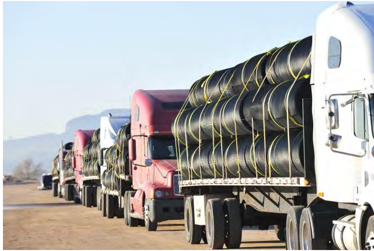
Figure 10 – Delivery of geonet drainage material
