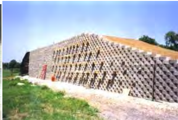
Figure 5. Louisiana Transportation Research Center (LTRC) Test Wall Built with Silty-Clay Reinforced Fill over Soft Soil
