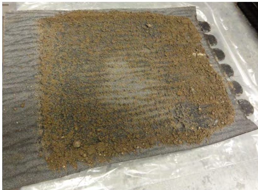
Figure 8. Thick soil film retained on BGM/Fill Interface after testing (non-saturated condition).
