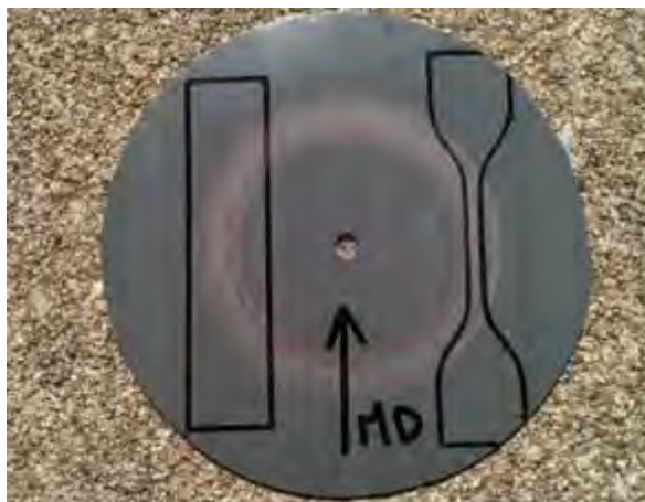
Figure 2. Abraded specimen with tensile test outlines for strength and elongation retained properties.
