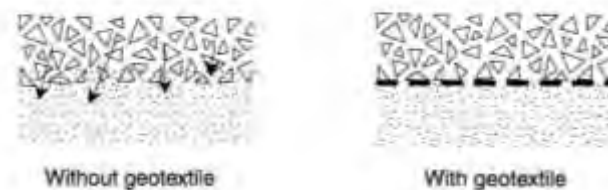
(b) Mechanism of stone base intrusion into fine soil subgrade and prevention using geotextiles
