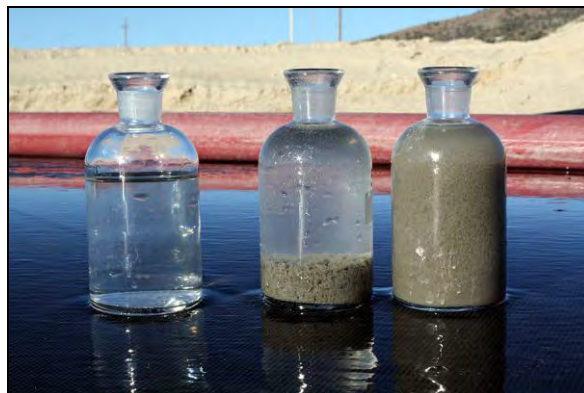
Figure 3. Results of dewatering with geotextile containers showing filtrate, conditioned slurry, and in-situ slurry.
