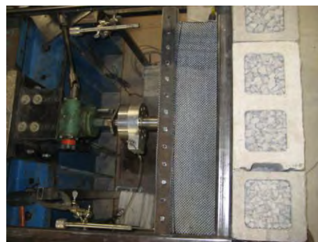
Figure 5. TFHRC Frictional Connection Test with Hollow Core CMUs Infilled with No. 57 Aggregate.
