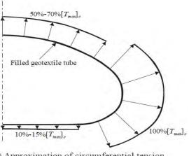
b) Approximation of circumferential tension distribution in terms of [*T<sub>max</sub>*]
