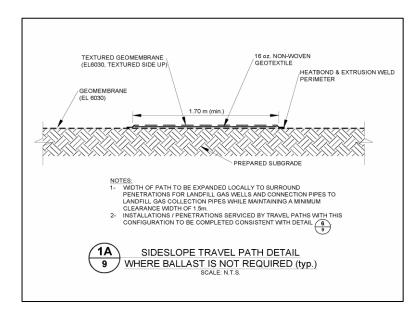
Figure 10 Sideslope Travel Path Detail
