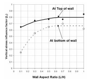
Figure 5. Vertical stress influence factors at the top and bottom of the wall (Kniss et al., 2007)
