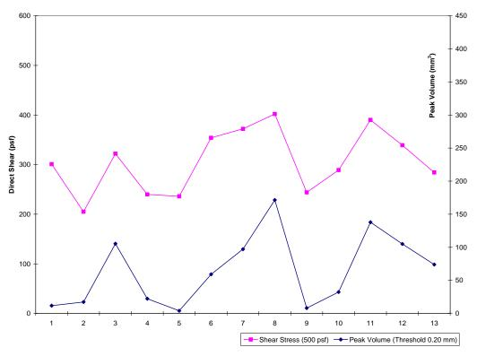
Figure 12. Chart of Direct shear vs. Peak Volume (0.20 mm threshold) by sample.
