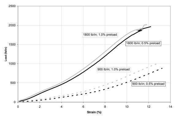
Figure 2. 4-inch Wide, 0.5 and 1.0% Preload, Avg of All Specimens - Lab #1
