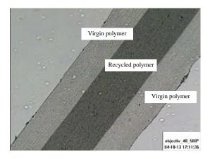
Figure 4: Microscopic section of a HDPE drainboard including a layer of recycled resin
