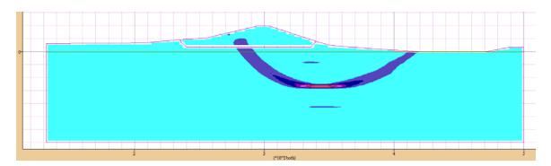
Figure 4. Failure surface without geotextile and without water. FOS = 1.33.
