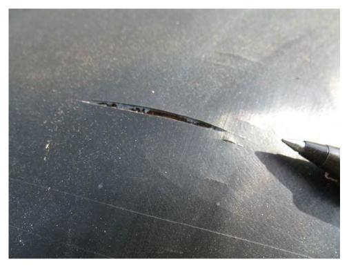
Figure 2 Stress cracks initiated at extrusion die line above protruding subgrade stone
