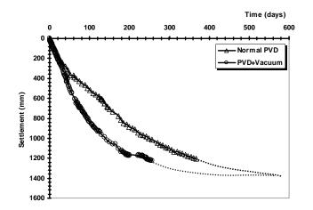
Figure 9. Comparison of settlement of PVD improvement with and without vacuum preloading (Sta. X=14012, Y=12567-12633 for PVD with embankment and Sta. X=12566.4, Y = 12570.000 for PVD with vacuum preloading)
