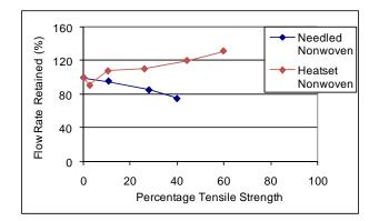
Figure 13. Flow rate retained versus percentage ultimate tensile strength of two nonwoven geotextiles
