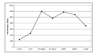
Figure 6. Tear Strength Properties (ASTM D624, Die C).
