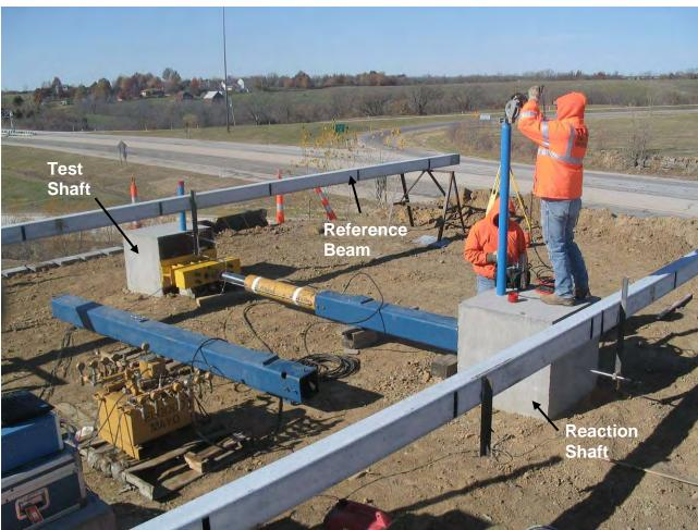
Figure 3 Test apparatus including hydraulic pump and cylinder, load cell, reference beams, LVDTs, and inclinometer.
