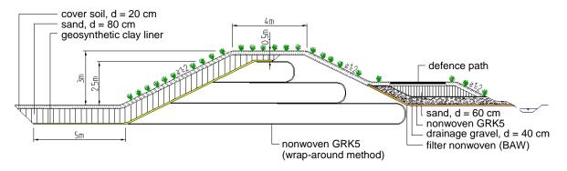
Figure 9. Cross-section of a reconstructed Oder River levee in Poland (Heerten 1999)
