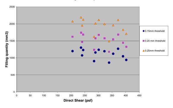
Direct Shear vs. Filling Quantity at various thresholds
