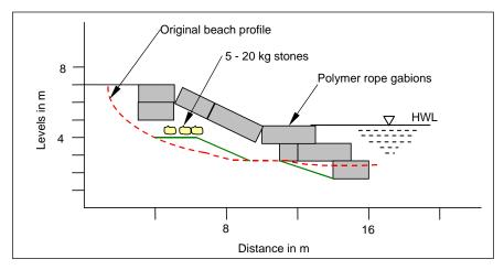
Figure 7. Schematic of the section showing anti-sea erosion bund at Swaminarayan temple.
