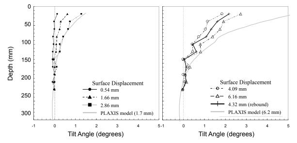
Figure 7. Rotation angle at the plate edge as a function of depth and applied surface displacement without geogrid reinforcement. PLAXIS modeling results are shown at two surface displacement levels for comparison.
