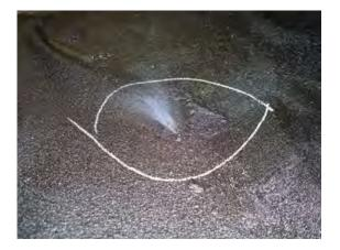
(c) Marked presence of smoke in a defect in a thin section of geomembrane
