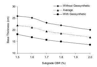
Figure 3. Relationship of CBR to base course thickness
