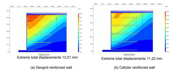
Figure 11. Extreme total displacement shedding plot
