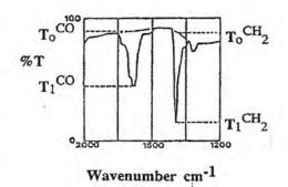
Figure 6. Calculation of Carbonyl Index (Broutman and Duvall, 1989)
