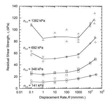
Figure 5. Effect of displacement rate on residual shear strength for monotonic shear.
