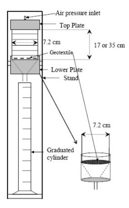
Figure 1. Schematic of Falling Head Test and Pressure Filtration Test Apparatus.
