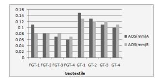
Figure 12. AOS of nanoclay formulated and standard polyester nonwoven geotextiles before/after immersion. (Where A, B mean before and after immersion, respectively)
