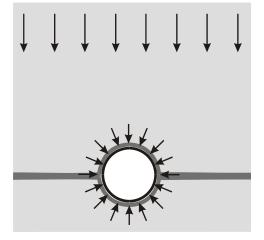
Figure 3: pipe loading mechanism
