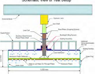
Schematic View of Test Setup
