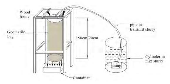
Figure 2. Hanging Bag Test Set-Up.
