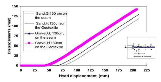
Figure 7. Displacement of the points located at 130 cm length of the geocomposite sample.
