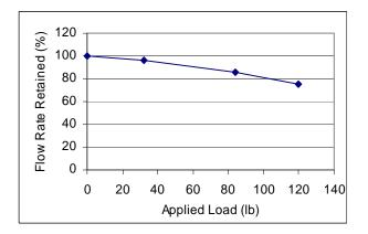
Figure 5. Flow rate retained versus applied load of the needle-punched NW geotextile.
