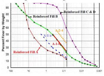
Figure 3: Gradation of the Backfill Soils
