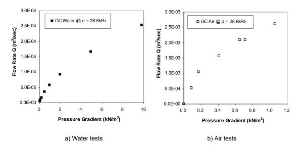
Figure 7 Linear-flow rate of geocomposite vs. pressure gradient
