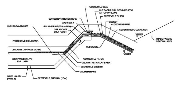
Figure 4. Lining system after dismantlement of batten strip anchor.
