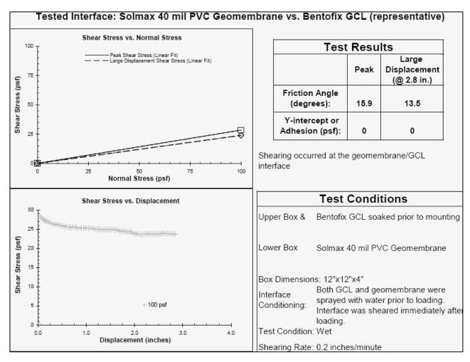
Figure 6. Direct shear test results: Interface sprayed with water before test assembly.
