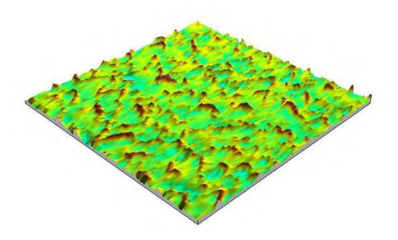
Figure 1. Three dimensional topological characterization of a textured geomembrane.
