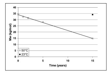
Figure 8. Molecular weight evolution with time for PET yarns exposed to deionized water at 50°C and 23°C during 15 years.
