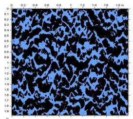
Figure 4: 3D topological characterization of a textured geomembrane (zero plane threshold)
