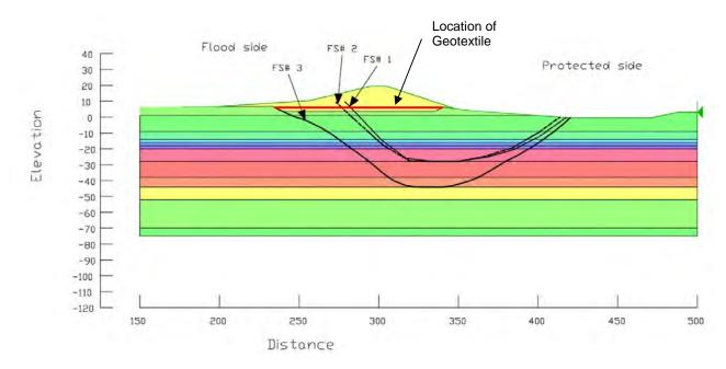
Figure 3. Limit equilibrium failure surfaces. FS# 1 = failure surface without geotextile and without water, FOS = 1.26. FS# 2 = failure surface without geotextile with WL = 19.5 ft, FOS = 1.22. FS# 3 = failure surface with geotextile with WL = 19.5 ft, FOS = 1.23.
