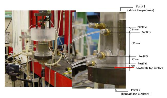
Figure 2. Permeameter cell and port arrangement on the side wall
