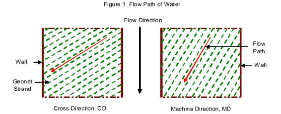
As shown in Figure 1, the CD (Cross Direction) geonet channels, direct the water flow into the wall; whereas the MD (Machine Direction) geonet channels, primarily direct the water flow out of the drainage end of the transmissivity apparatus. This investigative study attempts to estimate the fraction of turbulence contributed by the geonet strands that direct the water flow into the wall of the transmissivity apparatus as measured by flow rate loss caused by the side walls.
