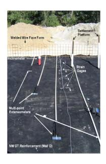
Figure 5: Instrumentation for Each Test Wall
