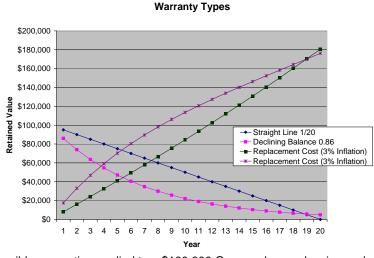
Figure 5 Possible warranties applied to a \$100,000 Geomembrane showing replacement costs
