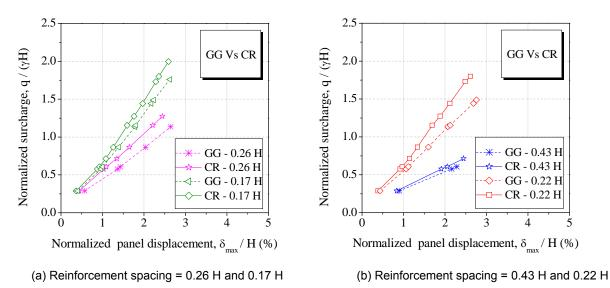
Figure 7. Comparison between geogrid (GG) and cellular reinforced (CR) wall for surcharge pressure versus maximum panel displacement
