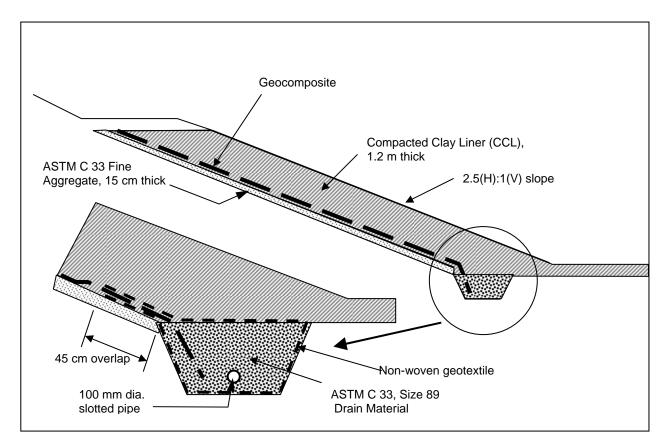
Figure 3. Geocomposite drain details (not to scale).
