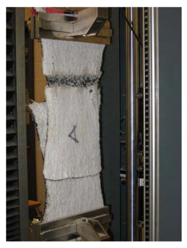
Figure 9. Tensile failure of specimen by pre-engineered groove.
