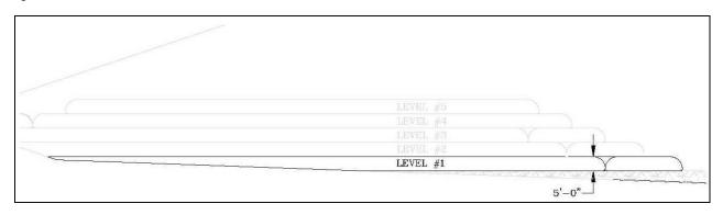
Figure 2. Cross section of the first layer of geotextile tubes, used to level the CF floor (the leveling layer).
