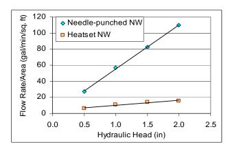
Figure 3. Changes in flow rate per area with hydraulic head for two types of nonwoven geotextiles.
