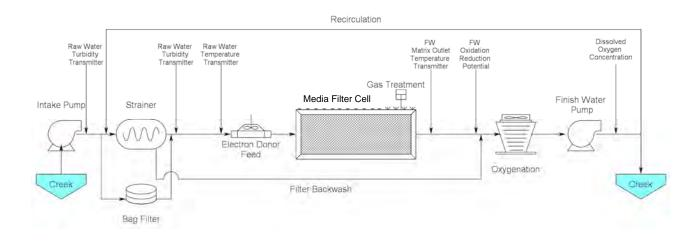
Figure 3. Schematic of subsurface treatment system
