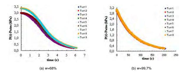
Figure 5. Variation of the gas pressure with time for the GCL samples (Pitanga et al., 2008).
