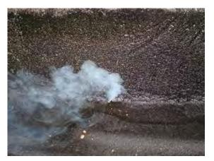
(d) Smoke plume seen at inadequate geomembrane foundation connection
