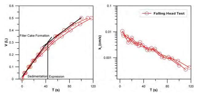
Figure 3. Falling Head Test Results.
