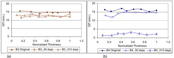
Figure 5. OIT profiles of B3 and B4 at 85°C incubation temperature
