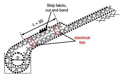
(b) Drainage pipe in a trench
