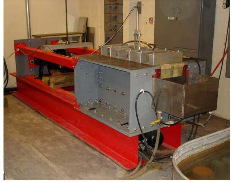
Figure 1. Dynamic direct shear machine.
