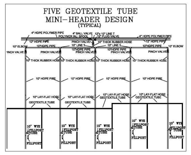
Figure 1. Typical mini-header design.
