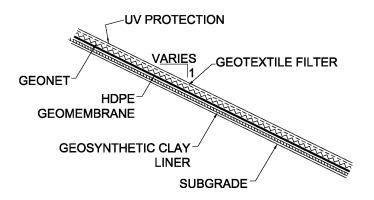
Figure 1. Side slope lining system
