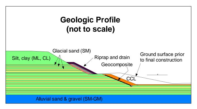
Figure 1. Schematic view of geologic profile.
