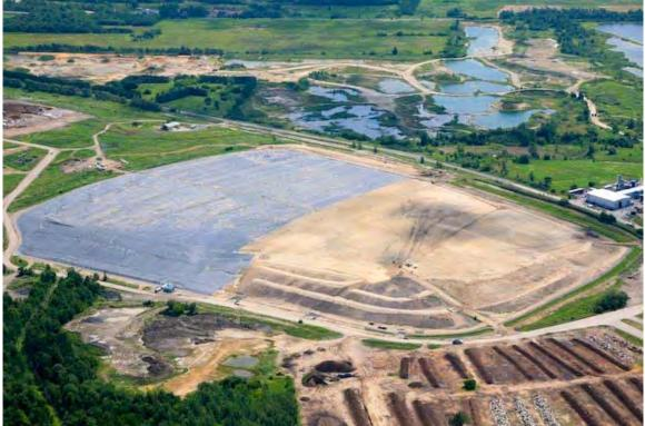
Figure 1 Landfill Cap Under Construction
