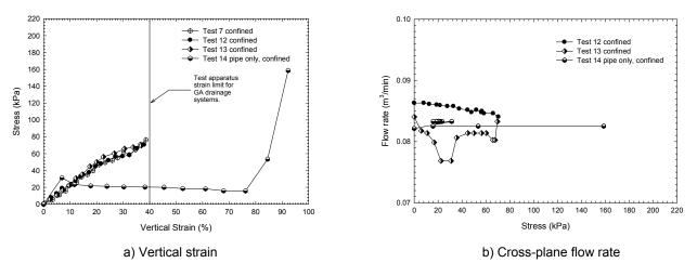
Figure 12. Test results between GA drainage systems with pipe and a stand-alone (bare) pipe.
