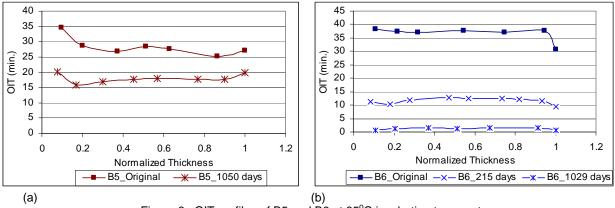
Figure 6. OIT profiles of B5 and B6 at 85°C incubation temperature
