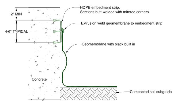
Figure 13. Basic concrete embedment strip elements.
