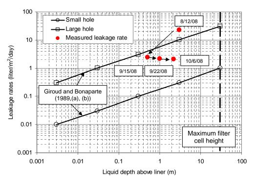
Figure 10. Decrease in leakage rate (8/12/08 to 9/15/08: tear repairs at the west end; 9/15/08 to 10/6/08: clamp repairs)
