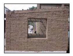
Figure 5.Non plastered side and plastered side after testing.
