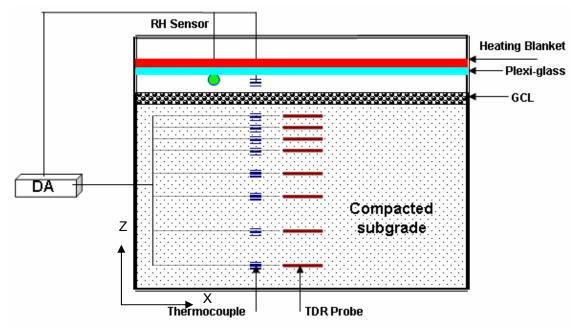
Figure 6: Schematic instrumentation details of the big-box model
