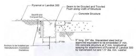
Figure 10. Transition detail of a woven HPTRM to a concrete channel.
