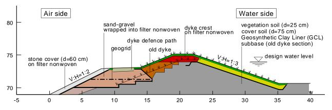
Figure 1. Standard cross-section of a reconstructed Elbe levee near Bösewig / Sachsen-Anhalt (Heerten et al. 2006)
