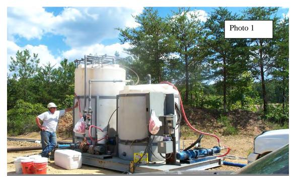
The treatment plant utilized an anionic flocculation polymer and a cationic coagulant polymer to treat the slurry before it was pumped into the bags. (Photos 2 and 3)
