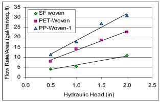
Figure 4. Changes in flow rate per area with hydraulic head for three types of woven geotextiles.
