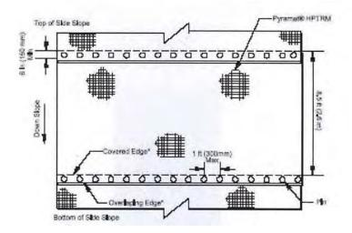
Figure 4. Pyramats® HPTRM overlap at roll edge detail.
