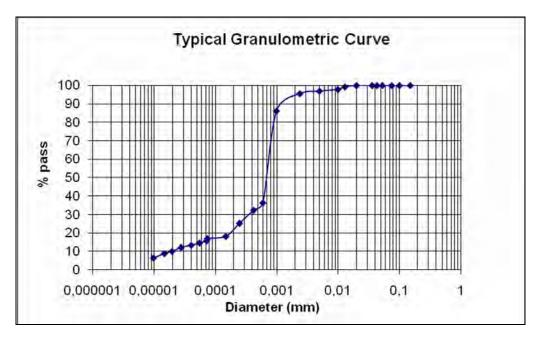
Figure 6 – Typical granulometric curve of Sediment A.
