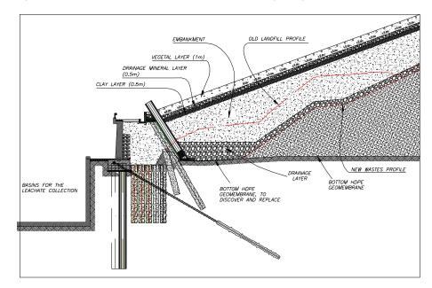
Figure 4a Section at the toe of Scarpino, before the beginning of the stabilization works
