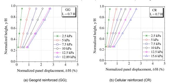
Figure 5. Relationship between normalized wall height and normalized panel displacement at various applied surcharge pressures for the reinforcement length of 0.7 times height of wall
