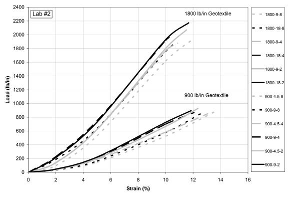
Figure 7. All Widths and Preloads – Avg of All Specimens – Lab #2
