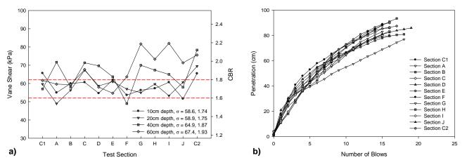
Figure 13. Average strength of artificial subgrade after trafficking: a) vane shear, b) DCP.
