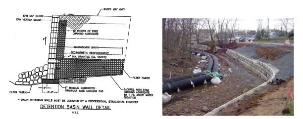
Figure 4. Detention basin wall or wall along drainage channel.
