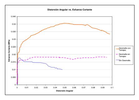
Figure 8. Comparative evolvement curves of plain, reinforced without plaster and reinforced and plastered walls in shear test.
