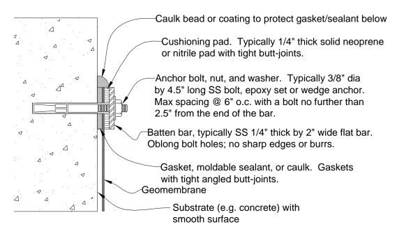
Figure 10. Schematic of typical batten bar elements.
