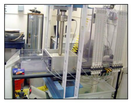
Figure 2. Photograph of a hydraulic transmissivity test apparatus.
