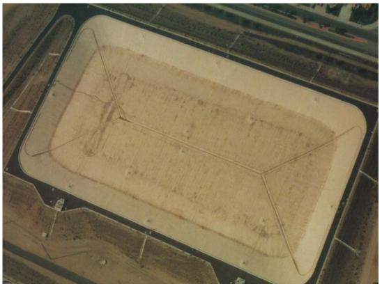
Figure 1 – Overhead view of a ballast and float defined sump tensioned cover system
