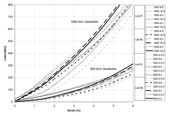
Figure 12. Close-up of Low Strain Region - Avg of All Specimens - Labs #1 & #2
