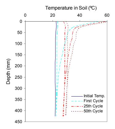
Figure 8: Temperature profile for heat/cool cycles in subsoil
