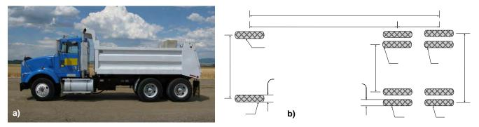
Figure 10. Three-axle dump truck used for trafficking: a) side view of vehicle, b) axle dimensions and associated weights.
