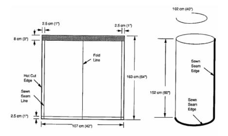
Figure 2 - Geotextile before and after preparation (Koerner & Koerner, R. M., 2006).
