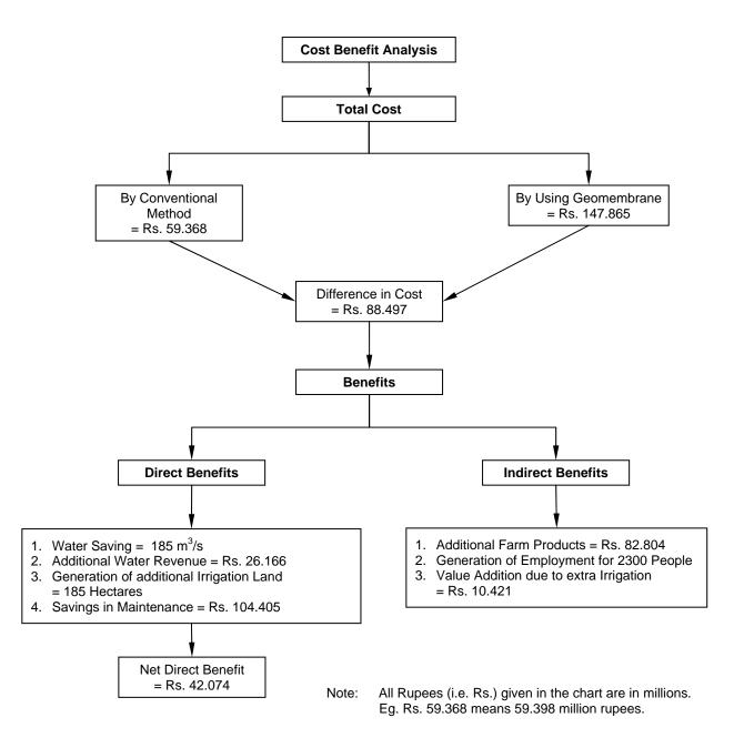
Figure 7. Flow chart showing the Cost Benefits of Geomembrane Lining in Doodhganga Canal.
