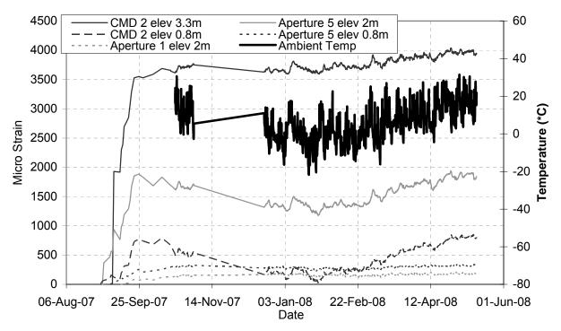
Figure 7 Shows temperature and all strain measurements over the period of study for three gages that correlate with ambient temperature and two that do not correlate.
