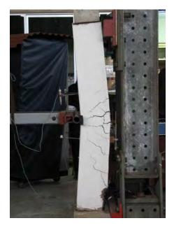
Figure 9. Out of plane bending test on reinforced adobe wall.
