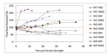
Figure 14. The flow rate retained versus percent ultimate tensile strength of five woven geotextiles.
