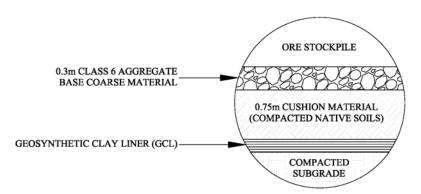
Figure 4. Two-hectare ore pad liner system detail.
