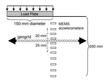
Figure 4. Test schematic for monitoring rotation. MEMS accelerometers were spaced 20 mm apart (center to center) near the geogrid and 25 mm apart further from the geogrid.
