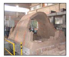
Figure 6. Reinforced vault and non reinforced vault after test.
