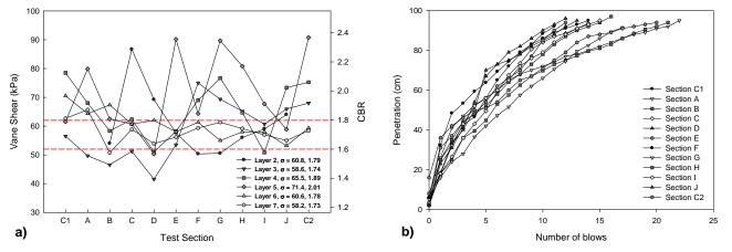
Figure 7. Average strength of artificial subgrade during construction: a) vane shear results, b) DCP results.
