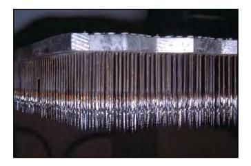
Figure 1. Needle Board
