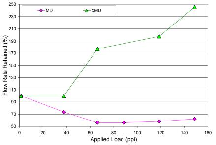
Figure 3. Flow Rate Retained (%) vs. Applied Load (ppi) for Woven, PP, Geotextile (Style B)
