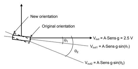
Figure 3. Calculating rotation of accelerometers with respects to horizontal.
