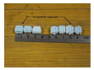
Figure 1. Photo showing a close-up view of typical individual pieces of geosynthetic aggregate.
