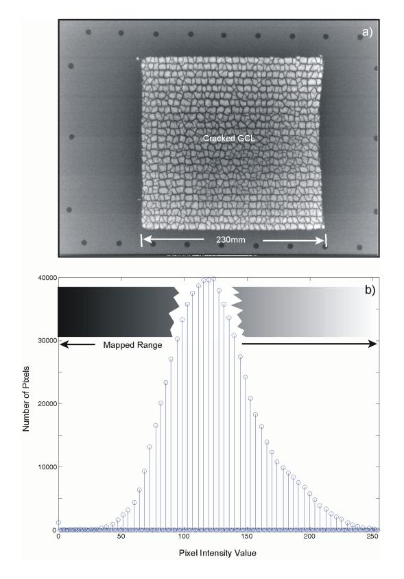
Figure 4. a) Histogram adjusted corrected image, and b) histogram of pixel intensity values
