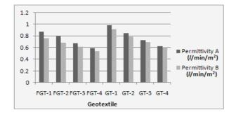
Figure 13. Permittivity of nanoclay formulated and standard polyester nonwoven geotextiles before/after immersion. (Where A, B mean before and after immersion, respectively)
