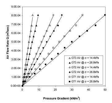
Figure 3 Geotextile air radial flow rate versus pressure gradient
