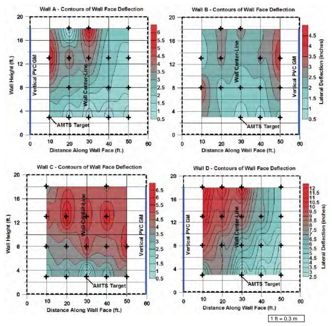
Figure 10: Horizontal Movement of the Face at End of Test
