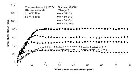
Figure 9. Direct shear stress versus direct shear displacement of geogrid with sand backfill
