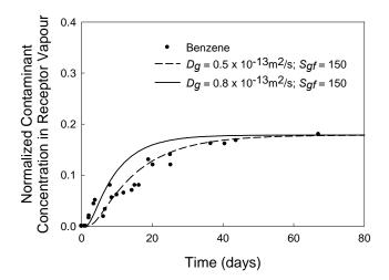
Figure 7. Change in benzene concentration in the receptor during vapour diffusion tests using co-extruded GM.
