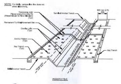
Figure 1. Turf reinforcement mat used in a trapezoidal channel or swale.
