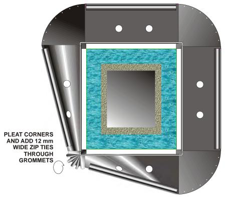
Figure 6. Gas Trapping Curtain Corner Pleating for Installation
