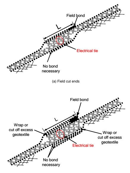
(b) Factory ends with excess geotextile
