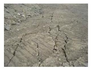
Figure 13 - Parallel cracks developed at the base, as the berm settled and shifted inward
