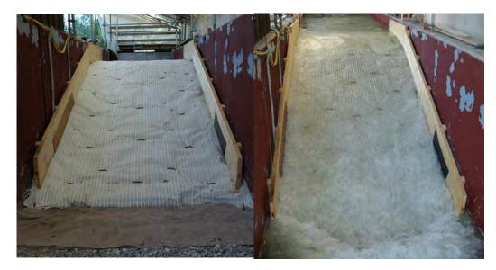
Figure 8. Model experiments at the Technical University Munich, Overflow of the inner embankment per method (II) Left: before overflow, right: in overflow state with up to 300 l/m s (Haselsteiner et al. 2007).
