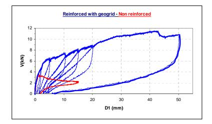
Figure 10. Comparative curves of plain and reinforced walls in bending.
