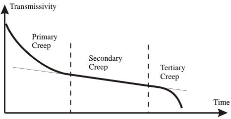
Figure 1: Creep behavior of planar drainage geosynthetics
