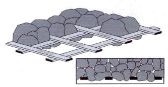
Figure 2. Interaction of aggregate with geogrid
