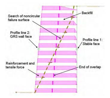
Figure 3. Limit equilibrium model of wall Test 2b
