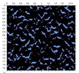
Figure 5: 3D topological characterization of a textured geomembrane (10 mil threshold)
