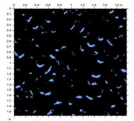
Figure 7: 3D topological characterization of a textured geomembrane (20 mil threshold)
