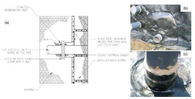
Figure 6. Design and installation of pipe penetrations: (a) design detail for side wall pipe penetration; (b) installation of side wall pipe penetration; and (c) installation of vertical monitoring port
