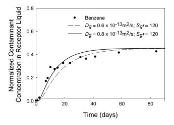
Figure 3. Change in benzene concentration in the receptor during dissolved phase diffusion tests using co-extruded GM.
