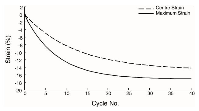
Figure 7. Comparison of maximum shrinkage strain versus that at centre of seam
