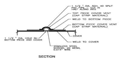
Figure 11. Perimeter Vent Detail
