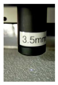
Figure 3. Photograph illustrating scanning beam directly downward to a textured geomembrane surface.
