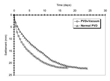
Figure 5. Settlement-time relationship from large consolidometer of reconstituted sample in the laboratory using PVDs with and without vacuum preloading
