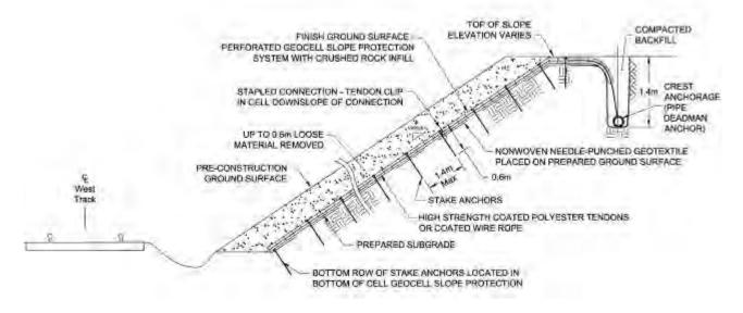
Figure 2. Site 1 geocell slope protection system detail (not to scale) (Boyle and Hudak, 2003).
