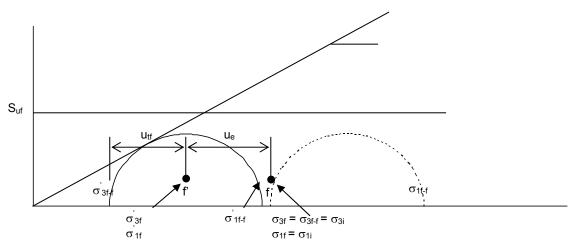
Figure 3. States of stress and undrained shear strength for post-construction and trafficking subgrade
