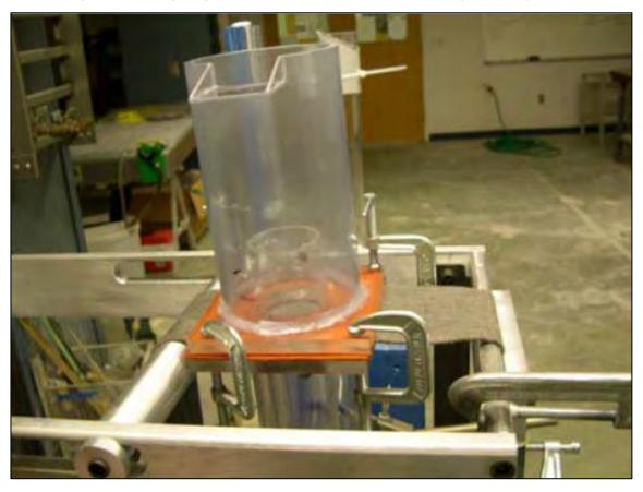
Figure 1. Mounting the geotextile test specimen in the tensile loading permittivity apparatus
