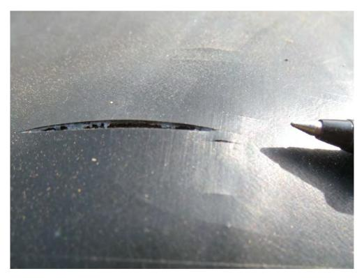
Figure 1. Stress cracks on die lines at subgrade stone protrusion.
