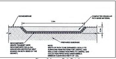
Figure 2 Access Path Detail
