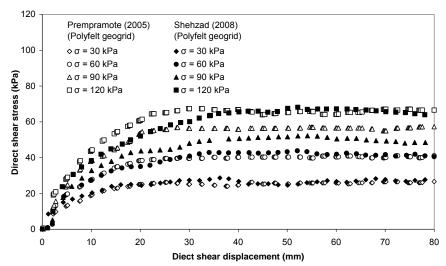
Figure 10. Direct shear stress versus direct shear displacement of geogrid with tire chips-sand backfill
