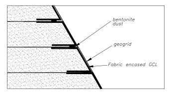
Figure 6 Particular of the reinforced earth embankment
