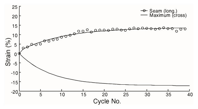
Figure 8. Seam separation as compared to absolute maximum shrinkage.
