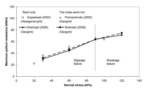
Figure 6. Maximum pullout resistances versus normal stresses for sand and tire chips-sand mixture
