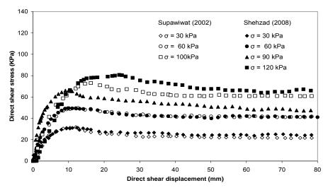
Figure 7. Direct shear stress versus direct shear displacement of sand only
