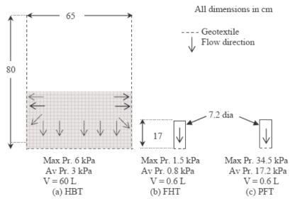
Figure 6. Comparison of Hanging Bag, Falling Head and Pressure Filtration Test Conditions.
