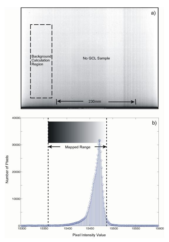
Figure 2. a) X-ray image of empty aluminum tray, and b) histogram of pixel intensity values
