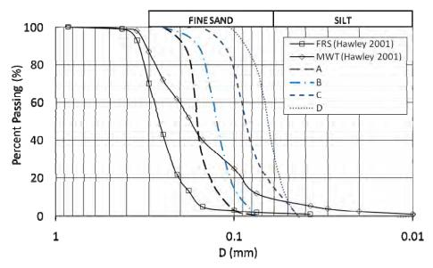
Figure 3. Soil gradations tested in cyclic flow
