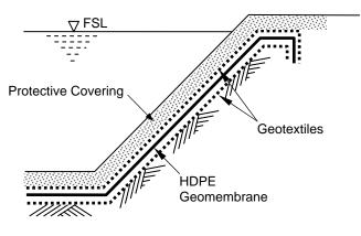
Figure 1. Typical cross section of the Canal Lining with Geomembrane and Geotextiles
