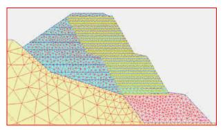
FIG. 3. Finite Element Model of Reinforced Slope in PLAXIS by Jewell Method
