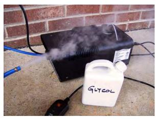
(d) Low pressure smoke generator producing liquid smoke from tube
