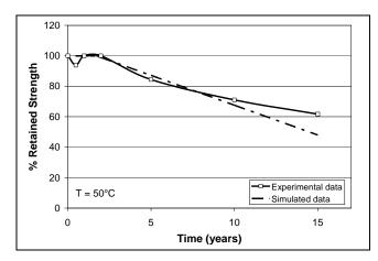
Figure 4. Comparison between experimental and simulated results for HTPET exposed to deionized water at 50°C.
