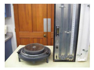
Figure 1 Radial Transmissivity Testing Device – ASTM D 6574 (Courtesy of TRI/Environmental, Inc.)
