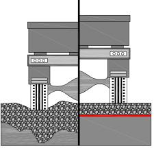
Figure 1. Illustration of geotextile separation function
