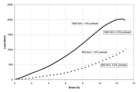
Figure 1. 2-inch Wide, 0.5 and 1.0% Preload, Avg of All Specimens - Lab #1
