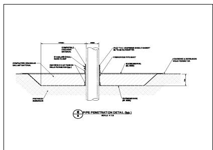
Figure 6 Modified Pipe Penetration Detail
