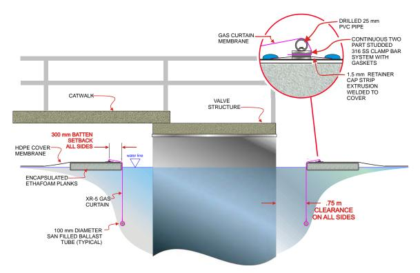
Figure 4. Gas Trapping Curtain Section Detail at Valve Structure
