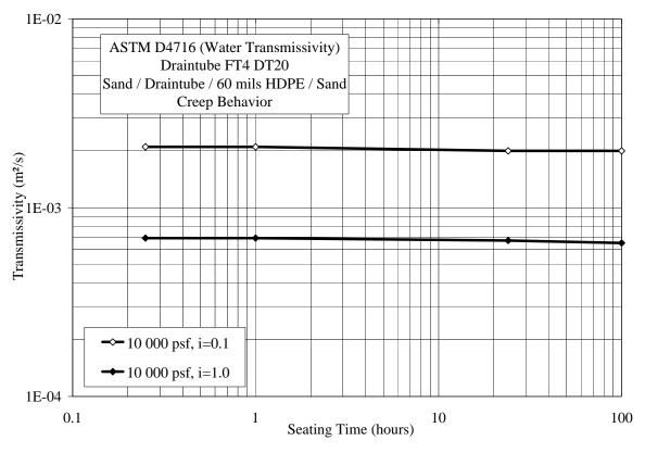
Figure 7: Effect of time on the transmissivity of "Draintube" geocomposite
