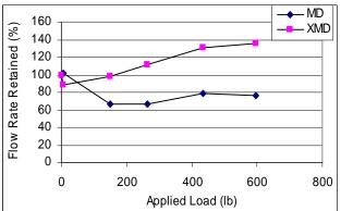
Figure 12. Flow rate retained versus applied load of the PP-woven-4 geotextile.
