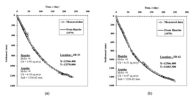
Figure 11. Back-calculated compressibility parameters of field observations of PVDs with vacuum preloading (a) Station ZB 53 (b) Station ZB 62
