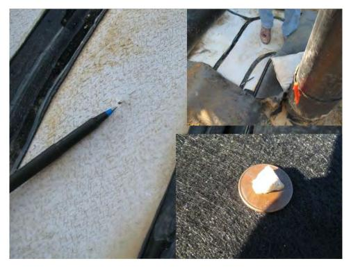
Figure 12. Small stone that penetrated 1.5 mm textured HDPE on concrete.
