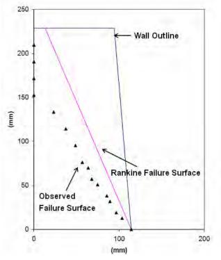
Figure 2. Compound failure at Test 2b, L/H=0.4 (Woodruff, 2003)
