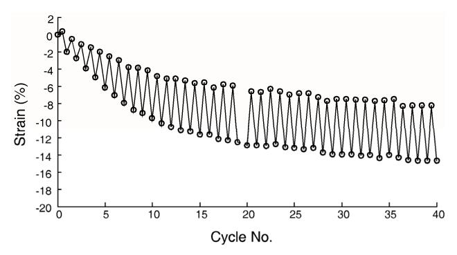
Figure 5. Shrinkage and swelling strain.
