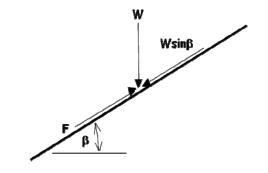
Figure 4. Breaking force of separation box with slope angle in waste landfills
