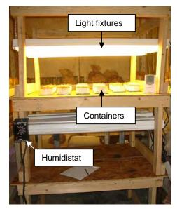
Figure 1. The test setup in the environmental chamber
