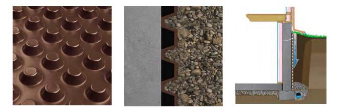
Figure 2: 'Air gap' function of dimple sheet
