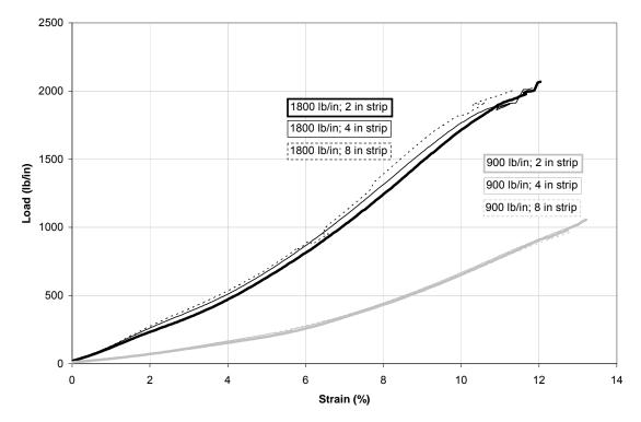
Figure 5. All Widths, 1.0% Preload, Avg of All Specimens - Lab #1
