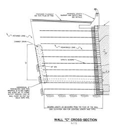
Figure 3. Cross-section of a wall using a stone backdrain.
