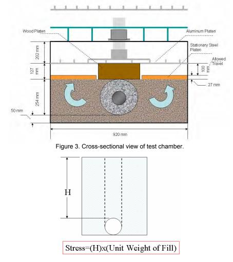
Figure 4. Moser's prism load concept to estimate long-term stress over a flexible conduit (Moser 1990).
