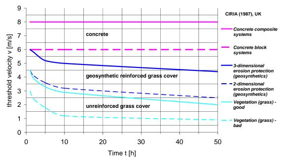
Figure 4. Effectiveness of non-armored and armored grass covers on dam embankments during overflow (CIRIA 1987).
