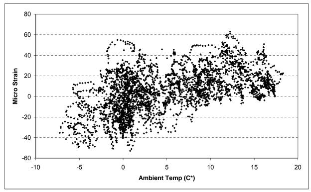
Figure 10 Weaker correlation for strain gages that did not correlate as well with ambient temperature.
