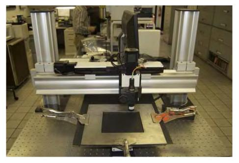
Figure 2. Photograph of an Optical Scanning Apparatus.
