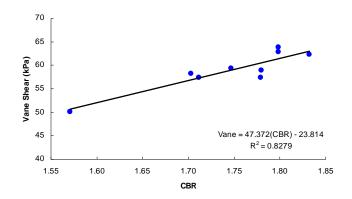
Figure 1. Relationship between California Bearing Ratio and the hand-held vane shear device.
