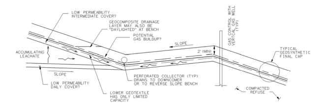
Figure 5. Typical inward sloping landfill bench.
