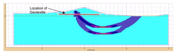
Figure 5. Failure surface with geotextile and without water. FOS = 1.51 at geotextile rupture.
