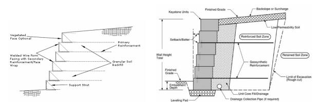
Figure 1. Welded wire vegetated face.
