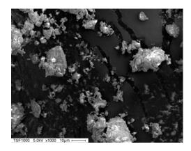
Figure 4. Scanning electron microscope (x1000) image of fines used in this study.
