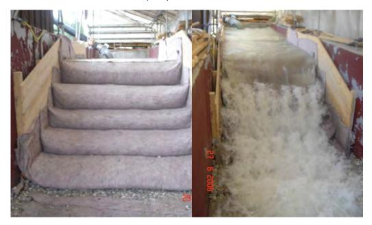
Figure 7. Model experiments at the Technical University Munich, Overflow of the inner embankment per method (III). Left: before overflow, right: in overflow state with up to 130 l/m·s (Haselsteiner et al 2007).
