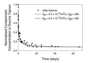
Figure 6. Change in *m*&*p*-xylenes concentration in the source during vapour diffusion tests using co-extruded GM.
