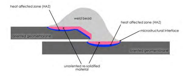
Figure 6. Cross section microstructure of extrusion weld.
