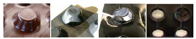
(a) No failure(b) Cracking(c) Severe cracking(d) Severe crackingFigure 8: Observations of the degradation of dimple sheets during a Stress-Cracking test per SAGEOS GD001
