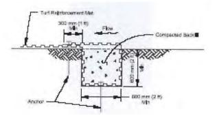
Figure 7. Terminal anchor trench (upstream) detail.
