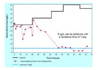
Figure 1. Column test result for selenium concentration decrease
