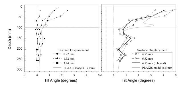
Figure 8. Rotation angle at the plate edge as a function of depth and applied surface displacement with geogrid reinforcement at 100 mm depth. PLAXIS modeling results are shown at two displacement levels for comparison.
