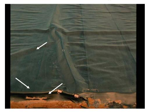
Figure 1 Isolated locations (arrowed) of stress cracking on wrinkles of HDPE liner in black liquor pond
