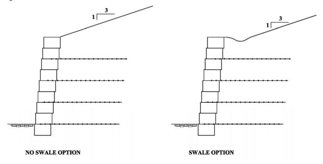
Figure 3. Distinction between no-swale or swale behind masonry blocks.
