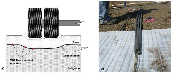
Figure 8. Displacement measurements: a) lead wire measurement locations, b) protective tubing.
