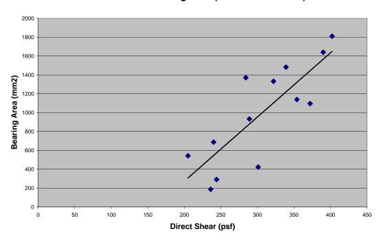
Direct Shear vs Bearing Area (0.15mm threshold)
