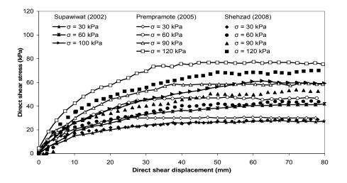
Figure 8. Direct shear stress versus direct shear displacement of tire chips-sand backfill
