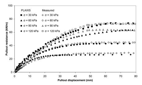
Figure 13. Comparison of measured and predicted pullout resistance from tire chips-sand backfill using finite element software
