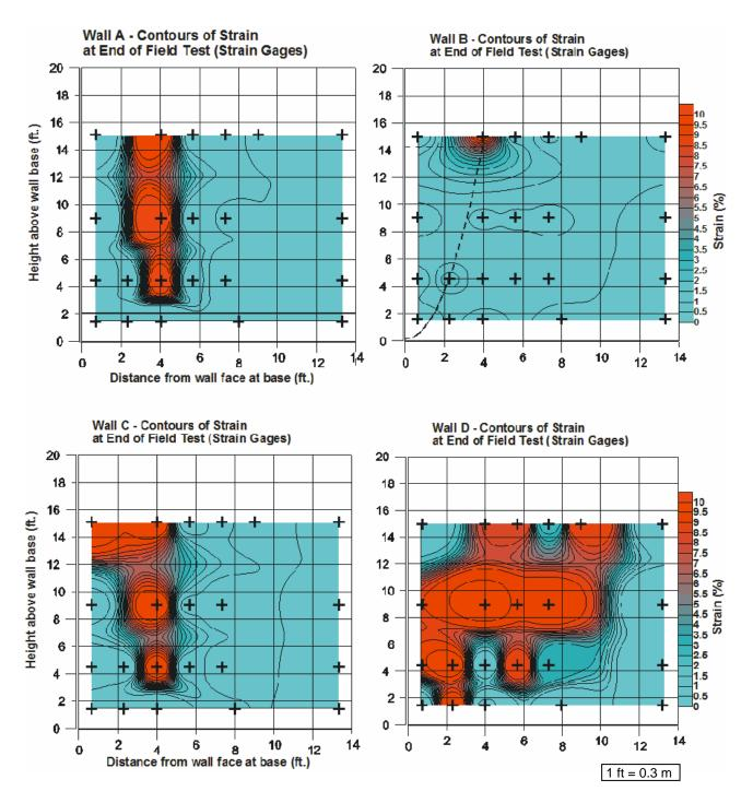
Figure 7: Strain in Reinforcement at End of Test
