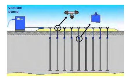
Figure 4. Cross-section of PVDs with vacuum preloading method
