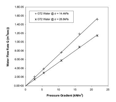
Figure 4 Geotextile water radial flow rate versus pressure gradient
