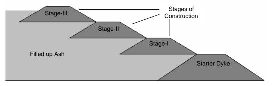
Figure 2 Raising of ash dyke by the upstream method of construction
