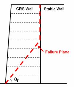
Figure 8. Define inclination angle of failure plane
