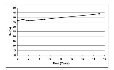
Figure 5. Evolution of crystallinity with time exposure for PET yarn exposed to deionized water at 50°C.
