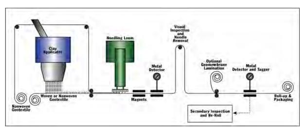
Figure 2. The needlepunched GCL production needle detection and removal system.
