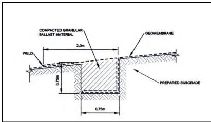
Figure 8 Primary Wind Uplift Ballast Trench
