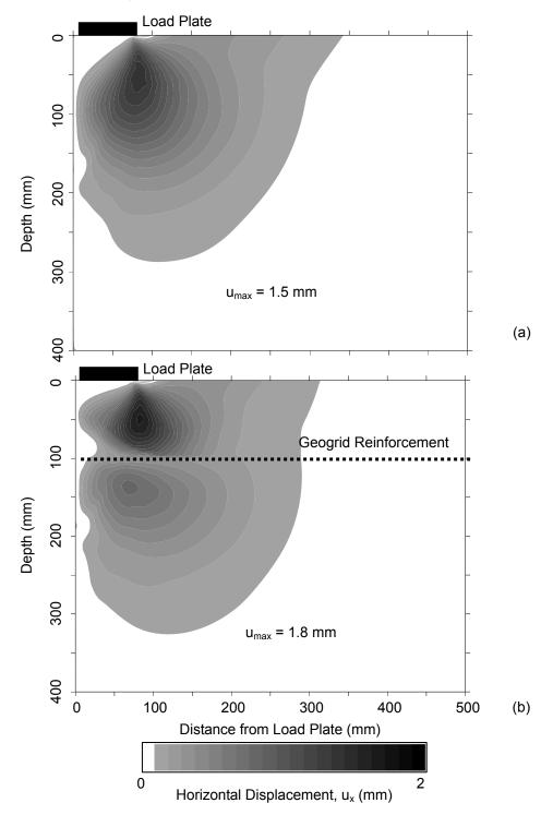
Figure 6. Horizontal displacement from PLAXIS analysis below a circularly loaded plate when (a) no geogrid is present, (b) geogrid is buried at 100 mm depth
