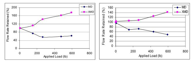
Figure 9. Flow rate retained versus applied load of the PP-woven -1 geotextile.
