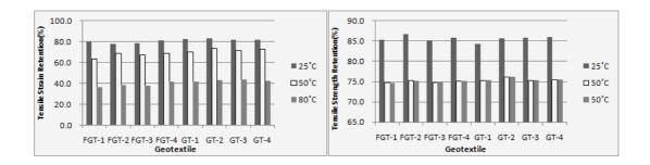
Figure 9. Chemical resistance by tensile property retention of nanoclay formulated and standard polyester nonwoven geotextiles.
