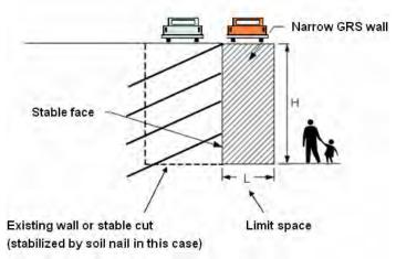
Figure 1: A narrow GRS wall system for widening of existing highway
