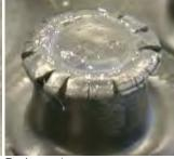
Rating = 4 Collapsed Dimple
