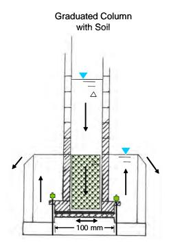
Figure 1. Cross section of testing device. (bold arrows are flow directions)
