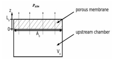
Figure 1. Lay out of gas permeability test based on the falling-pressure method.
