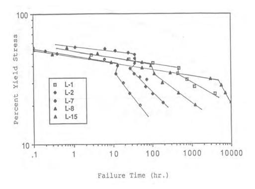
Figure 2. Stress rupture curves for five HDPE geomembranes (Hsuan et al, 1992).
