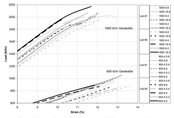
Figure 13. Close-up of Ultimate Strain Region - Avg of All Specimens - Labs #1 & #2
