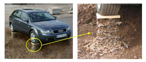
Figure 3. Lateral restraint of aggregate using high modulus laid and welded geogrids
