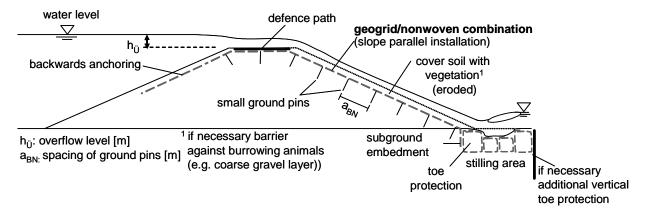
Figure 5. Overflow protection per method (II), embankment parallel with geogrid/nonwoven combinations and ground pins (Haselsteiner et al. 2007)
