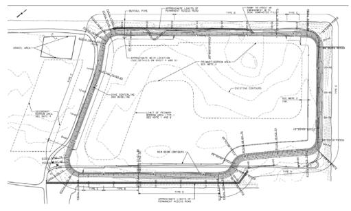
Figure 2 - Plan of Cleveland CDF 12 raised berm design
