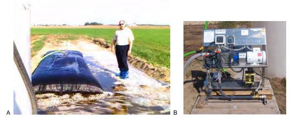
Figure 2. Swine manure was conditioned with Solve 10 followed by Solve 9248 and subsequently pumped into an agricultural weight geotextile tube container (A). WaterSolve's WSLP-2400 polymer make-down unit activated and injected Solve 9248 to the swine residual inline prior to the Geotube containers (B).
