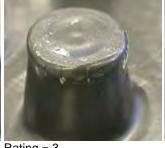
Rating = 3 Severe cracking
