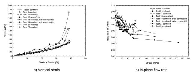
Figure 8. Test results obtained on GA drainage systems without pipe.
