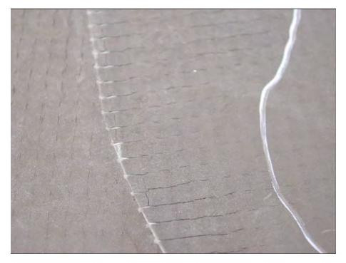
Figure 8. Stress cracking above warp yarns oriented at 90° in liner and patch.
