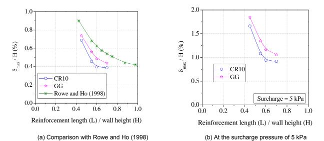
Figure 8. Relationship between maximum panel displacement ( $\delta_{max}$ ) /wall height to reinforcement length / wall height for different reinforcements
