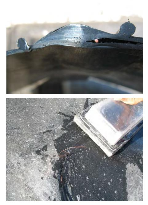
Figure 11. Installed (top) and exposed (bottom) conductive wire for water lance testing.
