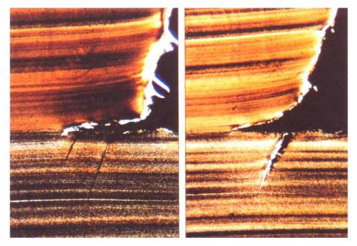
Figure 5. Initial crazing and opened stress crack at edge of weld bead.
