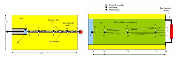
Figure 3. Dimension geocomposite tail (150\*50 cm) and sensors positioning.
