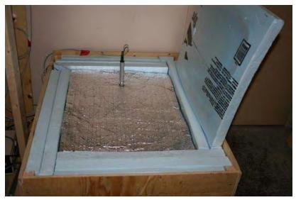
Figure 7: Insulation details around the soil box in the model
