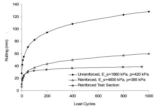
Figure 4. Unreinforced and Reinforced rutting predictions and comparisons
