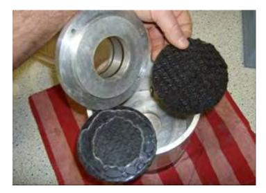
Figure 5. A geocomposite test specimen and its sealant so as to fix it the base of the flow cylinder.
