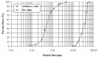
Figure 2. Gradation of tire chips and sand
