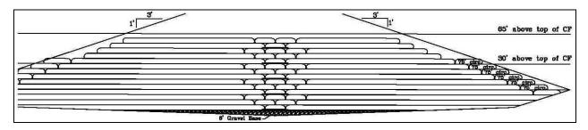
Figure 4. Cross-section of the CF, 140 feet north of the weep water sump, showing the first nine layers of tubes.
