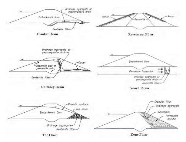
Figure 1. Examples of Potential Geotextile Applications in Embankment Dams (after FEMA draft document)
