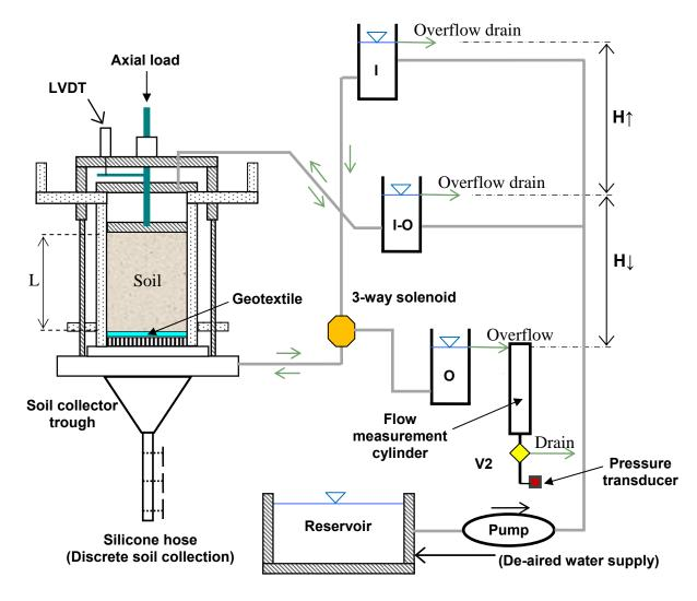
Figure 1. System configuration of Cyclic Gradient Ratio test device
