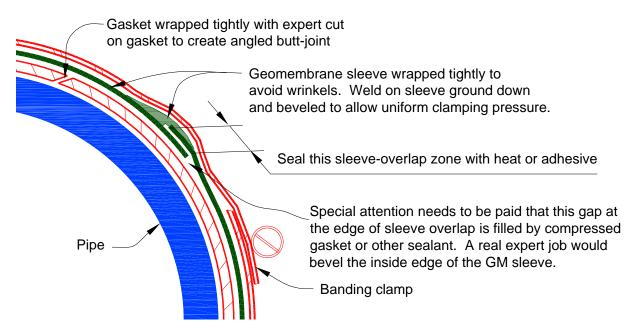
Figure 3. Detail schematic of critical gasketed boot issues.
