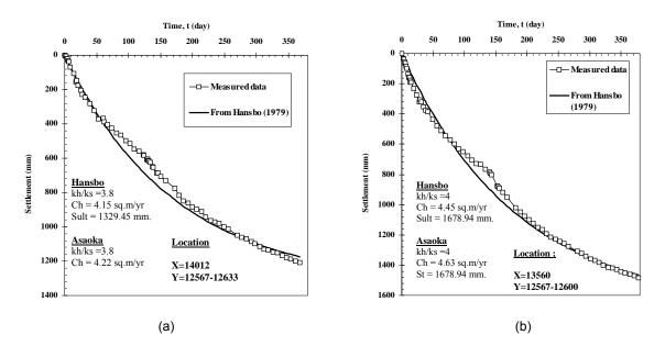
Figure 10. Back-calculated compressibility parameters of field observations of PVDs with embankment (without vacuum preloading) (a) X=14012 Y=12567-12633 (b) X=13560 Y=12567-12600
