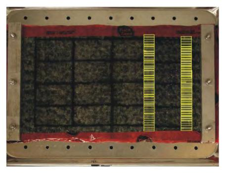
Figure 4. Virtual GeoPIV "patches" used to track seam movement
