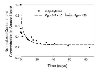
Figure 2. Change in *m&p*-xylenes concentration in source during dissolved phase diffusion tests using co-extruded GM.
