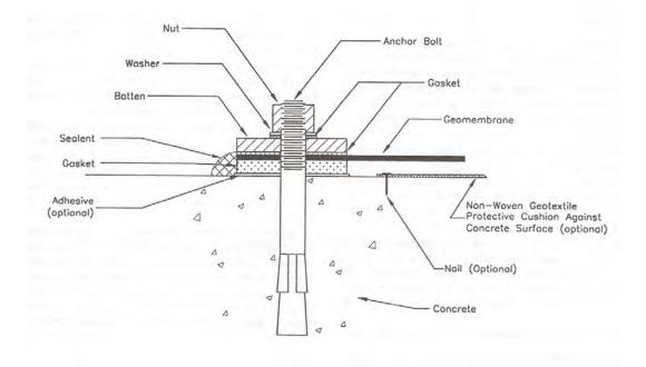
Figure 4. Cross section shown in ASTM D6497.
