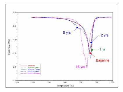
Figure 6. Evolution of heat flow with temperature and time exposure for PET yarn exposed to deionized water at 50°C.
