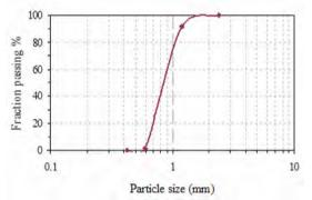
Figure 2 Particle size distribution curve for guartz sand
