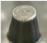
Rating = 1 No cracking observed
