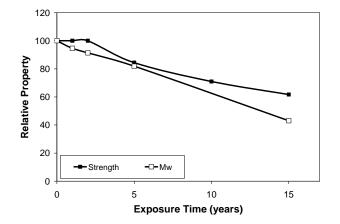
Figure 9. The relative change in Breaking Strength and Mw in H2O at 50°C.
