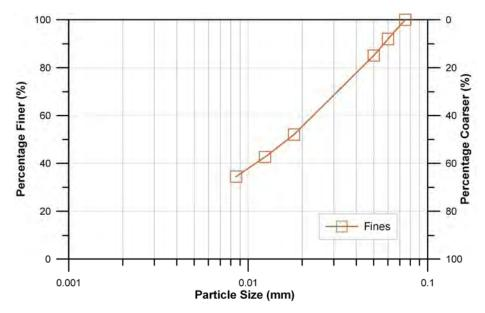
Figure 3. Particle size distribution of fines used in this study.
