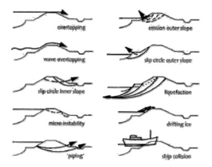
Figure 5. Potential failure modes of coastal structure (adopted from Pilarcyzk, 2000)
