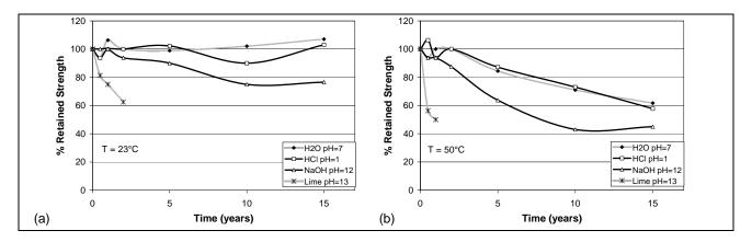
**Figure 2.** Hydrolytic degradation of PET yarns in various media (1<pH<13) at (a) 23°C and (b) 50°C during 15 years.
