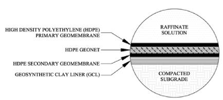
Figure 3. Evaporation pond liner system detail.
