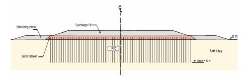
Figure 3. Cross-section of PVDs with embankment method (Seah, 2006)
