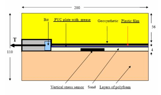
Figure 6. Schematic filling of the tank.
