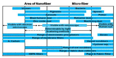
Figure 7. Relationship between separation fields and separation membranes using nanotechnology.
