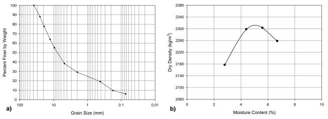
Figure 2. Base course material properties: a) grain-size distribution, b) compaction curve.
