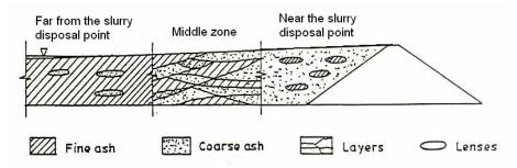
Figure 1 Sorting and layering in an Ash Pond (Modified after Datta, et al., 1996)
