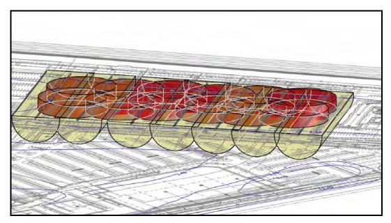
Figure 3: 3D model of estimated radii of vacuum influence from the horizontal and vertical LFG extraction wells
