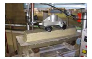
Figure 2. Gas permeability test on a compacted clay liner specimen subjected to a 4 point bending test (Barral et al., 2008).
