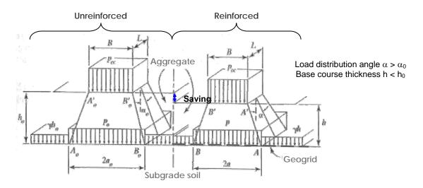
Figure 4. Increase of load distribution capacity with the use of geogrids (Koerner 1998)
