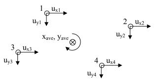
Figure 2. Coordinate system and displacement vectors used to calculate the average rotation between particles.
