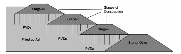
Figure 3 Possible use of PVDs for raising of ash dyke by the upstream method of construction
