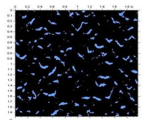
Figure 6: 3D topological characterization of a textured geomembrane (15 mil threshold)
