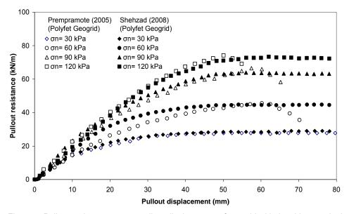
Figure 5. Pullout resistance versus pullout displacement of geogrid with tire chips-sand mixture
