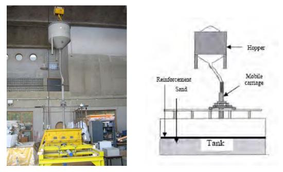
Figure 4. Pluviation system (INSA Lyon, LGCIE, Coulomb 3).
