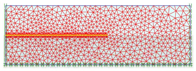
Figure 11. Pullout mesh generated by finite element software (at true scale)
