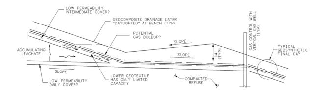
Figure 4. Typical outward sloping landfill bench.
