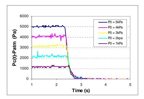
Figure 3. Results obtained on a non deformed CCL specimen under different pressure gradients (Barral et al., 2008).
