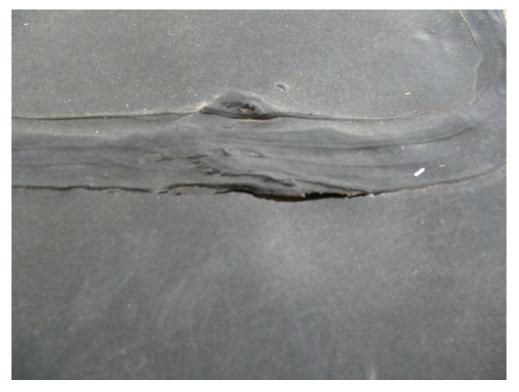
Figure 4. Stress crack (arrowed) along edge of extrusion weld.
