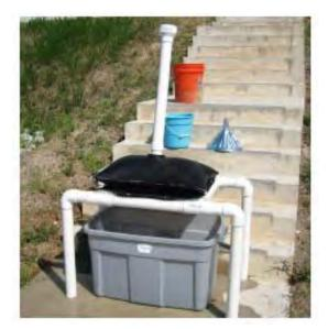
Figure 4 - Apparatus assembled to perform the Simulated Dewatering Test (TenCate<sup>™</sup> Geotube<sup>®</sup> GDT guideline).
