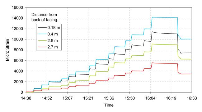
Figure 6 Strain measured in geogrid at elevation 14.4 feet next to the shaft spaced two diameters from the wall facing.
