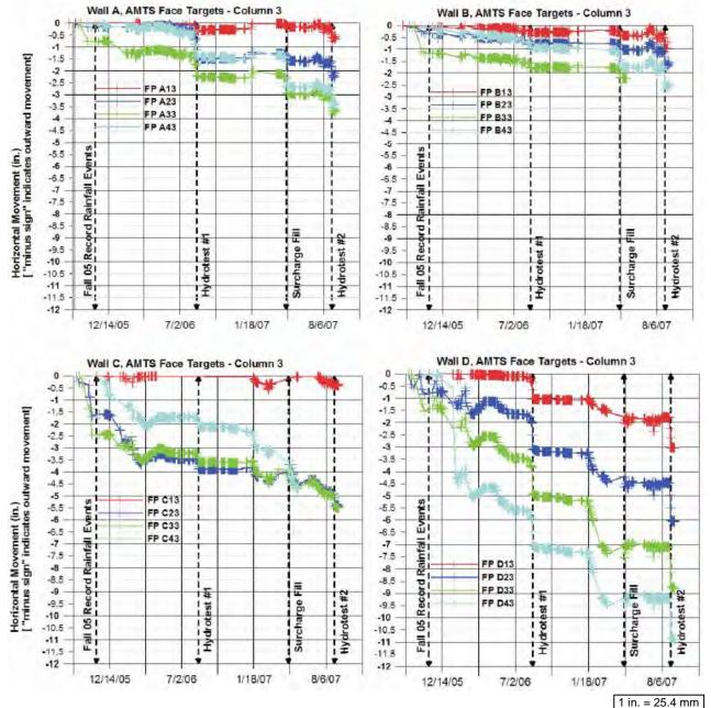
Figure 9: Horizontal Movement of Face at Centerline of Each Wall
