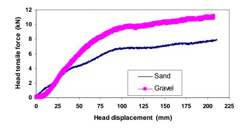
Figure 8. Tensile force at the head of geocomposite sample (vertical stress equal to 7 kPa).
