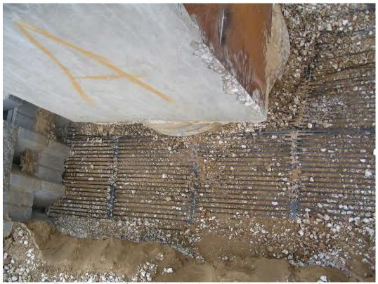
Figure 5 Exhumed section of geogrid showing elongation and tension in the reinforcement.
