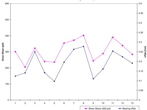
Direct Shear vs. Bearing Curve sPpk
