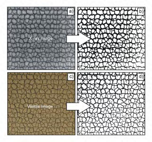
Figure 6. Crack distribution in a) X-ray image, b) thresholded X-ray, c) visible image, and d) thesholded visible image
