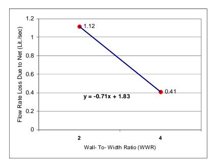
Figure 4. Flow Rate Loss Due to Net VS. Wall-To-Width Ratio
