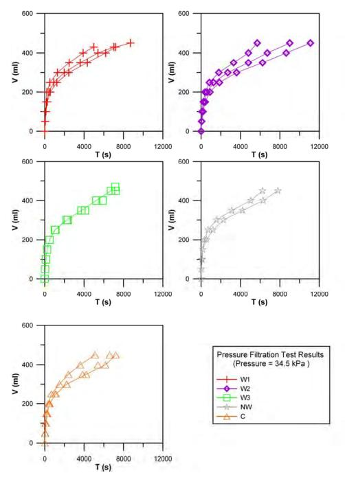
Figure 5. Temporal flow characteristics from pressure filtration tests.
