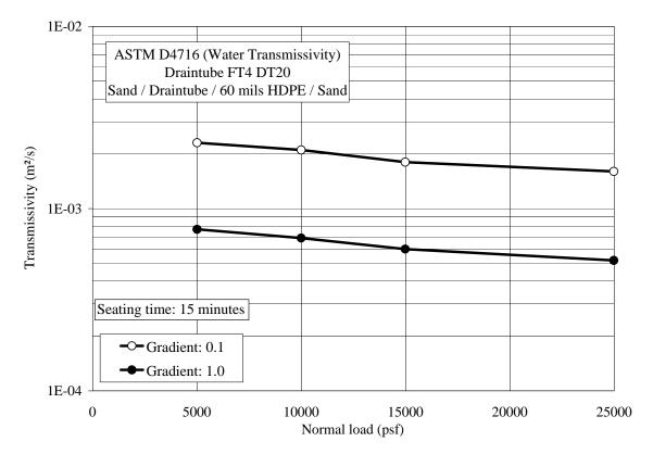
Figure 6: Effect of normal load on the transmissivity of "Draintube" geocomposite
