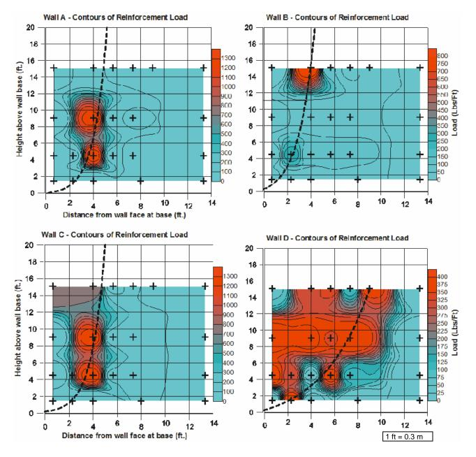
Figure 8: Force in Reinforcement at End of Test
