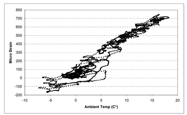
Figure 9 Data from strain gages that correlated well with ambient temperature.
