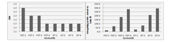
Figure 11. Allowable tensile strength of nanoclay formulated and standard polyester nonwoven geotextiles.
