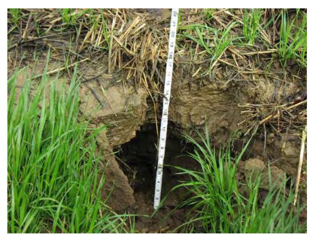
Figure 2. Void created by sapping of sand from below silt layer (ruler is in inches).
