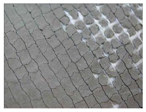
Figure 9. Stress cracking above both warp (vertical) and weft (horizontal) yarns.
