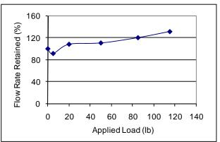
Figure 6. Flow rate retained versus applied load of the heatset NW geotextile.
