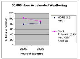
Figure 6 Tensile Results from 30,000 UV Test
