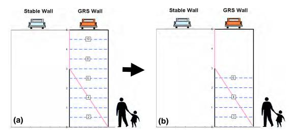
Figure 10. Illustration of two conceptually identical systems: (a) with upper layer reinforcements; (b) without upper layer reinforcements
