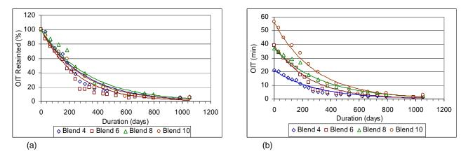
Figure 3. (a) Changing of OIT retained versus time of blends with CB at  $85^{\circ}$ C oven (b) OIT versus time of blends with CB at  $85^{\circ}$ C oven
