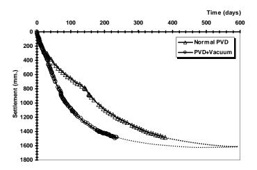
Figure 8. Comparison of settlement of PVD improvement with and without vacuum preloading (Sta. X=13560, Y=12567-12600 for PVDs with embankment and Sta. X=12566.4, Y = 12583.500 for PVDs with vacuum preloading)
