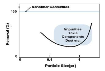
Figure 4. Effect of using a nanofiber geotextile filter.
