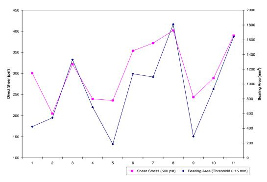
Figure 11. Chart of Direct shear vs. Bearing Area (0.15mm threshold) by sample.
