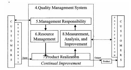
Figue 4. ISO 9001 Process Flow Diagram
