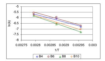
Figure 7. Arrhenius Plot of blends with CB
