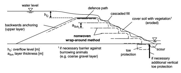
Figure 6. Integrated overflow protection per method (III) in envelope method (Haselsteiner et al 2007).
