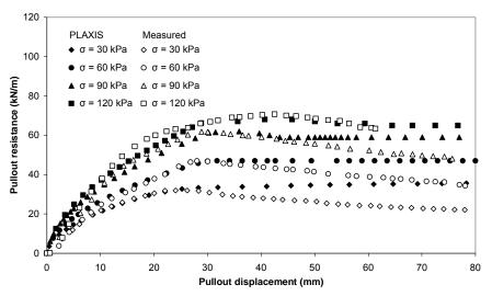
Figure 12. Comparison of measured and predicted pullout resistance from sand backfill using finite element software
