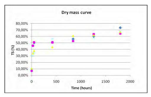
Figure 8 - Simulated Dewatering Test tests results of Sediment A.
