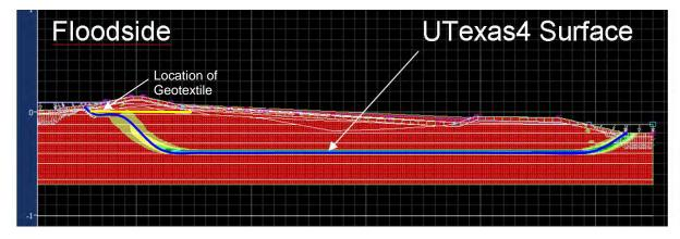
Figure 10. Comparison of the limit equilibrium failure surface (shown in blue) with numerical analysis accumulated shear strains for Lake Cataouatche section.
