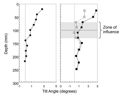
Figure 9. "Zone of influence" (shaded area) determined using rotation angle test results: (a) no geogrid and (b) geogrid at 100-mm depth. The solid symbols represent the rotation angles at maximum surface displacement and the open symbols represent the difference between the rotation angles with and without reinforcement (Δθ=θ reinforced-θ unreinforced).
