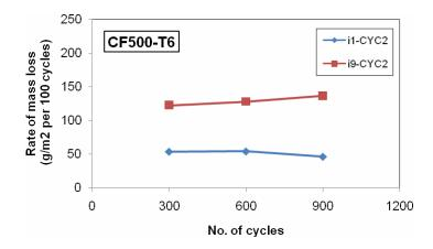
Figure 5. Rate of mass loss versus number of cycles
