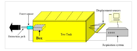
Figure 5. Pull-out test materiel (from Abdelouhab et al. 2008).
