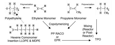
Figure 1. Chemical structures of olefin monomers and their structures after polymerization.
