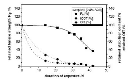
Figure 4. Change in break and AO with exposure time (Boehning et al., 2008)
