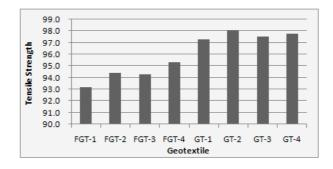
Figure 10. Biological resistance by tensile strength retention of nanoclay formulated and standard polyester nonwoven geotextiles.
