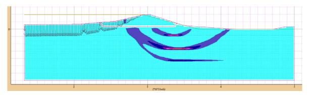
Figure 6. Failure surface without geotextile with WL = 19.5 ft. FOS = 1.20.
