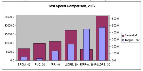
Figure 20, Comparison of Elmendorf and Tongue Tear Results at 20°C
