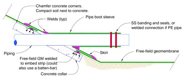
Figure 6. Concrete collar for attachment of free-field geomembrane at base of penetration to keep stress off of skirt-to-sleeve weld (courtesy of GSE Lining Technology).
