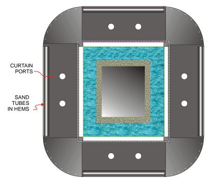
Figure 5. XR-5 Gas Trapping Curtain Plan
