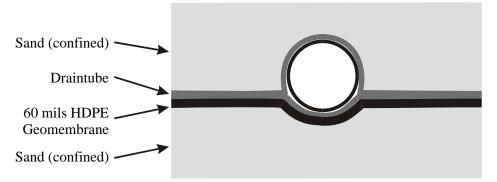
Figure 5: Test configuration
