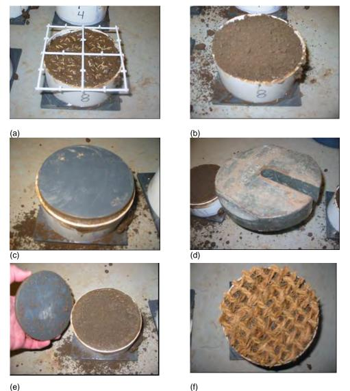
Figure 2. Steps involved in the preparation of the vegetated containers
