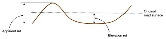
Figure 11. Illustration of rut measurements
