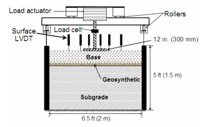
Figure 6. Schematic diagram of the pavement test facility
