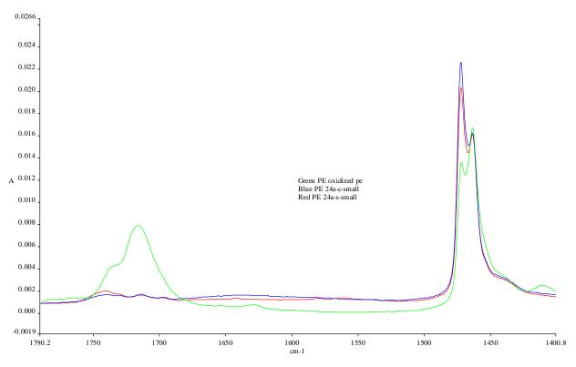
Figure 10. FTIR spectra of oxidized (green) and unoxidized (red/blue) PE.
