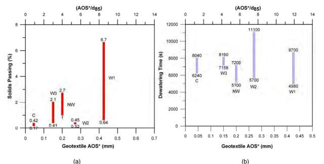
Figure 6. (a) Solids Passing and (b) Dewatering time versus geotextile AOS and (AOS/d<sub>85</sub>). Note:\* Manufacturer value
