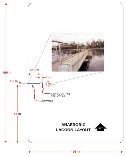
Figure 1. Anaerobic Lagoon Layout
