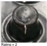
Rating = 2 Minor cracks
