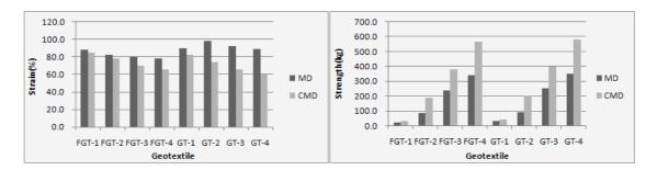
Figure 8. Tensile properties of nanoclay formulated and standard polyester nonwoven geotextiles. (Where MD, CMD mean the machine and cross machine directions, respectively)
