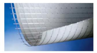
Figure 5. Combigrid<sup>®</sup> Geocomposite (geogrid reinforcement & needle punched nonwoven geotextile, firmly bonded between the cross laid reinforcement bars)
