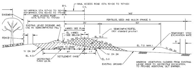
Figure 4 Typical Section Jefferson Parish Lakefront Levee (USACE, Nov 1987)
