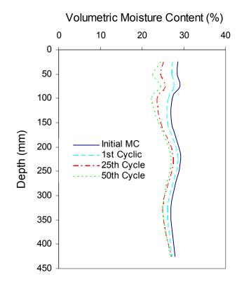
Figure 9: Volumetric moisture content profile in subsoil for heat/cool cycles
