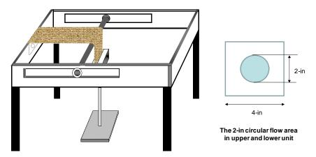
Figure 1b. Loading frame sketch and 2-inch flow area in the upper and lower units.
