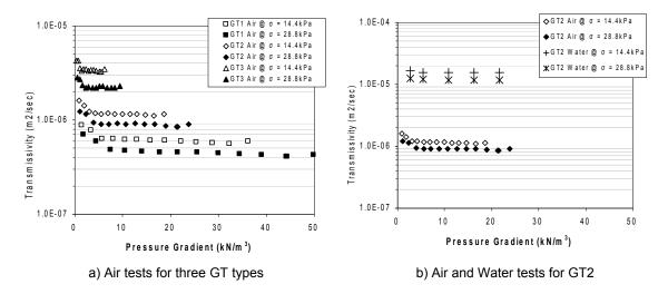
Figure 5 Radial transmissivity of geotextiles vs. pressure gradient
