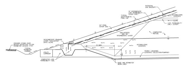
Figure 2. Perimeter anchor trench with some design issues.
