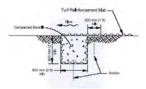
Figure 2. Initial anchor trench downstream detail.
