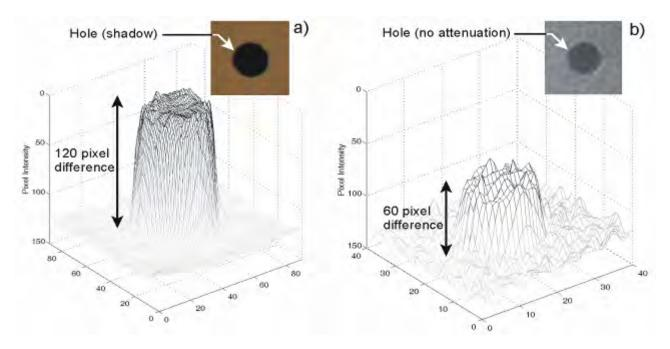
Figure 5. Pixel intensities of photogrammetric control markers in a) visible image, and b) x-ray image
