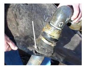
(a) Failed pipe boot at skirt-to-sleeve weld.
