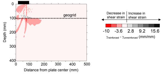
Figure 5. Difference in shear strains between reinforced and unreinforced sections for geogrid at a depth of 100 mm.
