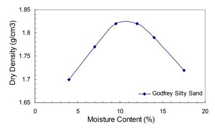
Fig. 2: Compaction curve for Godfrey foundation soil
