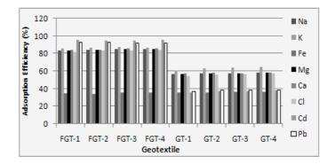
Figure 16. Component adsorption of nanoclay formulated and standard polyester nonwoven geotextiles.
