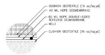
Figure 8. Details of welding with smooth 40-mil and textured 60-mil geomembranes
