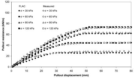
Figure 15. Comparison of measured and predicted pullout resistance from tire chips-sand backfill using finite difference software
