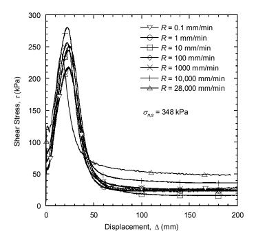
Figure 2. Shear stress-displacement relationships for seven monotonic shear tests at 348 kPa.
