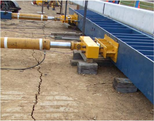
Figure 4 Cracks developed at the back of the reinforced soil mass.
