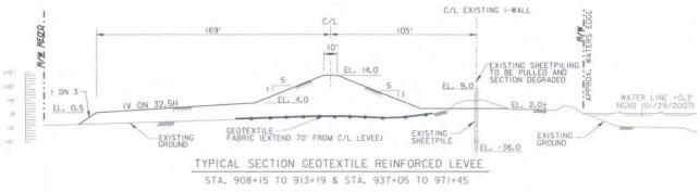
Figure 5 Typical Section of Reinforced Levee behind Existing I-Wall
