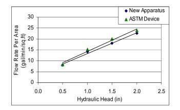
Figure 2. Comparing the flow behavior of ASTM D4491 test device and the new apparatus.
