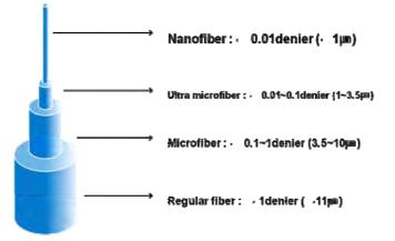
Figure 1. Comparison of nanofibers to conventional standard fibers.
