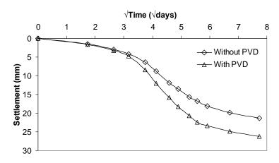
Figure 9 Settlement vs. square root of time for pond ash type NC
