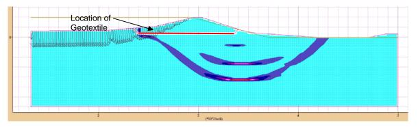
Figure 7. Failure surface with geotextile with WL = 19.5 ft. FOS = 1.30.
