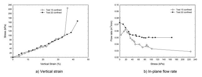
Figure 9. Test results obtained on high density GA drainage systems without pipe.
