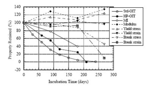
Figure 3. Change in break and OIT properties with exposure time (Hsuan, 2008)
