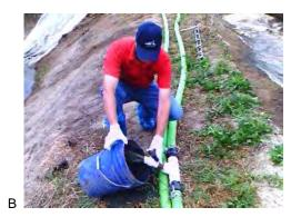
Figure 3. Chemically conditioned (Solve 9248) swine manure (right) and geotextile tube filtrate water (left) collected 06 September 2007 (A). Sample port used for monitoring inline chemical conditioning (B).
