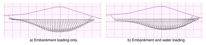
Figure 8. Geotextile displacement showing effect of storm surge water loading.
