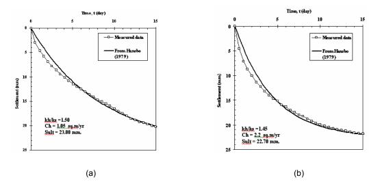
Figure 6. The observed and fitted curves for settlements to determine C<sub>h</sub> values for the reconstituted specimen in large consolidometer (a) PVD with surcharge and (b) PVD with vacuum preloading
