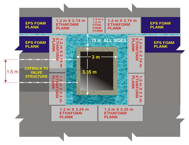
Figure 2. Foam Plank Detail at Concrete Structure
