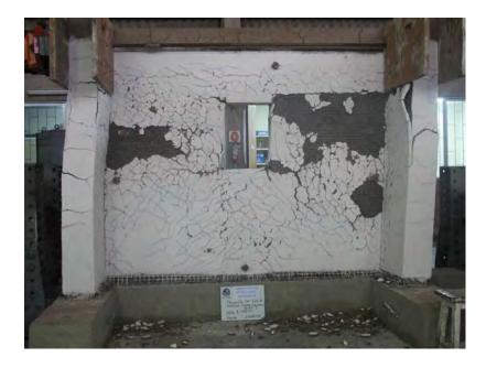
Figure 7. Cyclic shear test on reinforced adobe wall.
