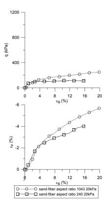
Figure 3. Stress-strain-volumetric response of the studied mixtures for a confining stress of 20kPa.
