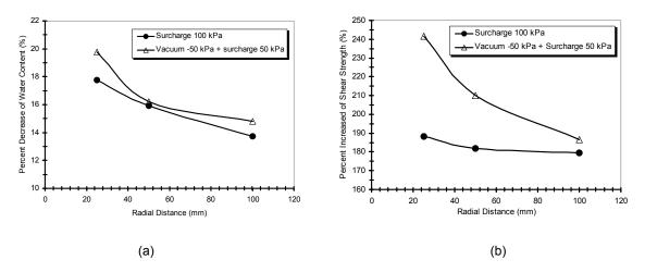
Figure 7. After consolidation test of the consolidometer using reconstituted samples of PVD with and without vacuum preloading (a) Water content reduction (b) Shear strength increase
