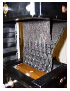
Figure 2. Peel testing of a drainage composite per ASTM D7005.
