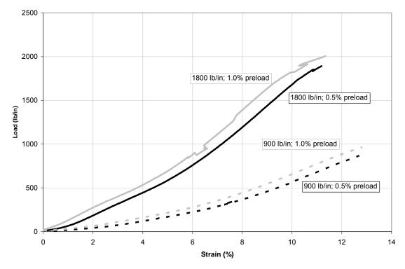
Figure 3. 8-inch Wide, 0.5 and 1.0% Preload, Avg of All Specimens - Lab #1
