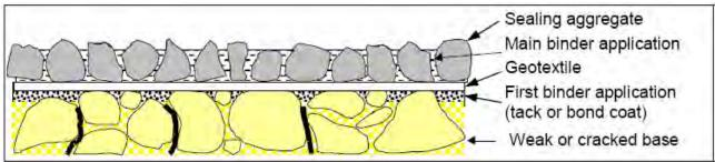
Figure 1 Paving Fabric Under Single Chip Seal (Alderson, 2006)
