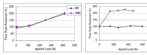
Figure 7. Flow rate retained versus applied load of the SF woven geotextile.
