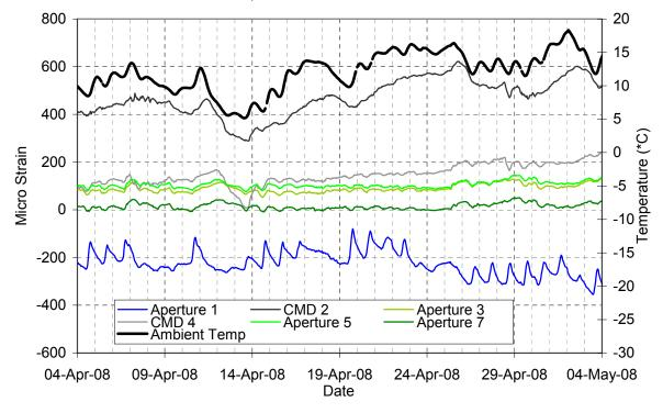
Figure 8 Shows temperature and all strain measurements at elevation 6.7 ft over a period of one month for four gages that correlate with ambient temperature and two that do not correlate.
