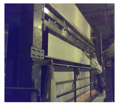
Figure 3. After detection, crewperson on catwalk checks for needle fragment(s).
