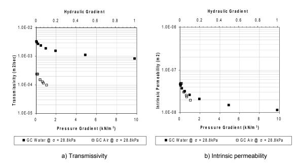
Figure 8 Linear-flow transmissivity and intrinsic permeability of geocomposite vs. pressure gradient
