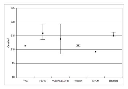
Figure 1 – Range in Cost for Exposed Geomembrane Liners
