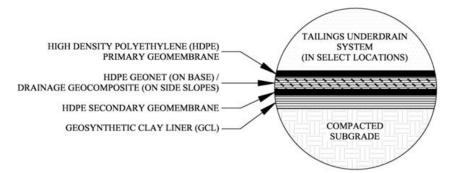
Figure 2. Tailings cell liner system detail.
