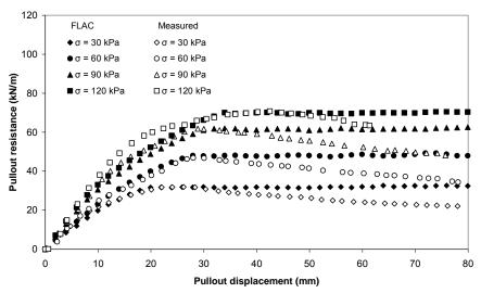
Figure 14. Comparison of measured and predicted pullout resistance from sand backfill using finite difference software
