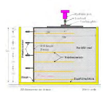
Figure 1. Test layout of reinforced soil wall
