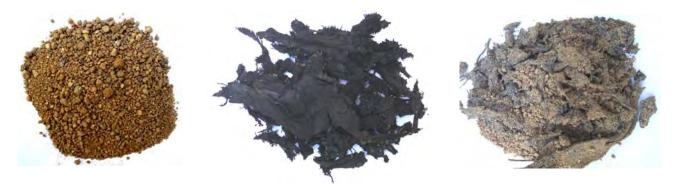
Figure 1. Sand, Tire-Chips and Tire Chips-Sand Mixture
