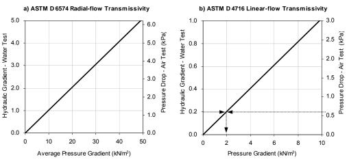
Figure 2 Equivalent Pressure Gradient Charts for Transmissivity Tests Example: On Chart b), for a hydraulic gradient i = 0.2 in water test, one can find the equivalent pressure drop  $\Delta P = 0.60$  kPa in the air test, and both are equivalent to a pressure gradient P<sub>G</sub> = 2.0 kN/m<sup>3</sup>.
