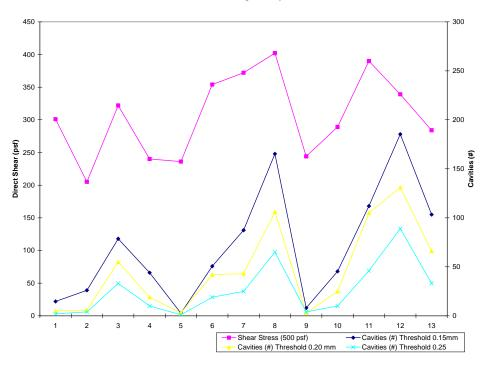
Figure 10. Chart of Direct shear vs. Filling Quantity – Cavities (0.15, 0.20 and 0.25 mm threshold) by sample.
