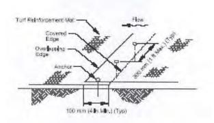
Figure 5. Turf reinforcement mat overlap joint.
