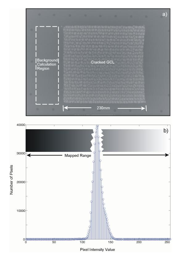
Figure 3. a) Corrected X-ray image and b) histogram of pixel intensity values
