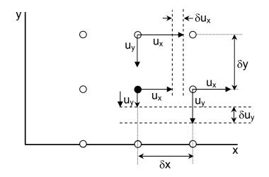
Figure 1. Relative displacement and rotation of particle in two dimensions with respect to x and y axes.
