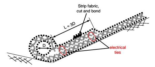
(a) Drainage pipe on a slope
