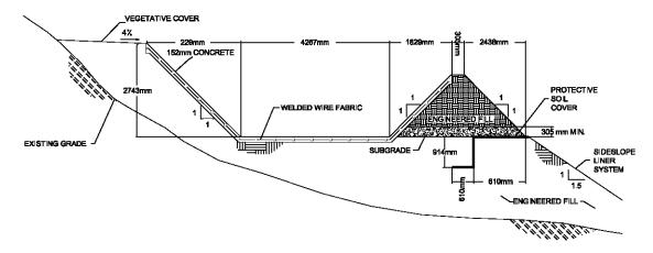
Figure 2. Initially proposed anchor trench
