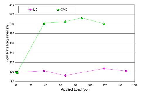
Figure 4. Flow Rate Retained (%) vs. Applied Load (ppi) for Woven, PET, Geotextile (Style C)
