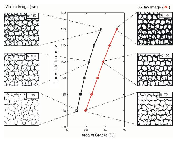
Figure 7. Effect of threshold intensity on apparent crack area on visible (a-c) and X-ray images (d-f).
