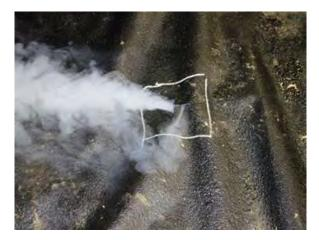
(a) Smoke emerging from inlet x-cut after tube is removed
