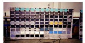
Figure 1 One of three natural weathering sample racks after 6 years of exposure.
