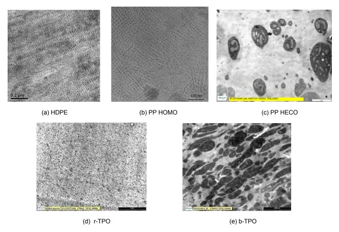
Figure 3. Micrographs demonstrating unique polyolefin morphology by type.
