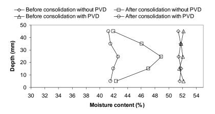
Figure 10 Profiles of moisture contents with and without PVDs for pond ash type NF
