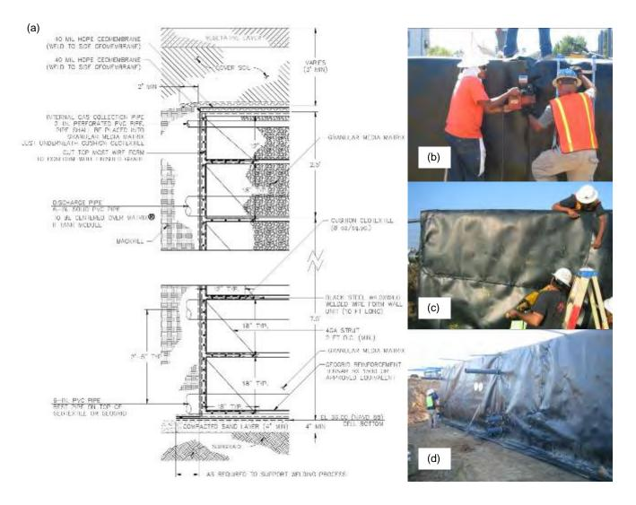
Figure 7. Side wall design detail and construction: (a) design of a side wall; (b) photo of fusion welding on a side wall; (c) extrusion welding for a folding part on a side wall; (d) construction of a side wall
