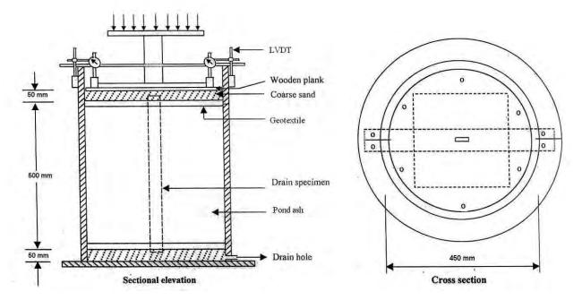
Figure 4 Typical arrangement for model test on pond ash with prefabricated vertical drains (Modified after Sampath Kumar, 2000)
