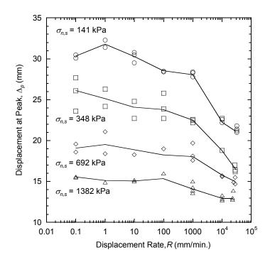
Figure 4. Effect of displacement rate on displacement at peak shear strength for monotonic shear.
