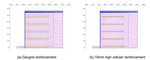
Figure 10. Geometry used in finite element analysis for reinforced soil wall with different reinforcement heights
