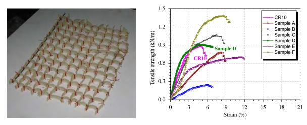
(a) Manually manufactured cellular reinforcements
