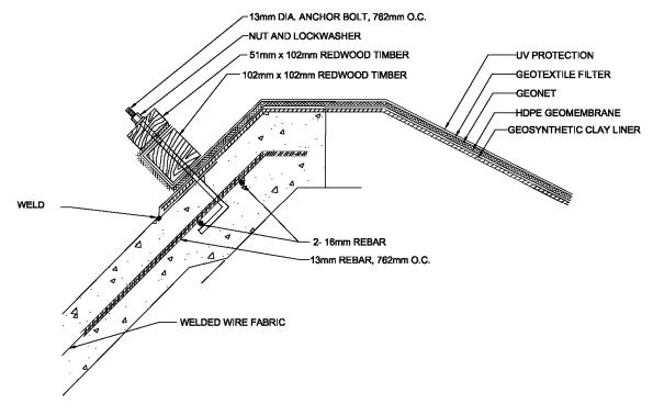
Figure 3. Batten strip anchorage system.
