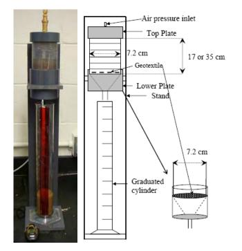
Figure 2. Pressure filtration test apparatus and schematic.
