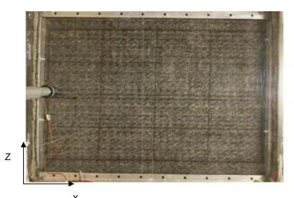
Figure 5: Installation of GCL in the big-box model
