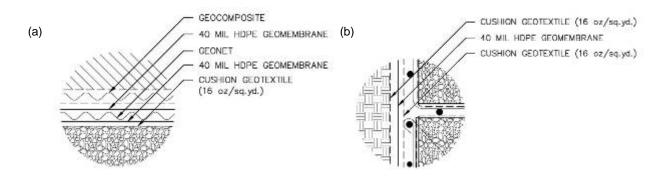
Figure 5. Details of geosynthetic systems: (a) top liner system and (b) liner system on the side
