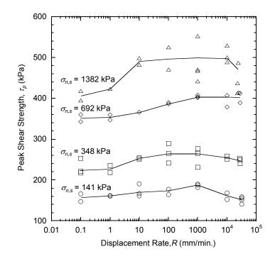
Figure 3. Effect of displacement rate on peak shear strength for monotonic shear.
