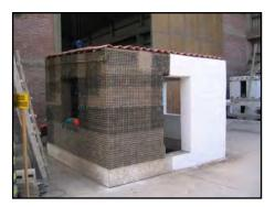
Figure 4.Model reinforced with geogrid, half plastered
