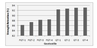
Figure 14. Strength retention of nanoclay formulated and standard polyester nonwoven geotextiles after clogging.
