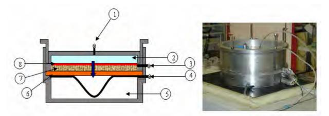
Figure4. Cell with a deformed base: 1 Water inflow; 2 Water pressure; 3 Gas outflow; 4 Gas inflow; 5 Porous mould; 6 GCL; 7 Sand; 8 Membrane (Pitanga et al., 2008).
