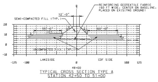
Figure 3 Typical design cross section of Cleveland CDF 12 raised berm where geosynthetic reinforcement was used
