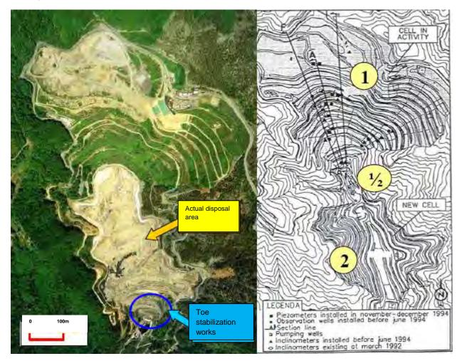
Figure 1 Scarpino landfill plant. The aerial view on the left is taken before the stabilization works begun. The picture on the right shows a plant of the disposal site in 1994.
