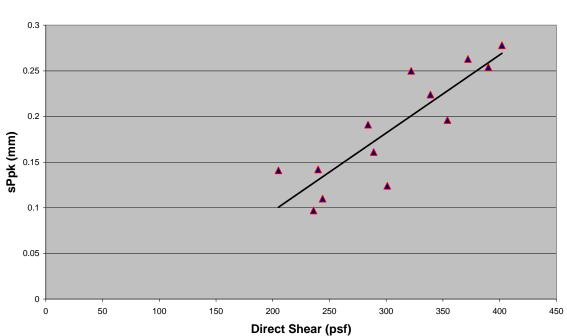
Direct Shear vs. sPpk (Bearing curve) with trend line
