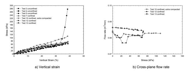
Figure 10. Test results obtained on GA drainage systems with pipe.
