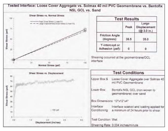
Figure 2. Direct shear test: Interface dry for test assembly, and then submerged after assembly.
