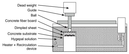
Figure 6: Stress-cracking test for dimple sheets
