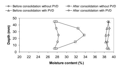
Figure 11 Profiles of moisture contents with and without PVDs for pond ash type NC
