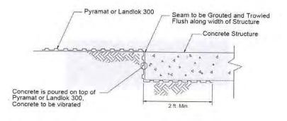
Figure 8. Transition detail between hard armor and TRMs or HPTRMs.
