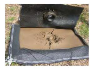
Figure 5 - Simulated Dewatering Test opened to check the dewatering level (TenCate<sup>™</sup> Geotube® GDT guideline).
