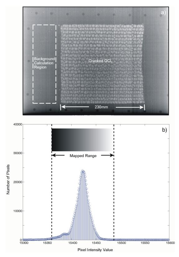
Figure 1. a) Raw X-ray image of GCL sample on aluminum tray, and b) histogram of pixel intensity values
