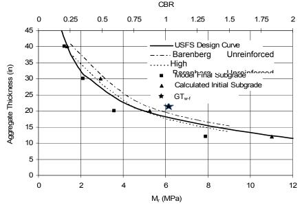
Figure 5: Model final subgrade CBR versus aggregate thickness with consideration for pore water pressure.
