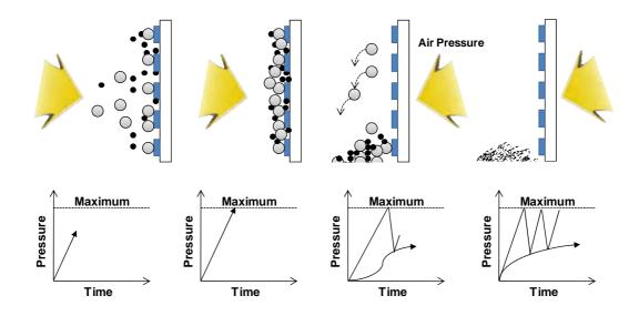
Figure 5. Maintenance of filtration efficiency for nanofiber filters.
