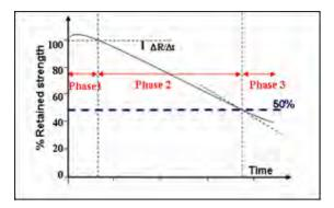
Figure 3. General hydrolytic degradation evolution with an incubation period followed by a constant rate.
