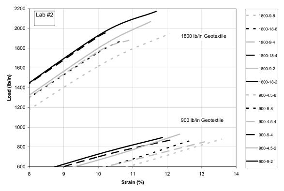
Figure 11. Close-up of Ultimate Strain Region – Avg of All Specimens – Lab #2
