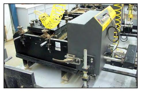
Figure 1. Photograph of a interface friction test apparatus.
