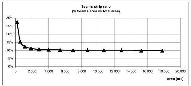
Figure 1. Relationship between the seam strip and the total area of the facility
