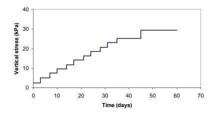
Figure 7 Application of Vertical pressure with time
