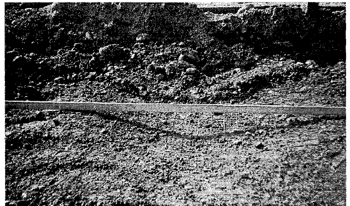
Figure 8: GGML2 and GGR1 section with CBR = 3 and T = 300 mm after 1000 EAL. The measurement beam is shown.
