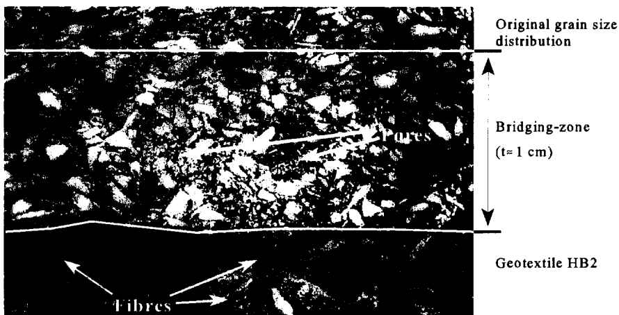
Figure 7. Microstructure at the interface Geotextile HB2/ Soil A (2 nd Test series; hydraulic gradient i=12 )
