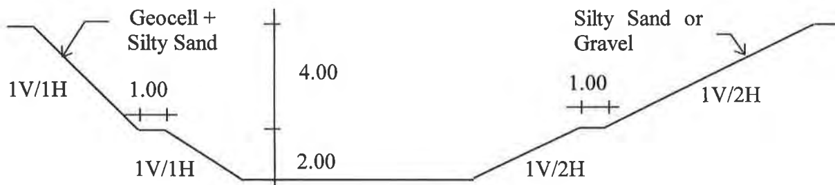
Figure 1 : Cross section of the liner systems on 1/1 and 1/2 slopes for the experimental GCL landfill cell.
