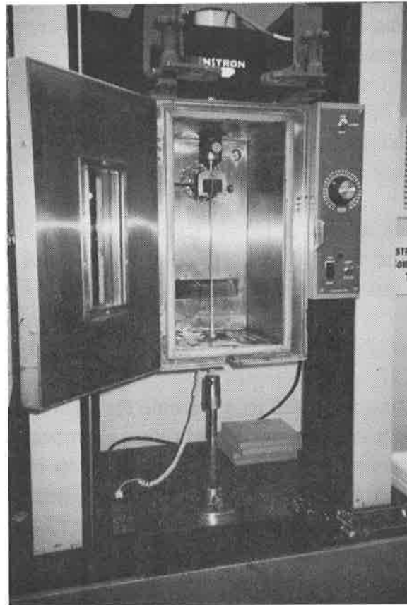
Figure 1. View of test apparatus showing conditioning chamber.
