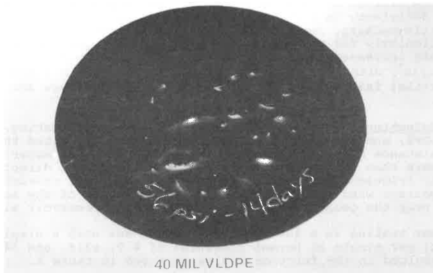
Figure 6. View showing condition of the 1-mm thick VLDPE after 14 days of testing on talus subgrade. Geomembrane did not fail.
