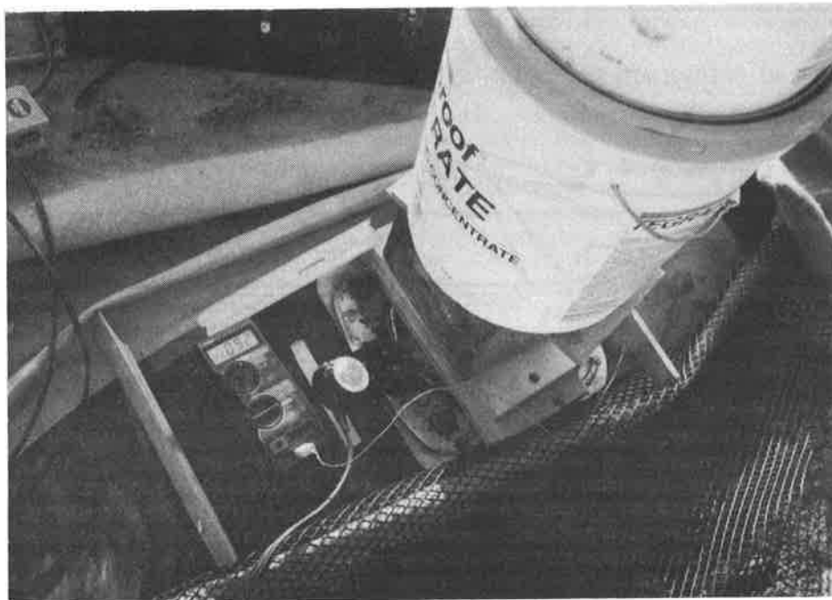
Figure 4. Application of Elevated-Temperature and Pressure During Attachment of the Strain Gauges to HDPE.
