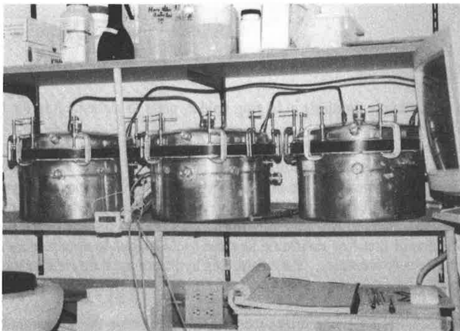
Figure 2. Fully assembled GCL test chambers.
