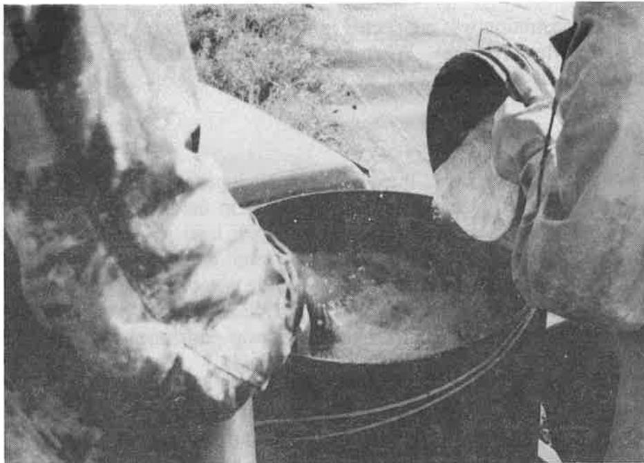
Figure 8. Mixing the Clay Slurry
