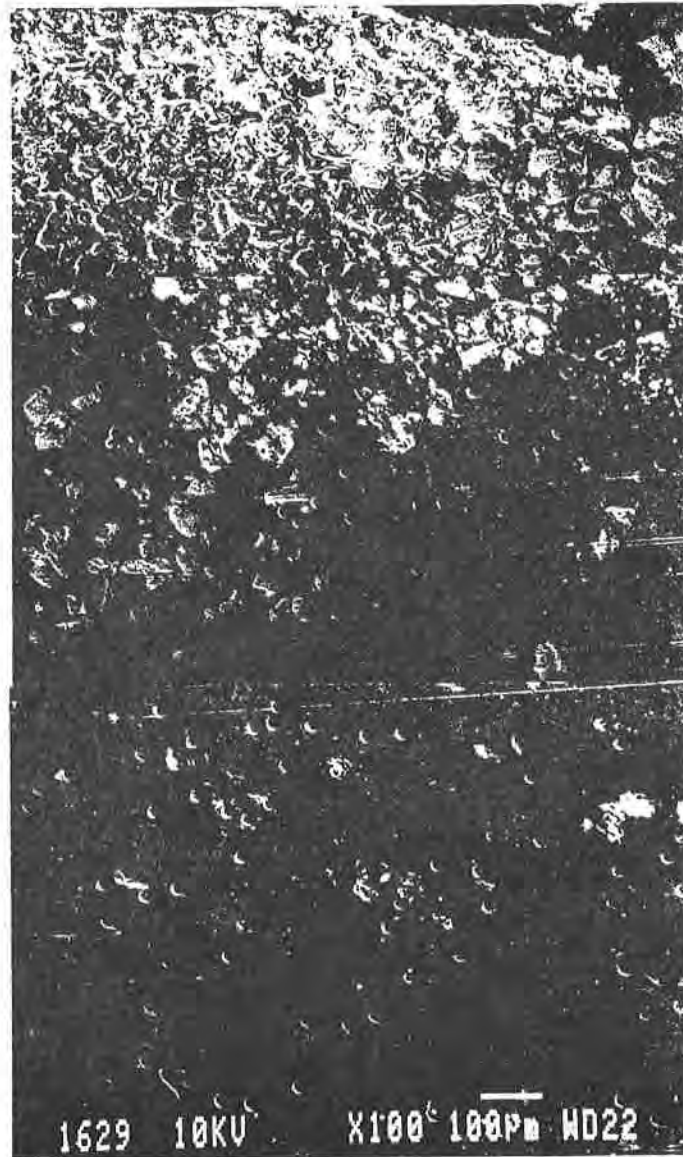
Figure 6 Microscopic view of cake at the surface of geotextile A1 after test under C_U = 5 \text{ g/l}
