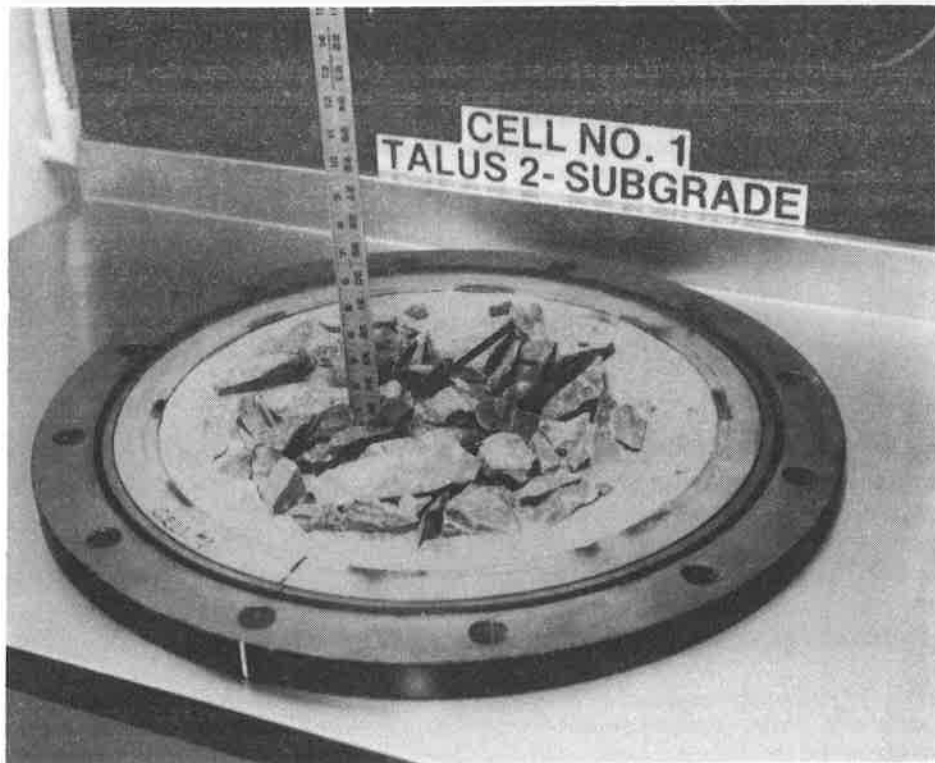
Figure 3. View to subgrade containing talus material obtained from Black Lake Dam. The arrow is pointing to the rock referred to in table 1 as the "killer" rock.
