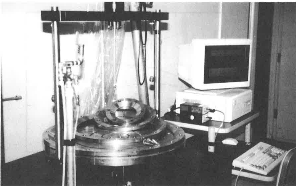
Figure 1 Axisymmetric tension test apparatus with 4 different clamping ring diameters
