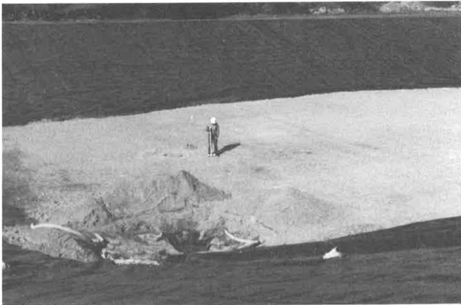
FIGURE 9. VIEW OF LANDFILL CELL WITH AN ELECTRICAL LEAK LOCATION RECONNAISSANCE SURVEY IN PROGRESS
