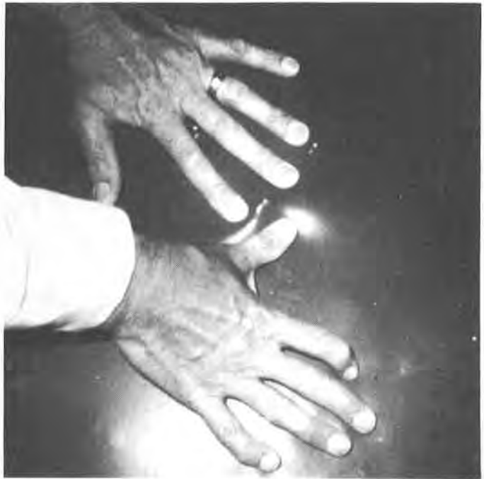
Figure 8: Geomembrane over one of the small, sharp rocks.
