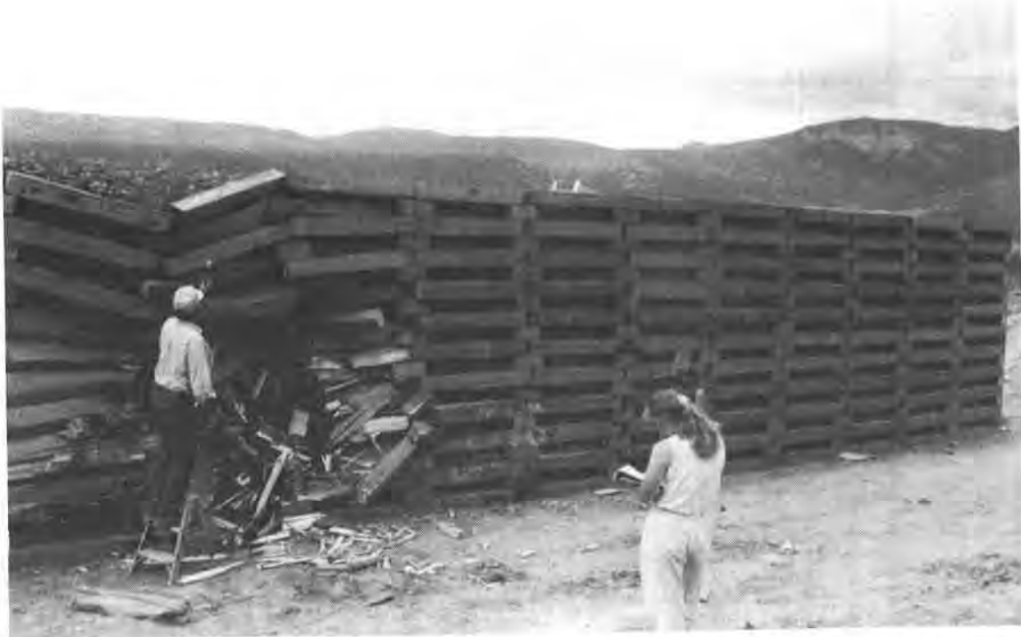
Figure 4. Test Wall After Rock Impact of Test No. 18
