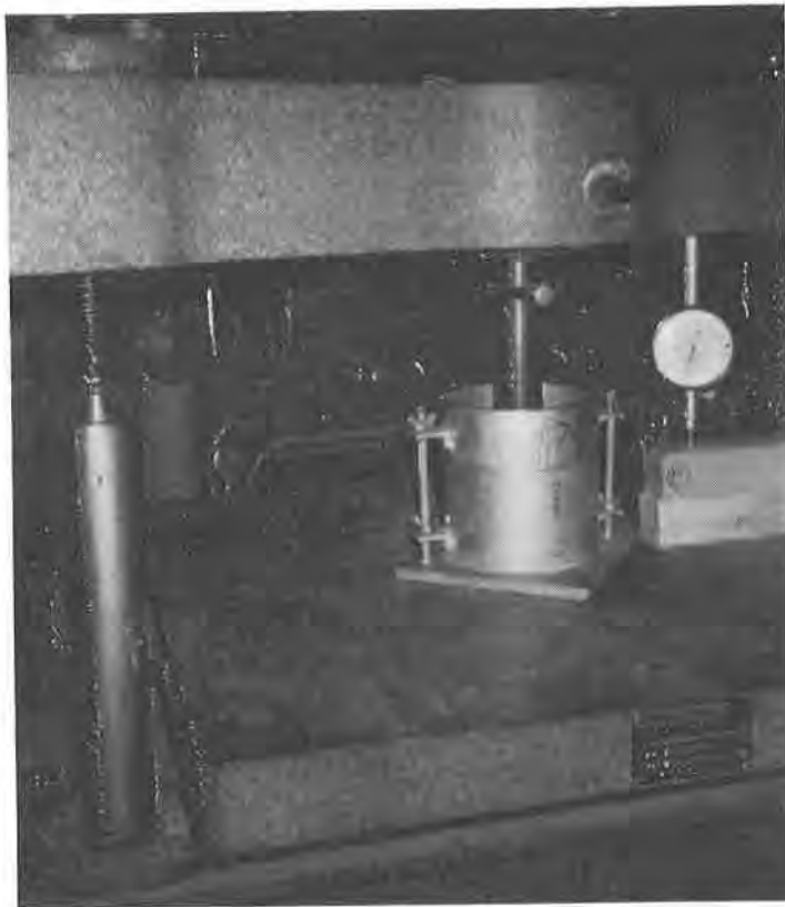
Figure 3. Specimen in Load Frame for CBR Test.
