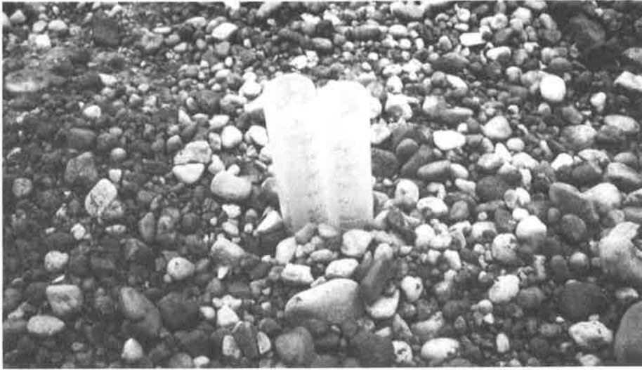
Figure 13. Graduated cylinders for water level measurement
