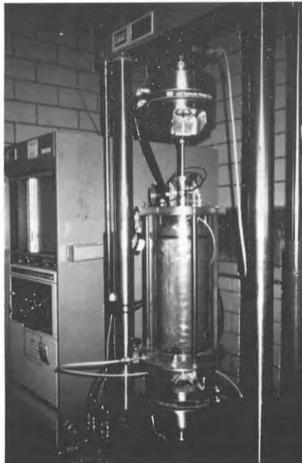
Figure 4. Triaxial Cell Mounted in MTS Load Frame for Resilient Modulus Test.
