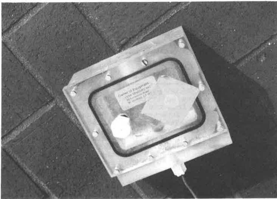
Figure 2. Calibration cell. White cap contains 1 mm hole. The "ground" electrode is inside the cell.
