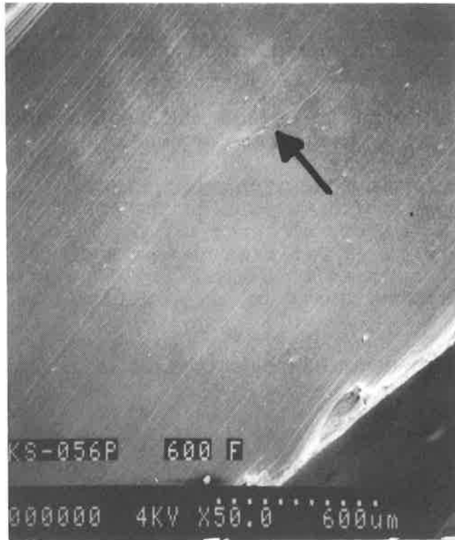
Figure 3. Thin cross section of KS-056P thermal seam made at 315°C (600°F) 50X magnification. (Arrow indicates seam area)
