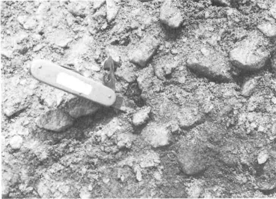
Figure 3. Stockpiled Araguaita Pit Slope Drain Material
