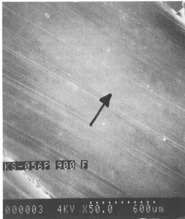
Figure 4. Thin cross section of KS-056P thermal seam made at 480°C (900°F) - 50X magnification. (Arrow indicates seam area)
