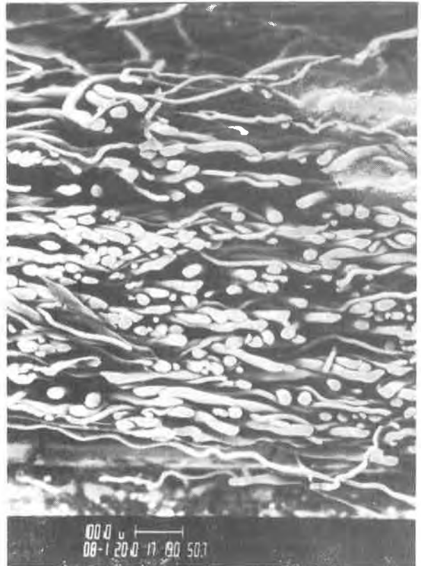
Figure 2. Micrographs of the In Plane and Perpendicular Cross Sections of the Geotextiles: a) Nonwoven, Heat Bonded Type, III Geotextile I and b) Nonwoven, Needle-Punched Type IV Geotextile M
