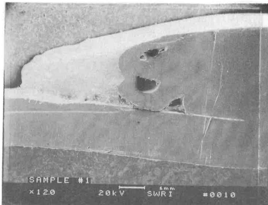
FIGURE 14. SEM IMAGE OF THIN SECTION CUT PERPENDICULAR TO 0.04-INCH DIAMETER LEAK
