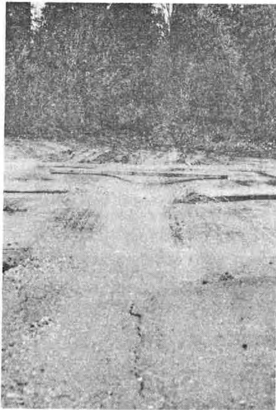
Photograph 5. Test sections after three inches of vertical deformation.
