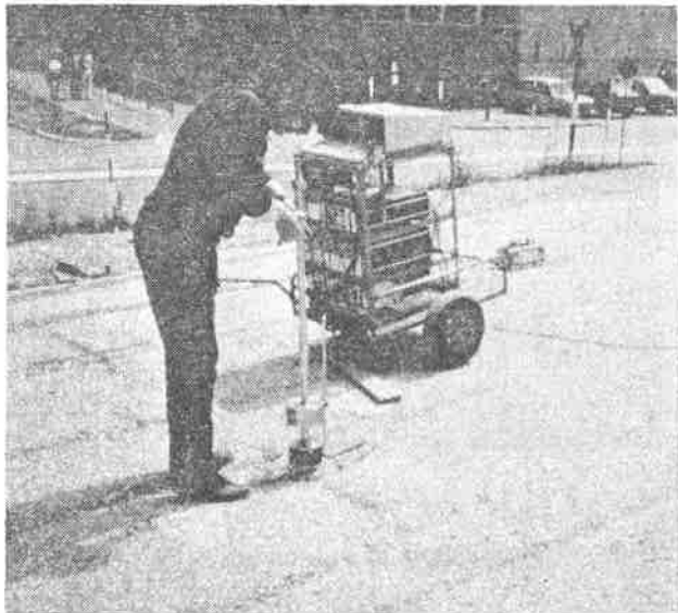
Photo 7: Dynamic plate loading tests
