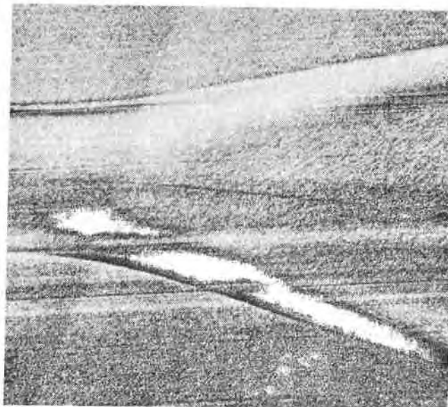
FIGURE 6. Distinct interface along the center of a fused seam weld zone. Wide bands are residual stress at edge of weld zone. (x 65)
