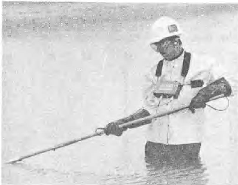
FIGURE 7. MANUAL LEAK LOCATION EQUIPMENT CONSISTING OF AN ELECTRODE PROBE AND ELECTRONICS UNIT
