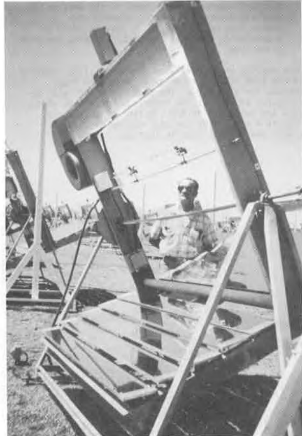
Figure 3. EMMAQUA test machine for accelerated outdoor exposure
