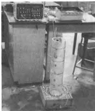
Fig. 1 - Photographs of Tube Test Setup and AE Monitoring During Test Series 3
