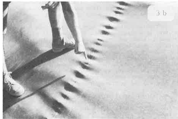
Fig. 3 Wrinkles in seams in a small dike exposed to sun and acid spray next to an ore treatment pad. The geomembrane had shrunk as a result of loss of plasticizers. However, loss of plasticizer is slower, and shrinkage is less, in seams because thickness is twofold.
