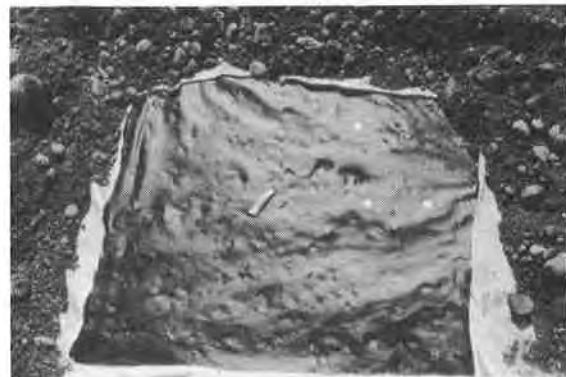
Fig. 8. CPE after test, geotextile both sides.
