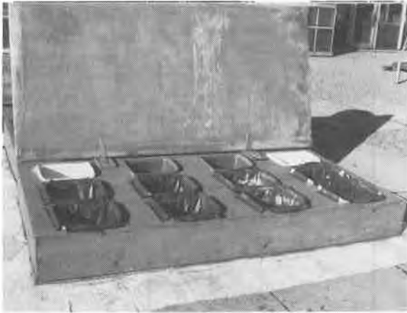
Fig. 3. - Photograph of Tub Exposure of Geomembranes to Various Chemicals
