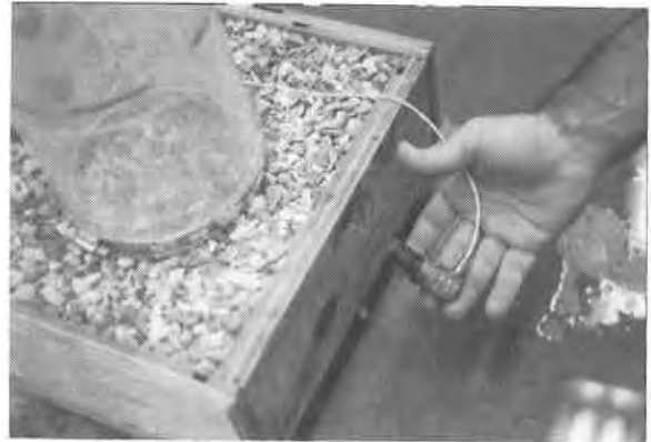
Fig. 2 - Photographs of Tank Test Setup with Wire Wave Guides and AE Monitoring Equipment
