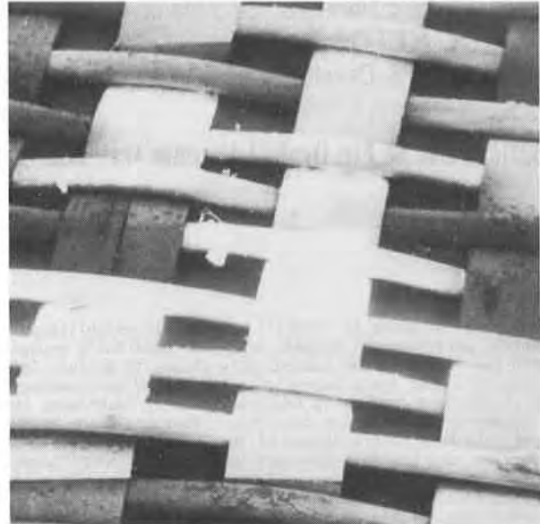
FIG. 2. Micrograph of Woven Monofilament on Tape Filter Fabric.
