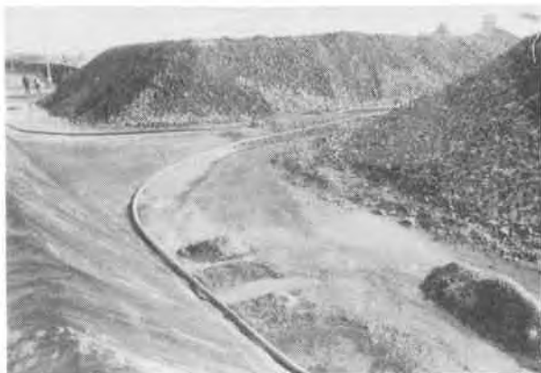
Photograph n° 7 : Sulfuric Acid leaching process Uranium Ore - (France) -
