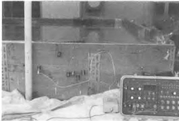
Fig. 2 - Photographs of Tank Test Setup with Wire Wave Guides and AE Monitoring Equipment
