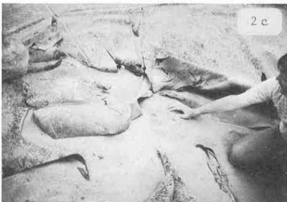
Fig. 2 Final stages of deterioration of a PVC geomembrane after it became stiff as a result of loss of plasticizers due to exposure to sun and sulfuric acid spray from an ore treatment pad. Seams appear to be the strongest areas of the geomembrane.
