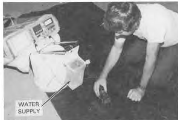
Fig. 7. Transducer holder being used with the UIP instrument to inspect chlorosulfonated polyethylene seam.
