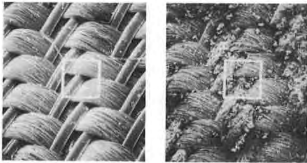
Fig. 5 GEOTEXTILE D (scale bar is 500 microns) (a) Unabraded (b) Rotary Abraded (1000 cycles)
