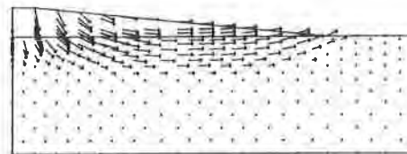
Fig. 7 Velocity Field Corresponding to the Plastic Region Shown in Fig. 6a. Impending Failure.
