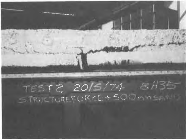
Fig. 2 Test with Structofors and Sand Bondbreaker in Progress
