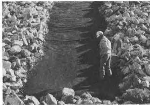
Fig. 13 Test Section Showing Condition of Filter Fabric Under Riprap Placed by Special Machine
