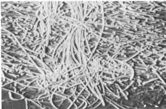
Fig. 6. Section of a needlebonded geotextile with porosity of 93%.
