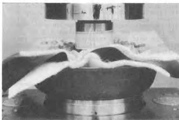
Figure 3. Apparatus to Estimate Geotextile Protection of Plastic Pond Liner Membrane During Aggregate Compression Loading.
