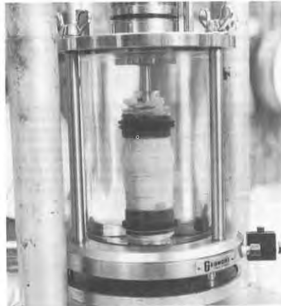
Fig. 2 Deformed shaped of internally reinforced sand tested in triaxial compression.
