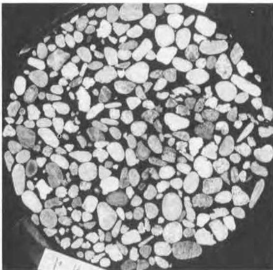
Fig. 1 Slice for pore-measurements of soils, taken from a resin bonded gravel
