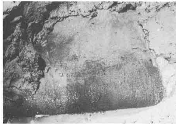
Photo 2 : Close-up of photo 1 - Top recently exposed and still pervious, bottom discoloured and impervious.
