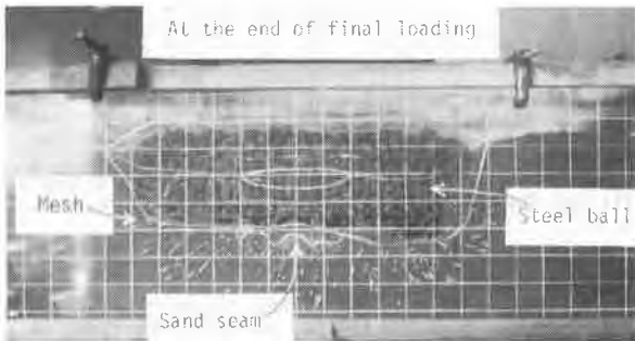
Fig. 5 Model footing test for the banking method using the resinous mesh (test series (4))
