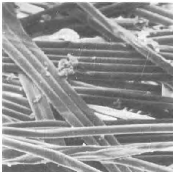
FIGURE 7 MICROSCOPIC VIEW OF HEAT BONDED GEOTEXTILE
