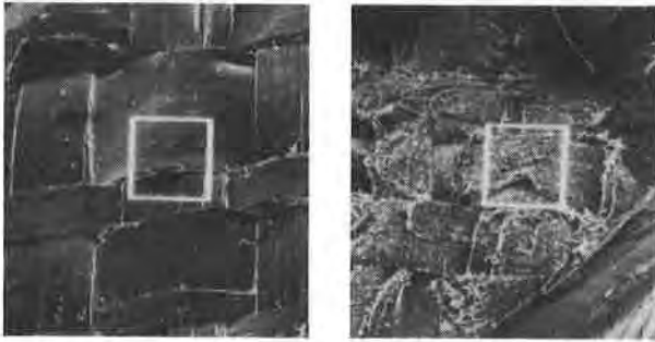
Fig. 4 GEOTEXTILE A (scale bar is 500 microns) (a) Unabraded (b) Rotary Abraded (1000 cycles)
