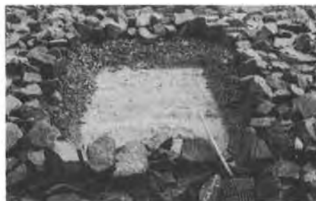
Fig. 3 Non-woven needle punched fabric after removing the cover layers
