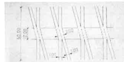
Fig.6 Special strip made according to Patent Nr 111085, used for lower bindings of the most loaded layers of dam.
