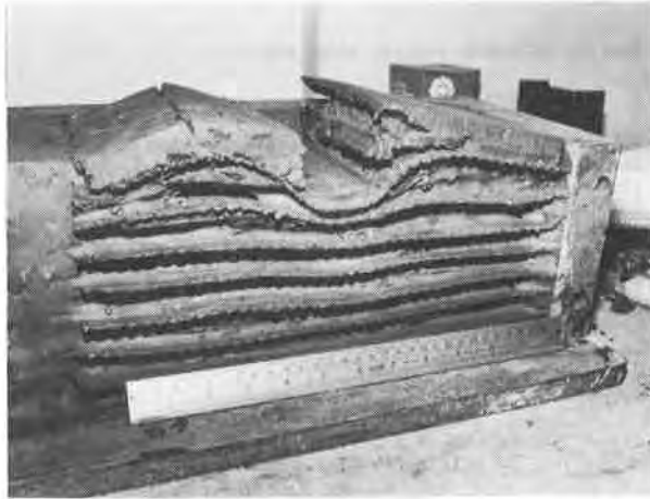
Fig. 11 Detail of Failure Mode for n = 8
