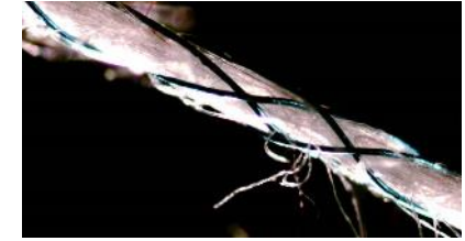
Insulated copper wires wrapped around a nylon/cotton yarn
