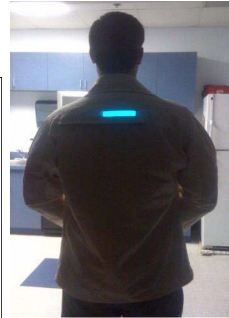
Control module and battery in pocket, Illuminated patch for demonstration of seaming technology only
