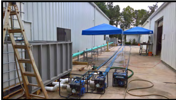
Figure 3. Sump Discharge is Pumped Back to Headbox
