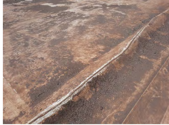
Figures 12 & 13. Surface cracks found in the RPP liner material folds and creases
