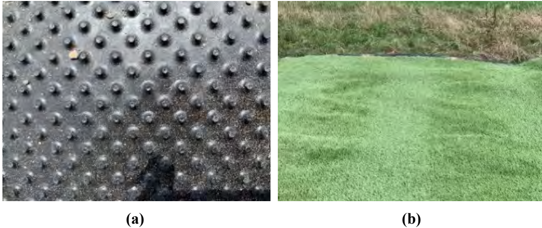
Figure 2. (a) Textured geomembrane layer (b) engineered turf.
