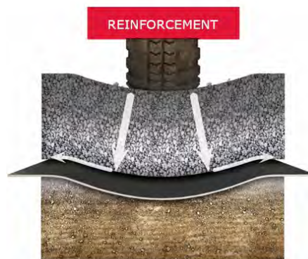
Figure 2. Mechanism of reinforcement – membrane effect.
