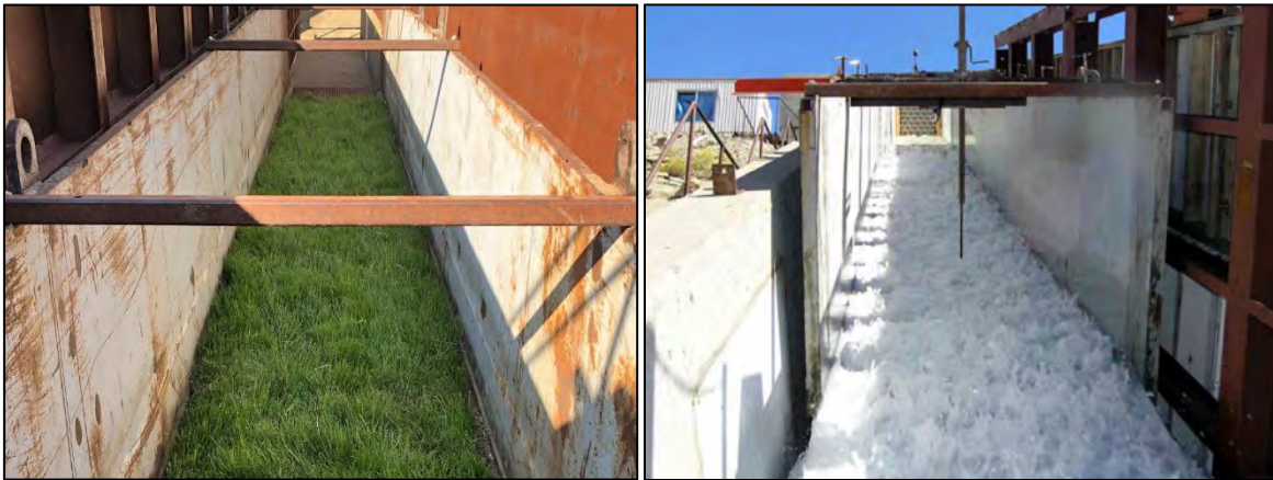
Figure 3. Full Scale Testing per ASTM D-6460 – Vegetated HPTRM (Left) and during Flume Test (Right)
