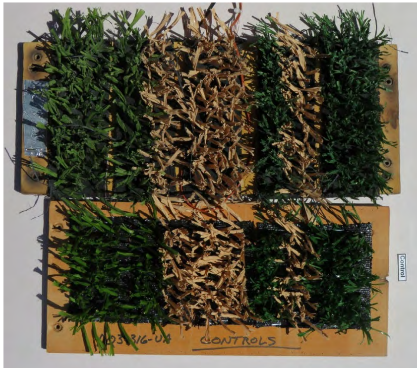
Figure 4. Laboratory weathered (top) at 21 years of equivalent exposure and control (bottom) engineered turf samples
