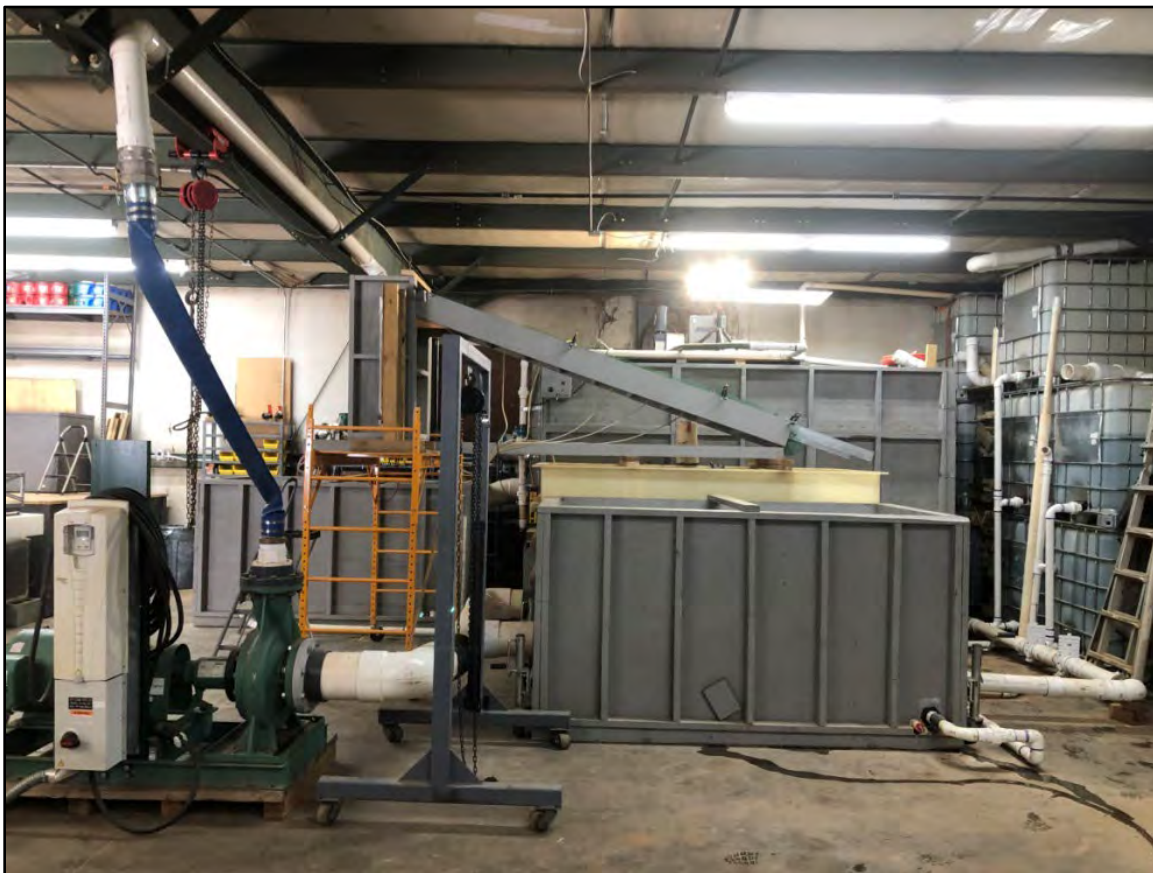
Figure 21. Steep Slope Test Apparatus Setup
