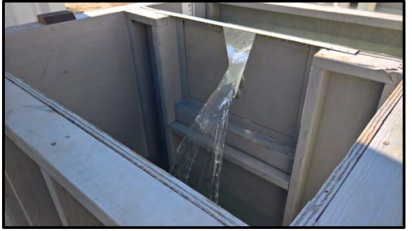
Figure 6. 33° V-Notch Weir used for Lower Flow Testing
