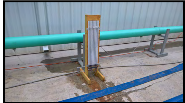
Figure 4. Monometer Board for Reading Piezometric Heads
