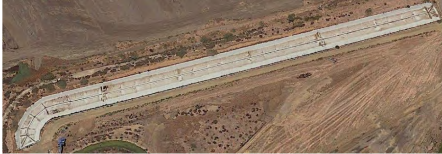
Figure 3. CSPE Floating cover on a channel at a Wastewater Treatment Plant capturing biogas and to eliminate odors. South Australia. (Image: Google Earth 2018)
