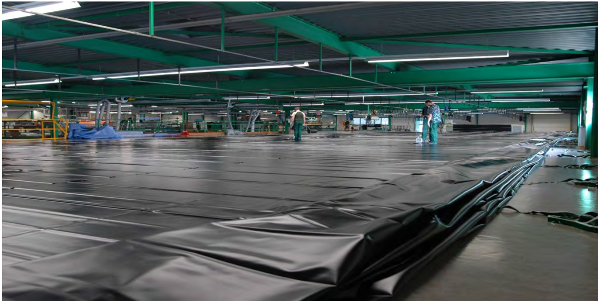
Figure 1. Prefabrication PVC geomembrane panels in production area
