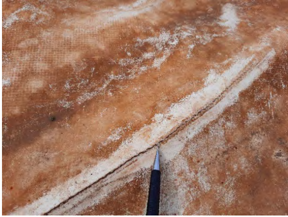
Figures 12 & 13. Surface cracks found in the RPP liner material folds and creases
