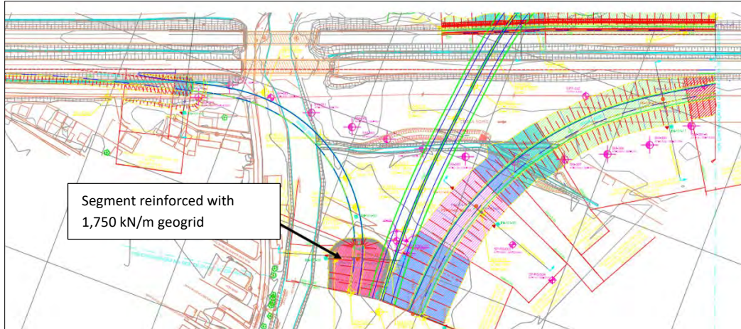
Figure 6 – Segments of the project with geogrids of varying tensile strengths
