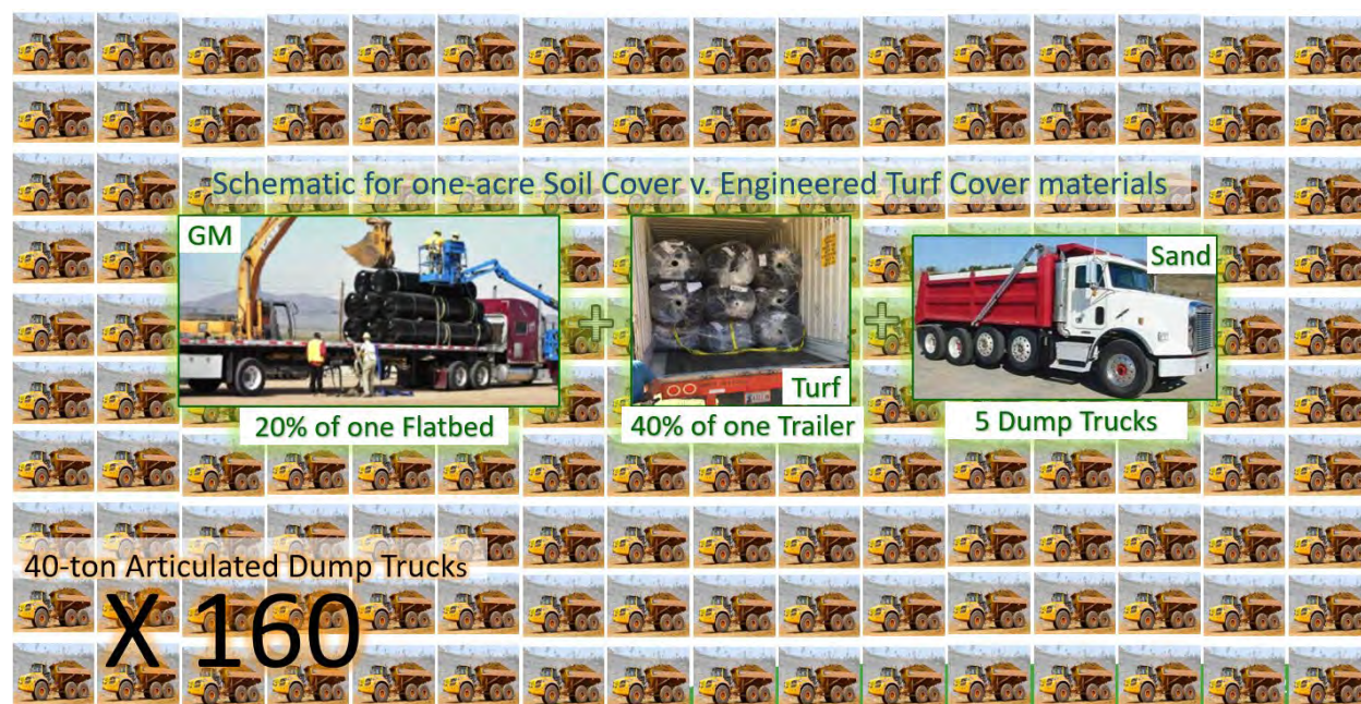
Figure 5. Schematic for transportation of construction materials: Soil cover v. ETC.
