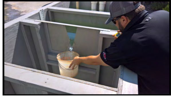
Figure 8. Example of Timed Catch to Verify Flow Rate
