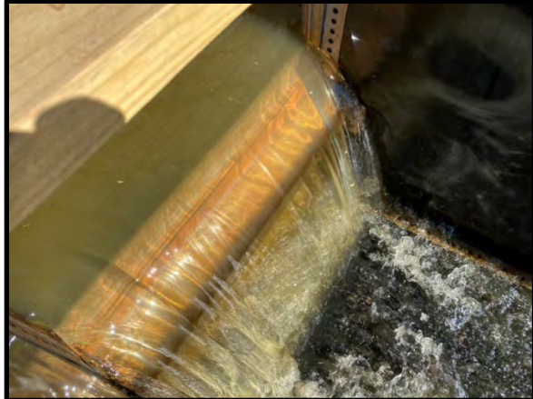
Figure 15. Uniform Flow Introduced Over the Sharp Crested Weir
