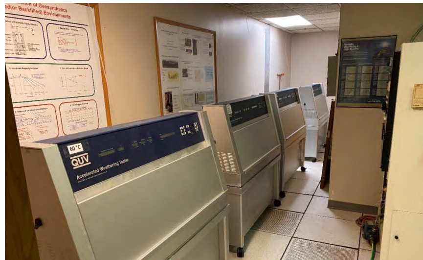
Figure 9. Photograph of the weathering durability lab at the Geosynthetic Institute (GSI). Note, four UV accelerated weathering apparatuses on the left and a single Xenon apparatus on the right
