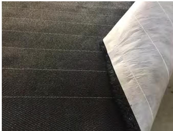
Figure 9. Geotextile tube with nonwoven filter inner liner.
