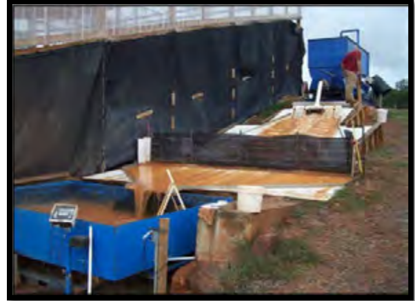
Figure 2. ASTM D 7351 Test Setup
