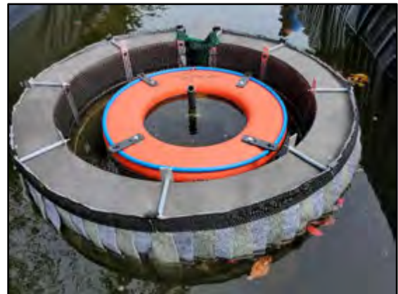
Figure 18. Skimmer Testing in Test Tank
