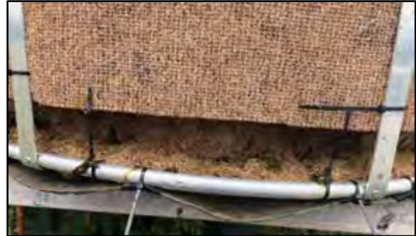
Figure 22. Blocksom Inlet Filter Material After Testing
