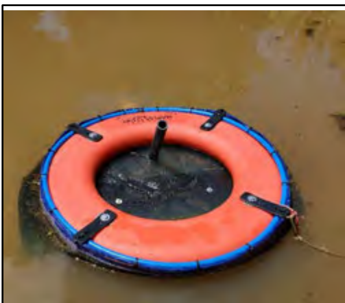
Figure 8. Skimmer with Siltron with Open Bottom
