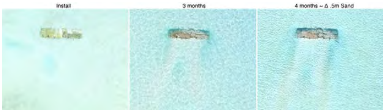
Fig 10. Aerial photos of the bladder over 4 months showing accumulated sediment change.
