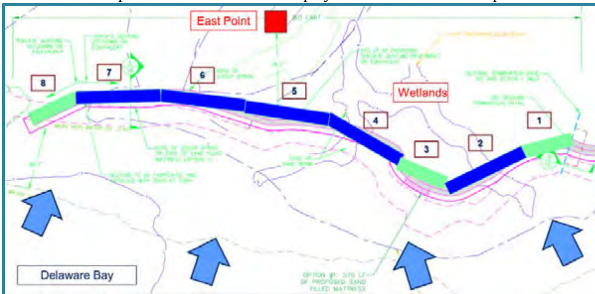
Figure 4: The eight sections on a plan view and the relative position of the Lighthouse and the wetlands to the structure.
