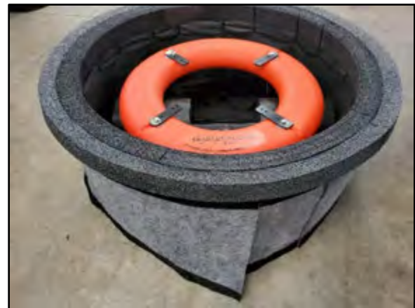
Figure 12. Skimmer Basket with Outer Layer X-Tex & Inner Layer Mirafi
