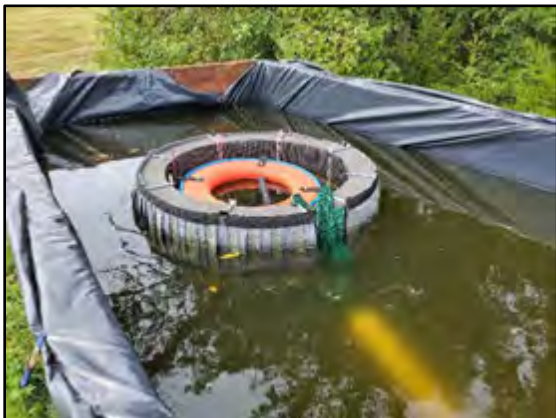
Figure 17. Skimmer Testing in Test Tank
