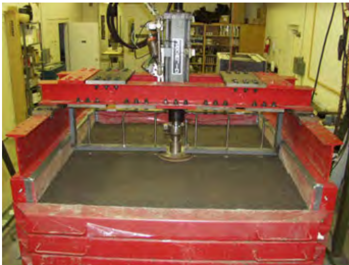
Figure 4. Completed test set up prior to load testing from Tingle and Jersey (2005). Construction of Model Pavement Sections
