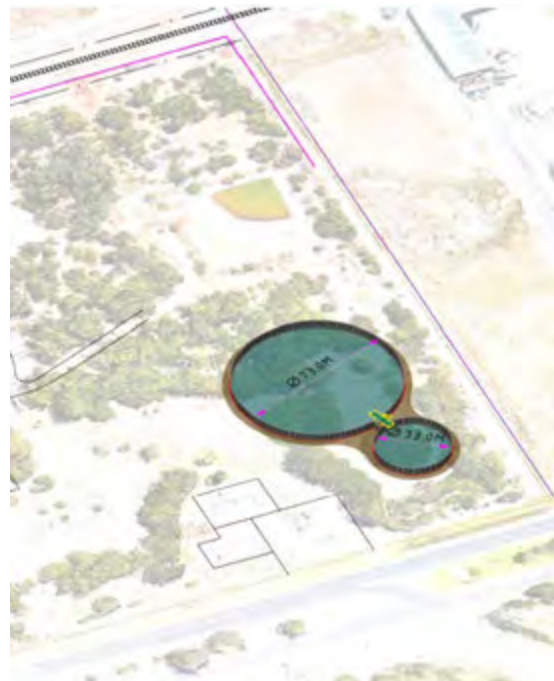
Figure 2. Two Modular Storage Tanks.
