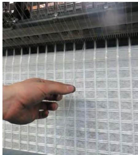
Figure 11. Insertion of the optical fibers in the product
