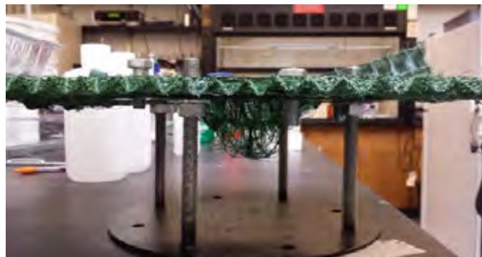
Figure 4. HPTRM A specimen after static puncture test.
