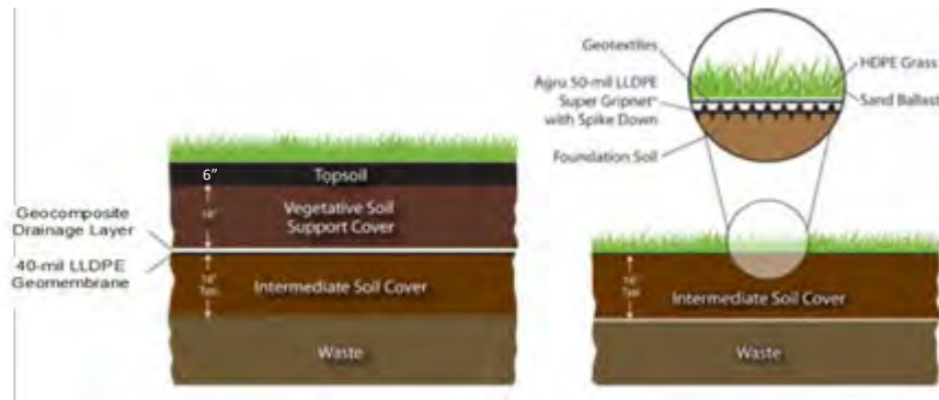
Figure 3. Comparison of a traditional soil cover with the engineered turf cover.
