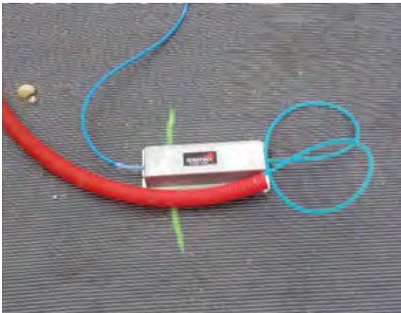
Figure 13. Hydraulic settlement gauge
