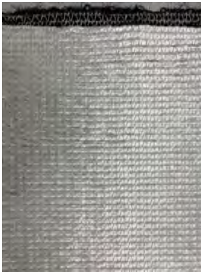
Figure 3. Detail of a high strength, high modulus, PVA reinforcement used on LTPs. (source: HUESKER Inc.)
