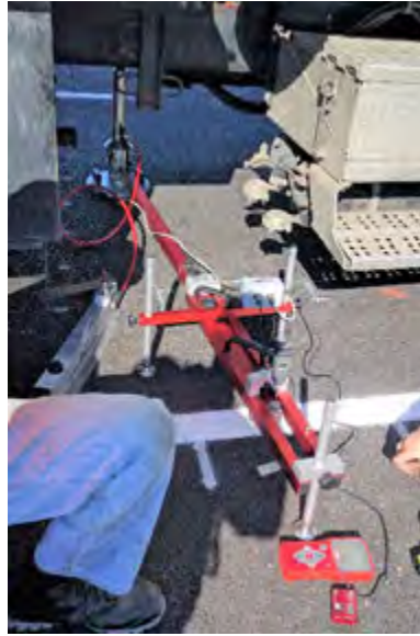
Figure 3. Static Plate Load setup used in the study.
