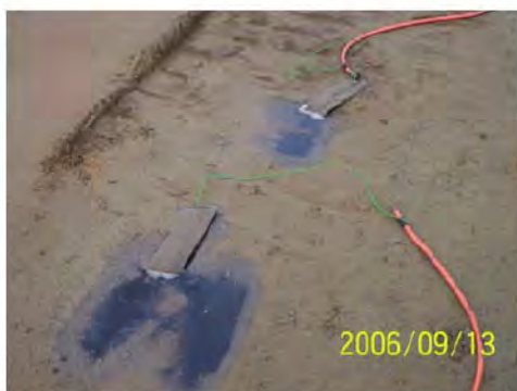
Figure 8: Discharge of groundwater from Cathode
