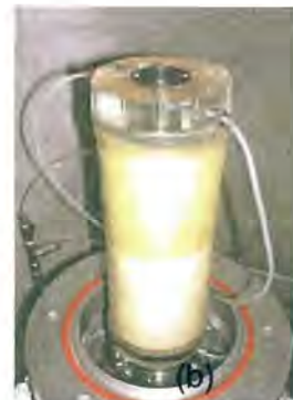
Figure 5 The bender-extender system used in the laboratory program (a) the pedestal of the device with the insert element, (b) EPS specimen mounted in the testing system
