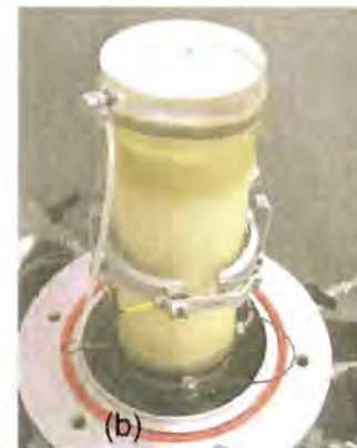
Figure 3 (a) The triaxial (cyclic/monotonic) loading system used in the laboratory program, (b) the local strain measuring transducers used in the triaxial tests on EPS specimens
