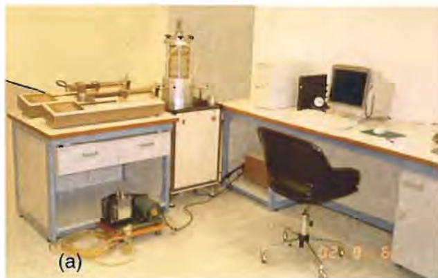
Figure 3 (a) The triaxial (cyclic/monotonic) loading system used in the laboratory program, (b) the local strain measuring transducers used in the triaxial tests on EPS specimens
