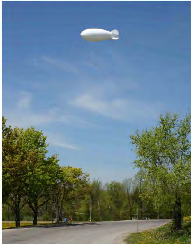
Figure 1 Photograph showing blimp equipped with a digital camera used to obtain images of geomembrane wrinkles.
