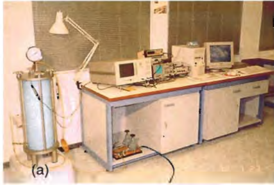
Figure 4 (a) The resonant column system used in the laboratory program, (b) cylindrical EPS specimen mounted to the pedestal of the resonant column device
