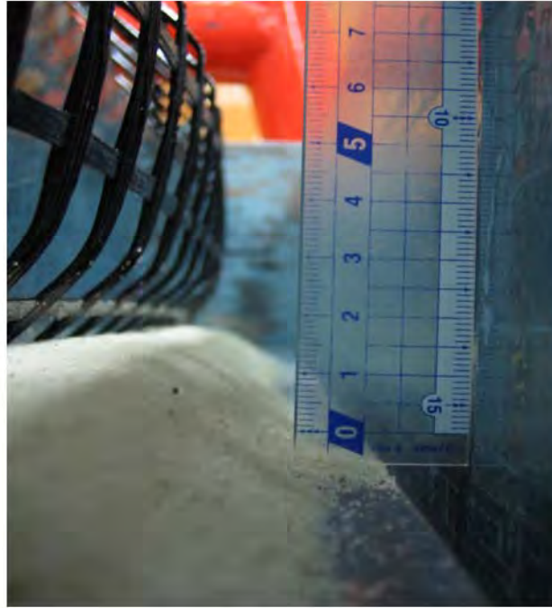
Figure 5. Soil particles are extruded out of shear box and heave up at the front edge of lower, larger shear box.
