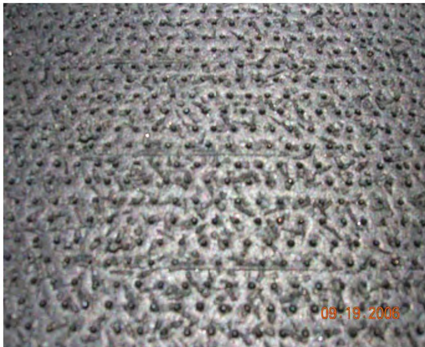
Figure 2. Flat Die Molded Textured Surface (Surface Friction Profile)
