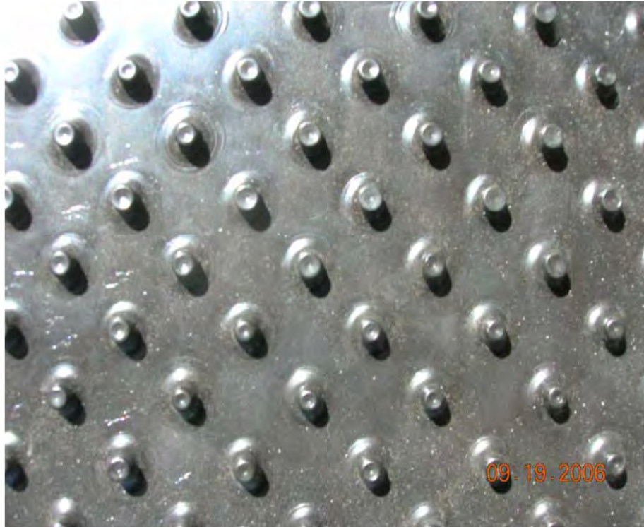
Figure 3. Flat Die Molded Structured Surface (Drain Surface Profile)
