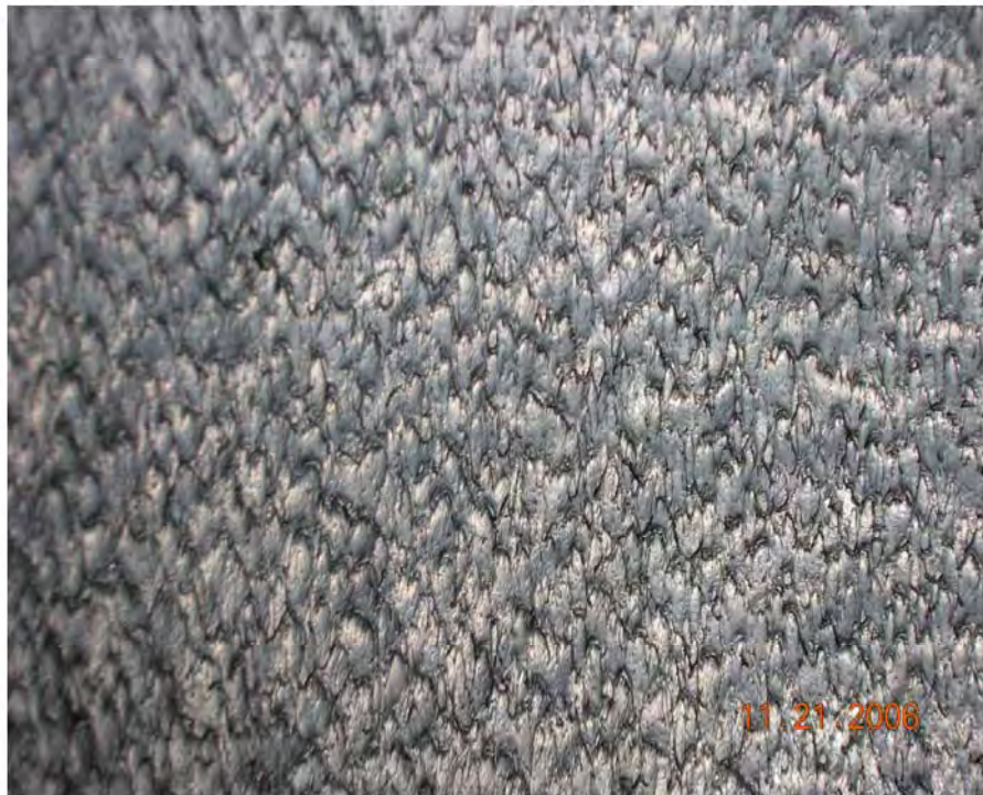
Figure 5. Co-extruded Surface Texture Medium (Blown Film Process)
