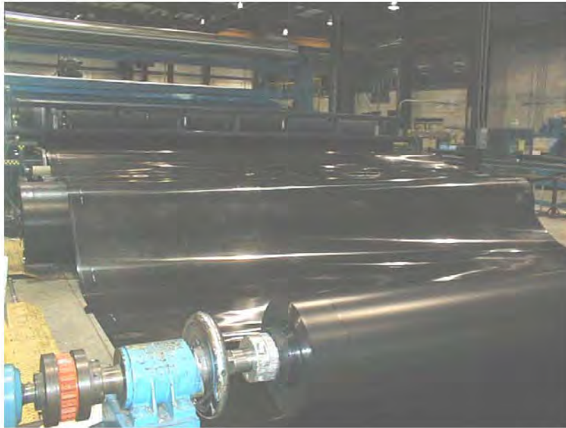
Figure 1. Flat Die Calendaring Manufacture (Smooth Sheet Production)
