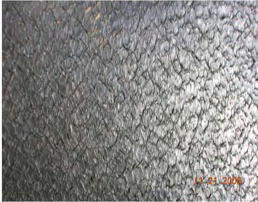
Figure 4. Co-extruded Surface Texture Light(Blown Film Process)
