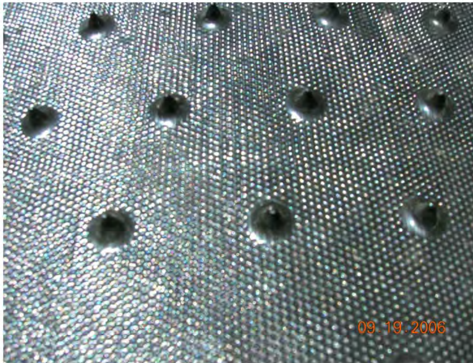
Figure 6. Bottom Emposed Structure or Spike Surface
